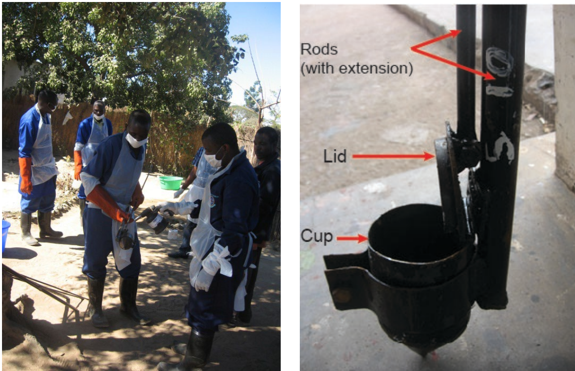
FIGURE 2-2: FIELD SAMPLING (LEFT) USING SPECIALLY DESIGNED PIT LATRINE SAMPLERS (RIGHT)
