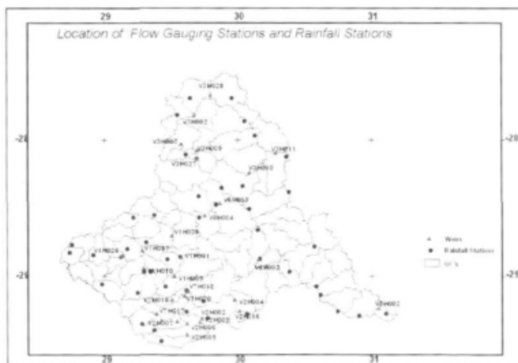
Figure 4.5 Raingauges and flow gauging weirs in the Thukela Catchment
