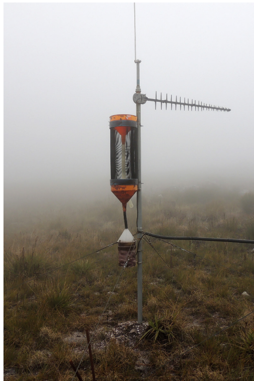
Left: The fog collector used at Dwarsberg weather station, Jonkershoek is based on a design used by other fog researchers in North and Central America.
