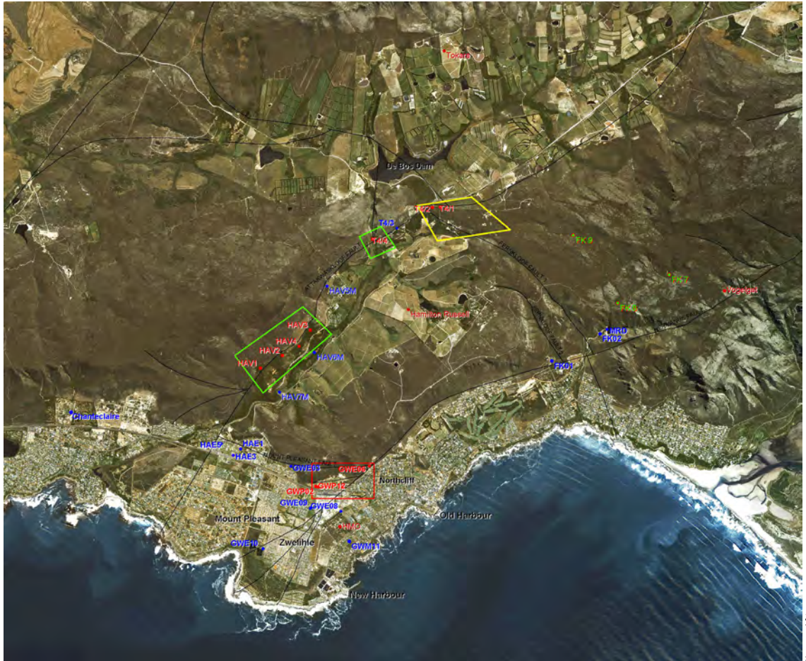
The three Hermanus wellfields and associated monitoring sites. The red block represents the Gateway wellfield, the green Campbell and the yellow Volmoed wellfield.
