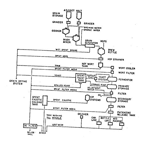
Figure 3.1 : Schematic of Brewing Process
