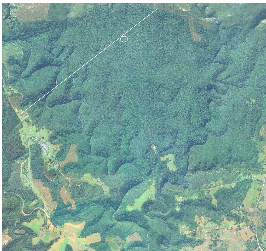
Figure 18. Aerial photograph of the Groenkop indigenous forest, showing the Saasveld campus in the southwest quadrant. The superimposed line shows the path of the LAS beam (3.1 km), while the circle shows the position of the Eddy Covariance system.
