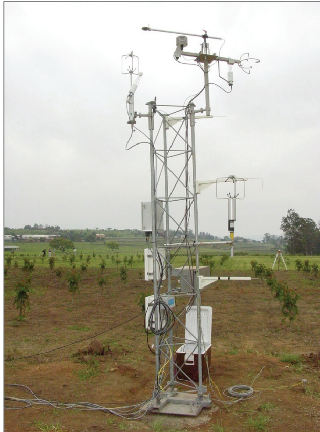
Plate 7.11 The micrometeorological mast with eddy covariance and surface renewal instrumentation
