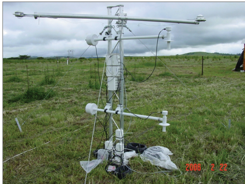
Plate 7.13 The OEBMS1 mast with pyrriadiometer, pyranometer, soil heat flux sensors and two ventilated thermometers (PT100) at the Ukulinga site
