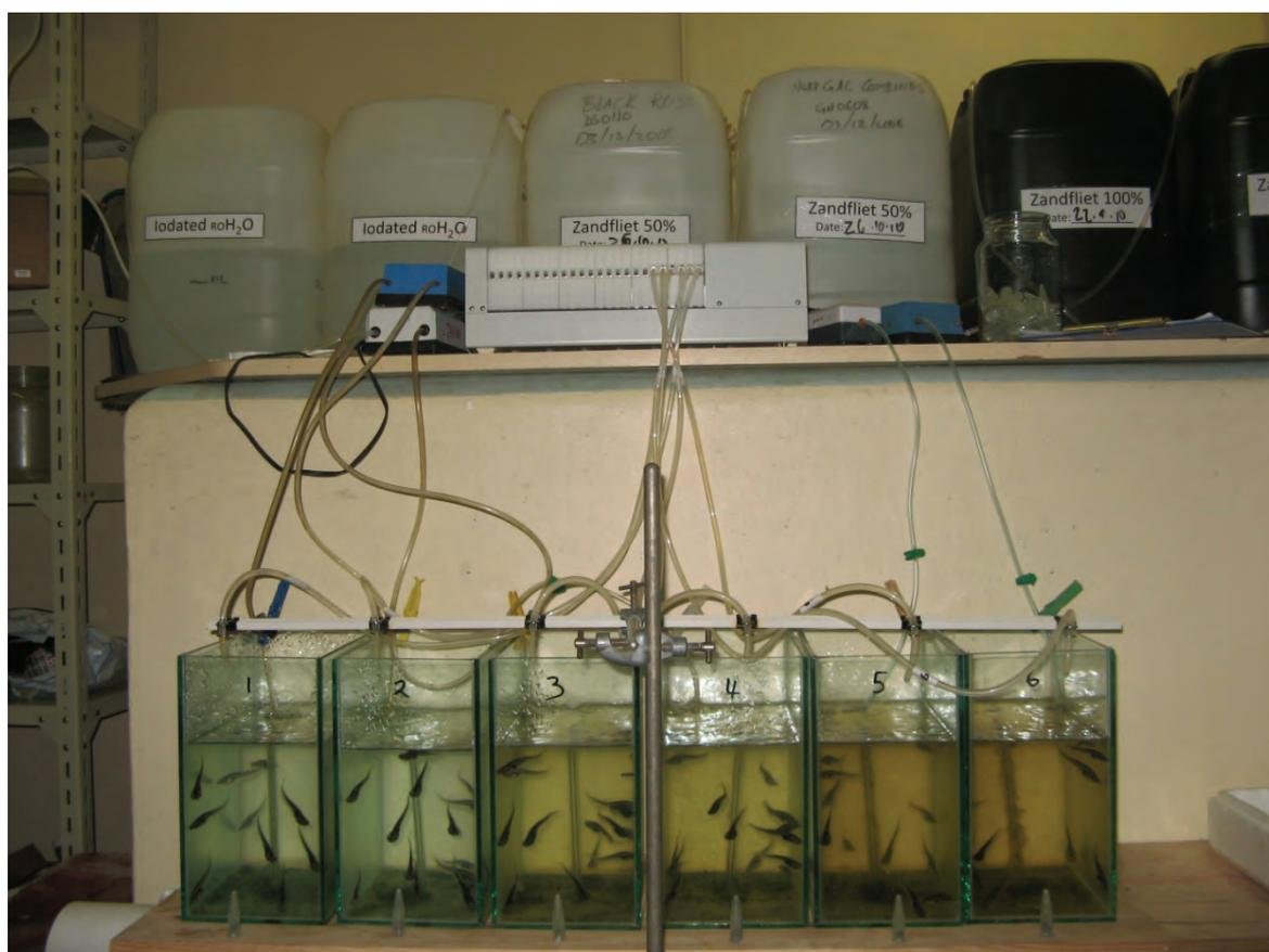
**Figure 13. Simple flow-through set-up. An 18 channel peristaltic pump was used to control the flow rate. Replicate exposures were included for a Water Control (Buffered RO water), 50% diluted effluent and 100% (undiluted) effluent.**
