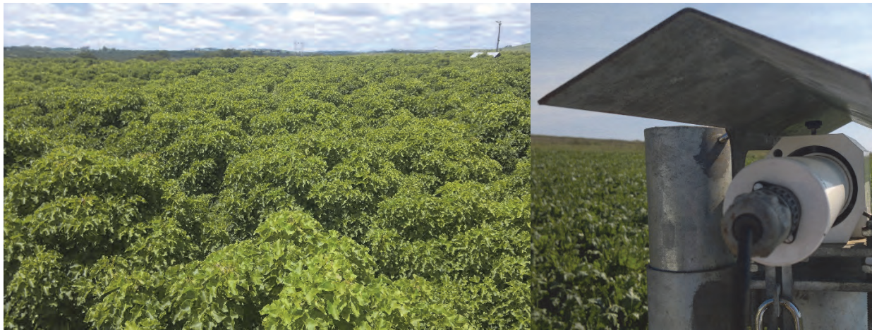
Figure 29 (a) View from the steel pole which supported the SLS receiver used to measure total evaporation diagonally across two adjacent Jatropha only (i.e. weed-free) plots at Ukulinga in January 2011 (b)
