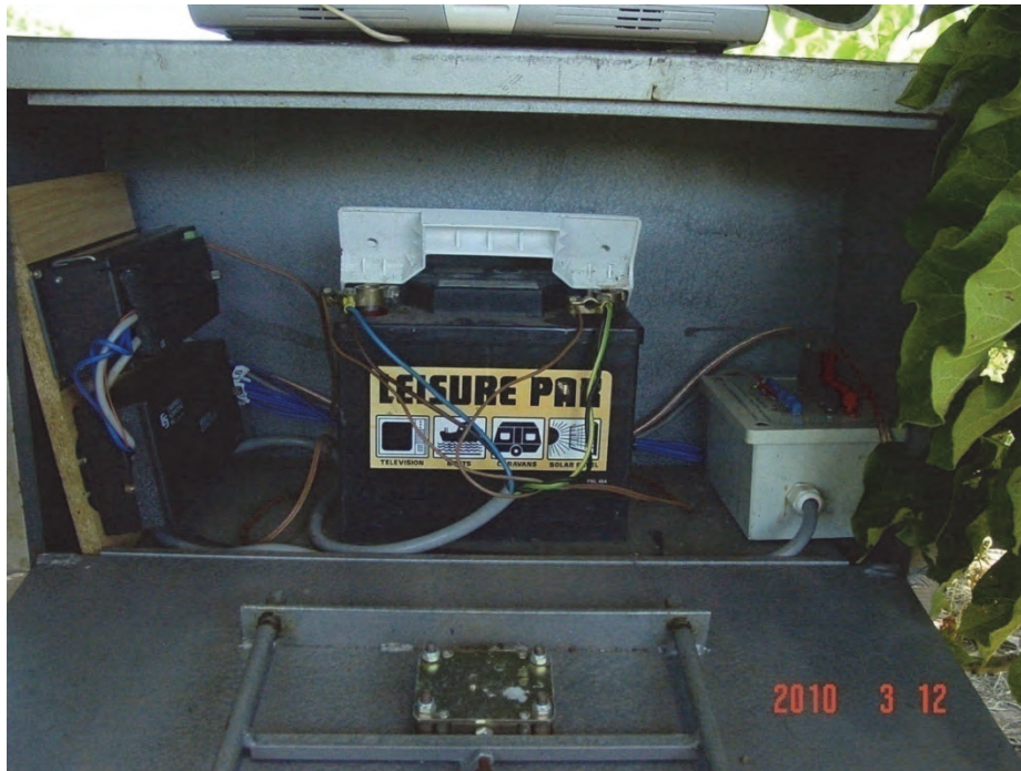
Figure 26 Hardware utilised for the monitoring of transpiration (sap flow)
