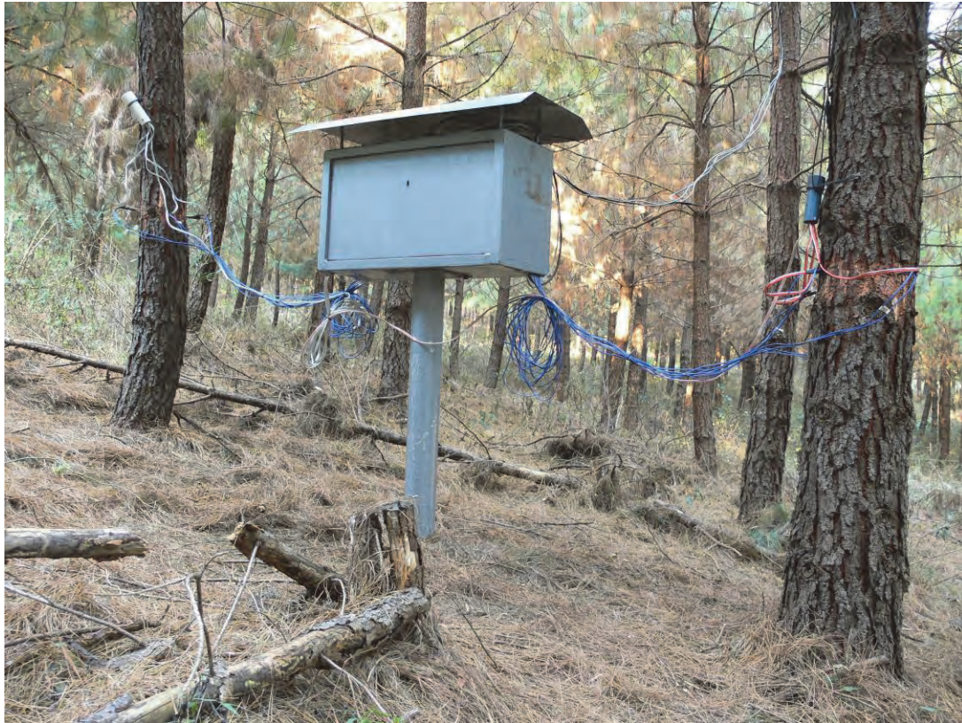
Figure 3. Heat Pulse Velocity system measuring sap flow in Pinus patula trees (Photo: M. Gush).
