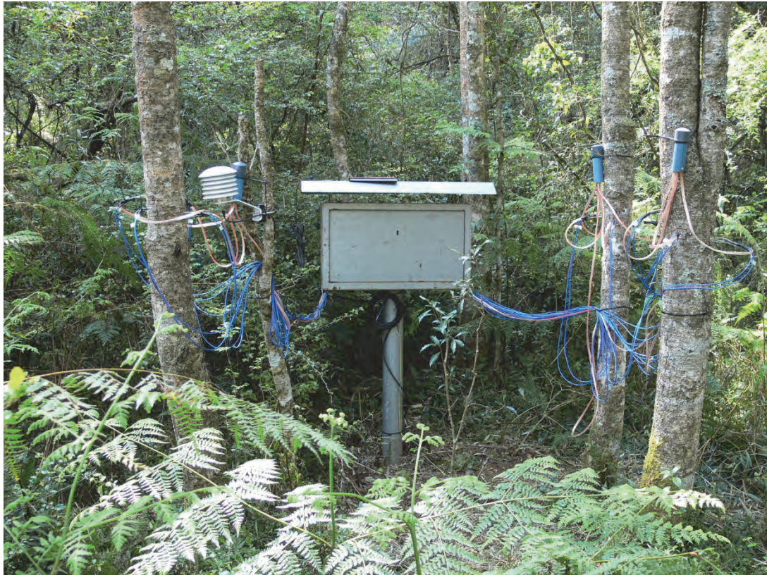
Figure 35. Heat Pulse Velocity system measuring sap flow in Rapanea melanophloeos (Cape Beech) trees at Ingeli (Photo: M. Gush).
