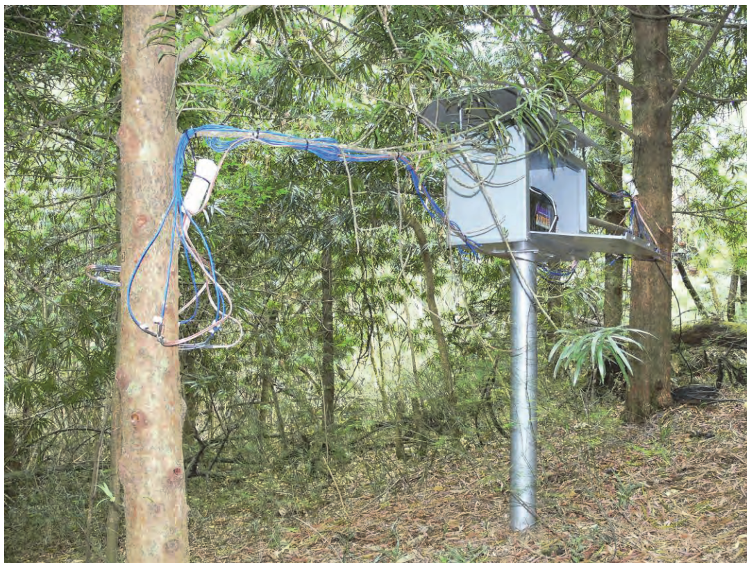
Figure 2. Heat Pulse Velocity system measuring sap flow in indigenous Podocarpus henkelii (Yellow-wood) trees (Photo: M. Gush).
