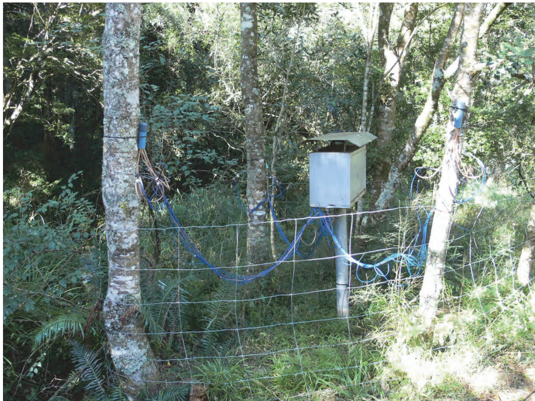
Figure 34. Heat Pulse Velocity system measuring sap flow in indigenous Celtis africana (White Stink-wood) and Prunus africana (Red Stink-wood) trees at Ingeli (Photo: M. Gush).
