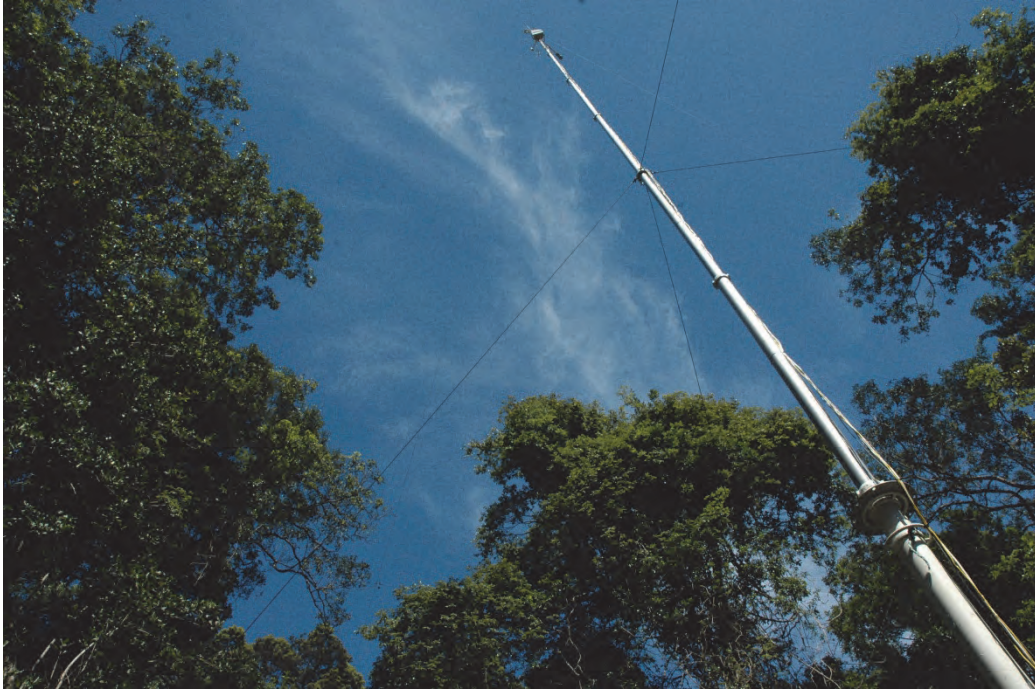
Figure 37. Telescopic mast and eddy covariance system projecting above the Ingeli forest canopy, and measuring ET_{EC} (Photo: M. Gush).
