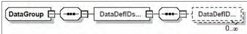
Figure 4.20 The DataGroup element in the revised ModelConfiguration schema
