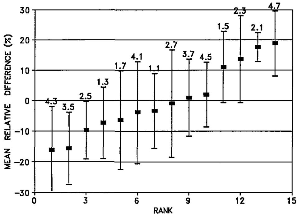
Figure 4.7 Ranked intertemporal relative deviation from the mean topsoil (0-0,45 m) water content based on all 15 measurements made during summer and winter. The vertical bars indicate the associated time standard deviation, while the numbers are the identification code for the 14 sampling sites.
