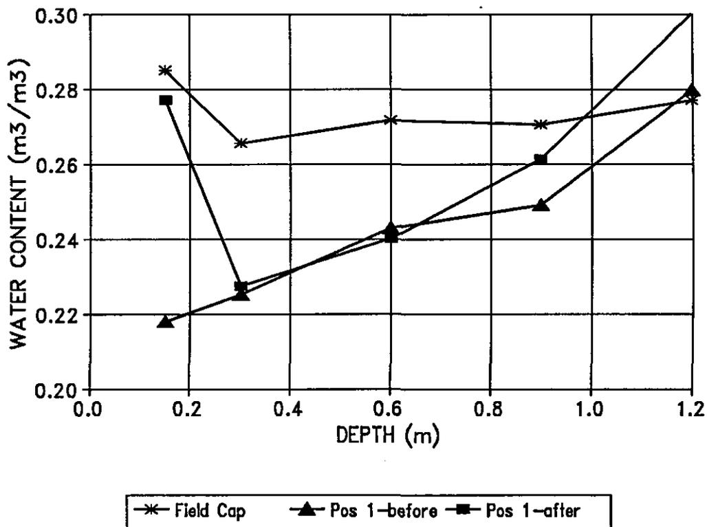
Figure 6.4 Depth distribution of soil water content at field capacity, before and after an irrigation event on 30/12/89. (FC = mean value for field capacity at site A2 and A4; spatial mean = of total area per emitter; Pos 1 = monitoring position below an emitter)
