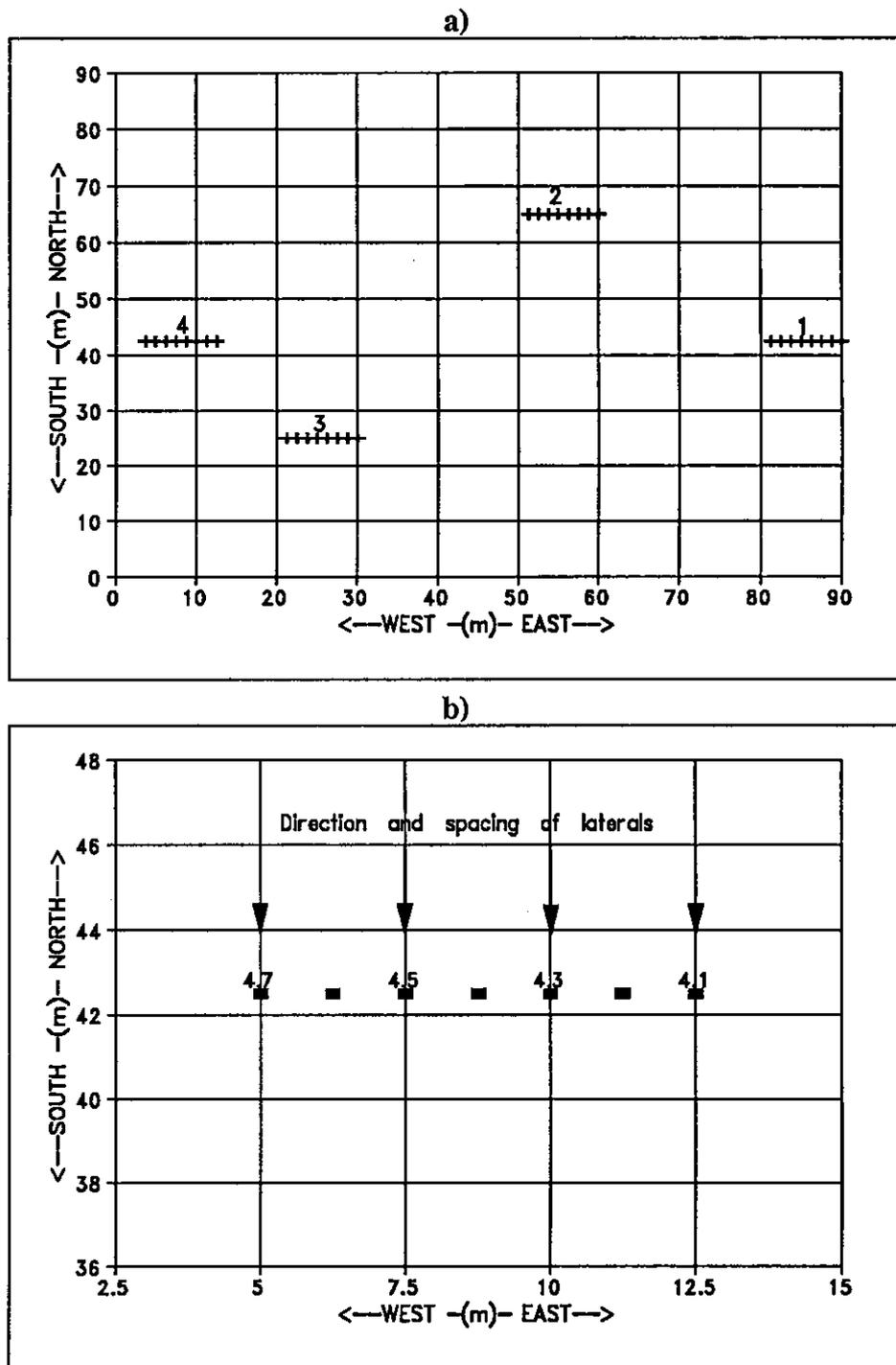
Figure 4.1 Location of: a) the 15 neutron access tubes distributed as four groups within the drip irrigated field, and b) spacing, location and identification within group 4.
