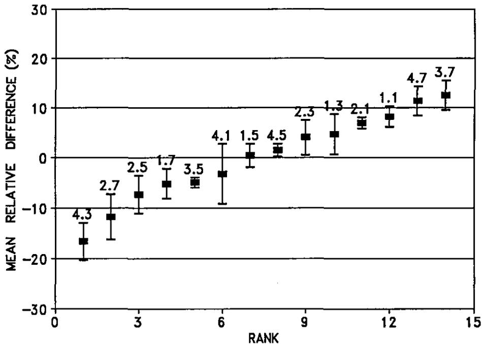
Figure 4.6 Ranked intertemporal relative deviation from the mean profile (0-1,05 m) soil water content based on 5 different measuring dates during winter. The vertical bars indicate the associated time standard deviation, while the numbers are the identification code for the 14 sampling sites.
