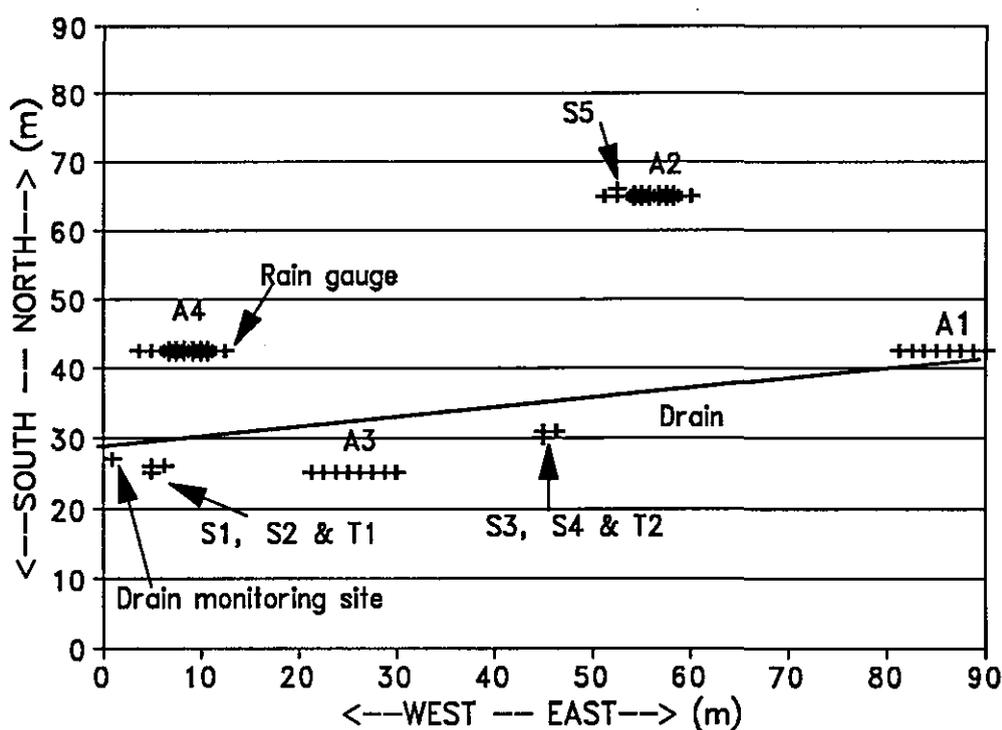
Figure 6.1 Map of the drip irrigated vineyard indicating the location of the drain pipe and various monitoring positions. (A=neutron access tubes and soil sampling sites, T=tensiometer site, S=porous cup sampler)
