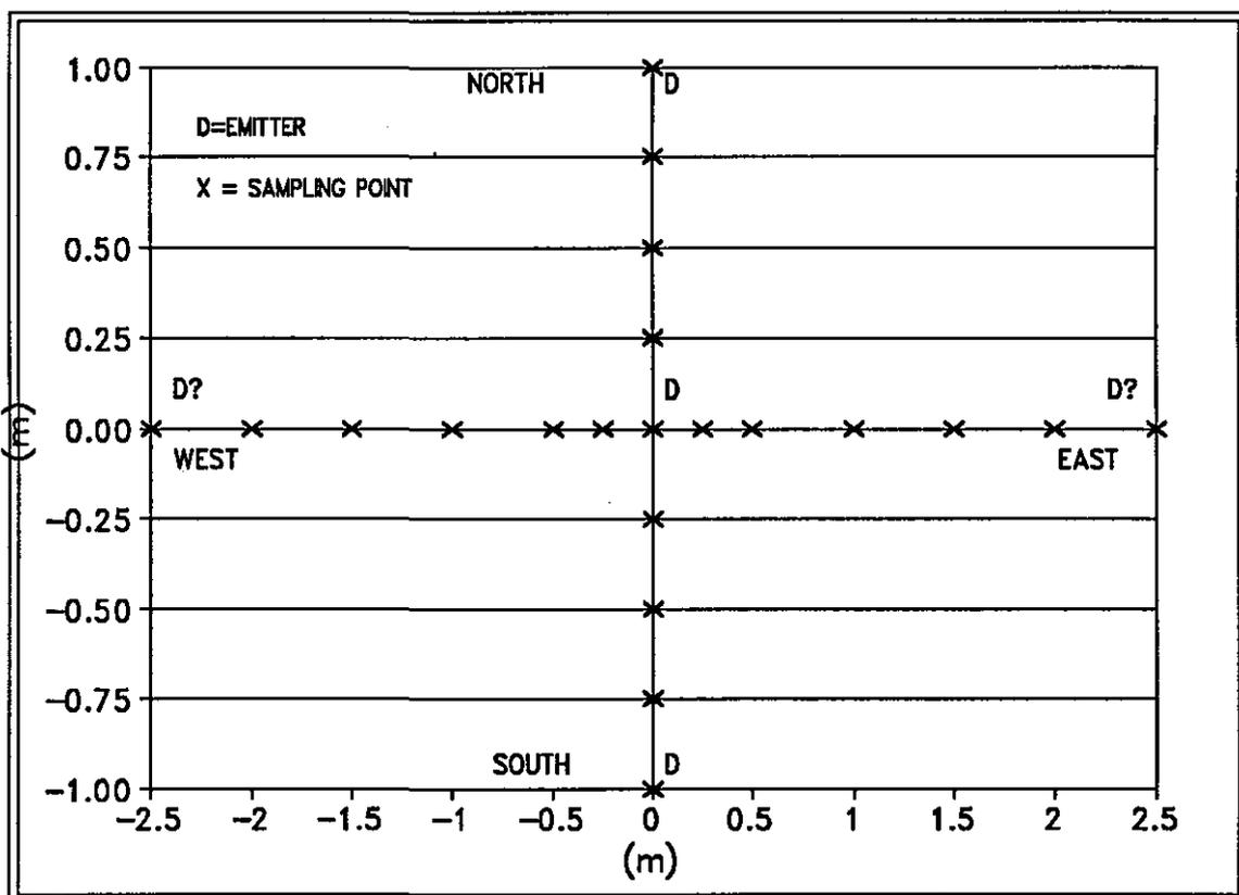
Figure 3.1 Diagram of the scheme involving 21 sampling points surrounding an emitter. This sampling scheme was replicated at four randomly chosen locations within the study area.
