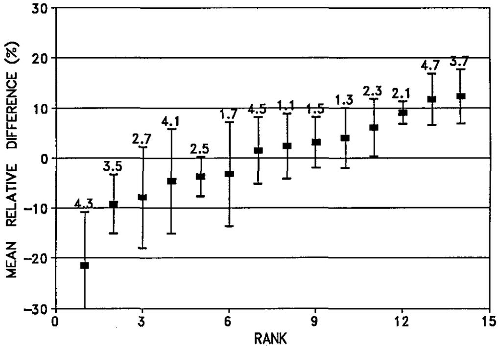
Figure 4.5 Ranked intertemporal relative deviation from the mean profile (0-1,05 m) soil water content based on 10 different measuring dates during summer. The vertical bars indicate the associated time standard deviation, while the numbers refer to the 14 sampling sites.
