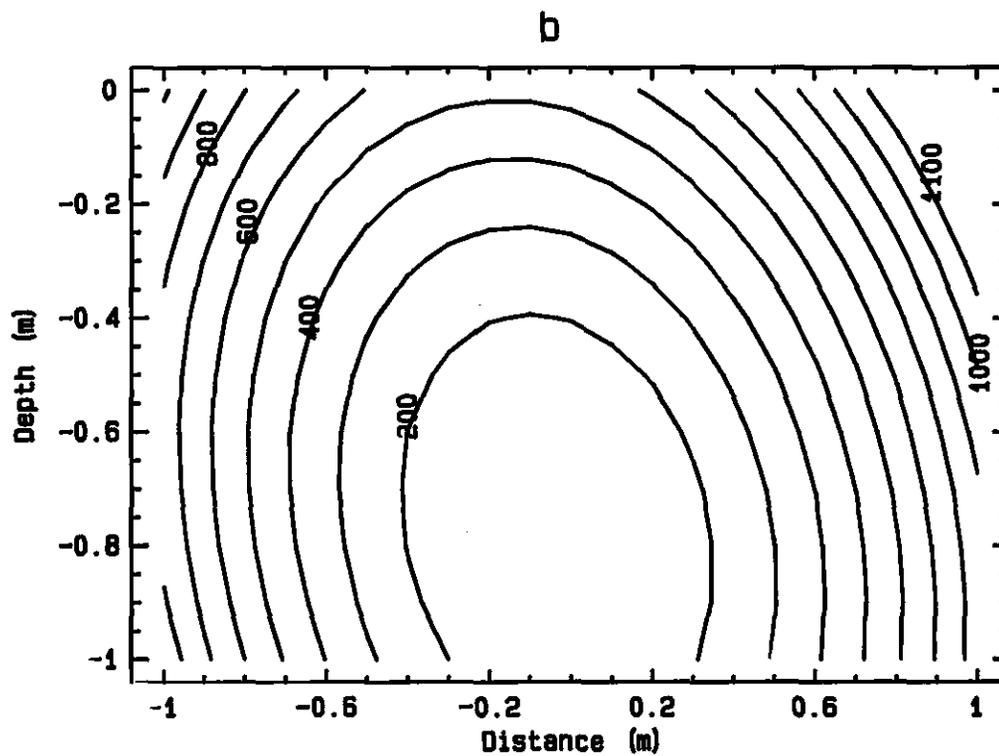
Figure 3.6 Iso-conductivity lines ( $\text{mS m}^{-1}$ ) around an emitter: a) north-south transect, b) east-west transect. Negative distances indicate points to the south and west of the centre emitter.
