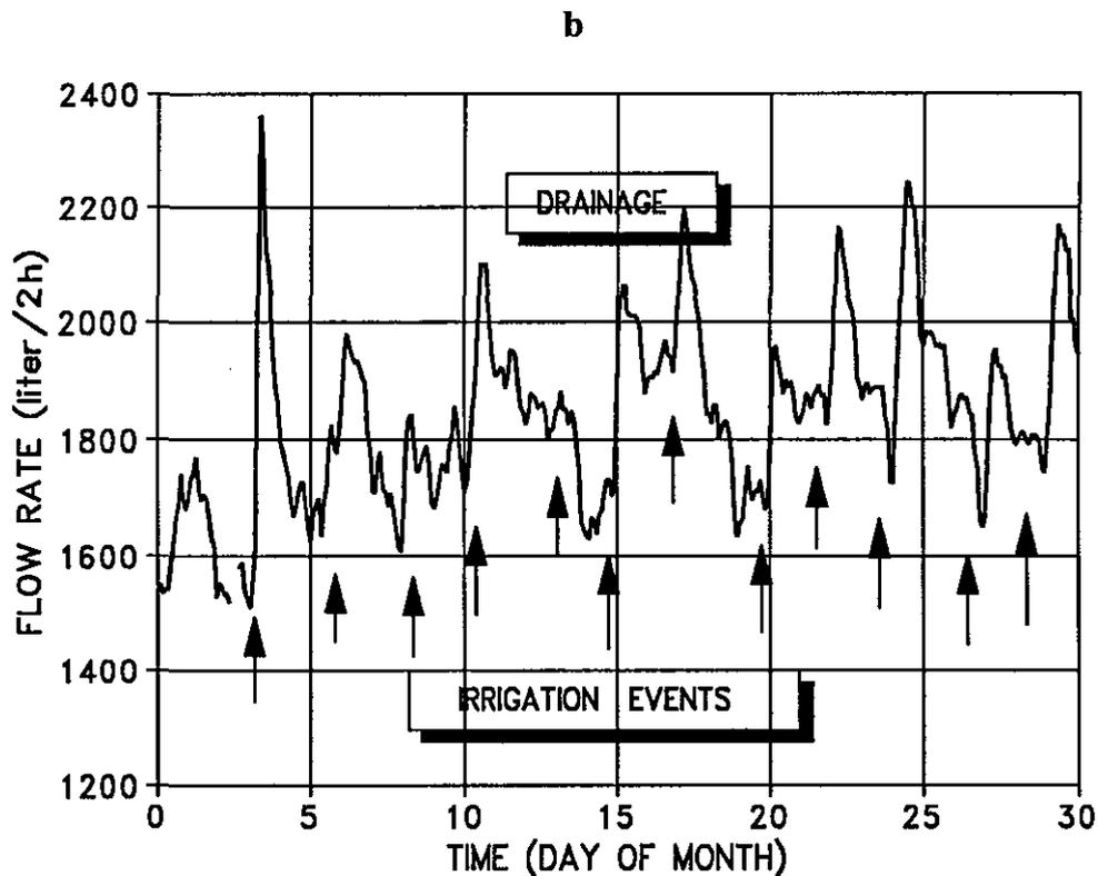
Figure 6.3 Flow rate in the tile drain for the period a) October to December 1988, and b) November 1988. The start of each irrigation event is indicated by the arrow
