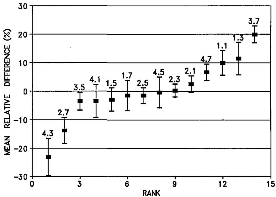
Figure 4.8 Ranked intertemporal relative deviation from the mean subsoil (0,45-1,05 m) water content based on all 15 measurements made during summer and winter. The vertical bars indicate the associated time standard deviation, while the numbers are the identification code for the 14 sampling sites.
