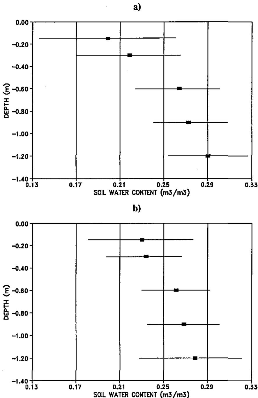
Figure 4.2. Mean and standard error of the volumetric soil water content at 14 monitoring sites in a drip irrigated vineyard near Robertson: a) Summer measurements (n=10), and b) Winter measurements (n=5).
