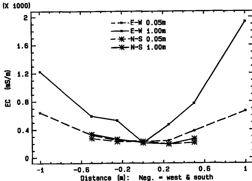
Figure 3.5 Distribution of salt at the 0,05 m and 1,0 m depth layers as a function of distance from the emitter
