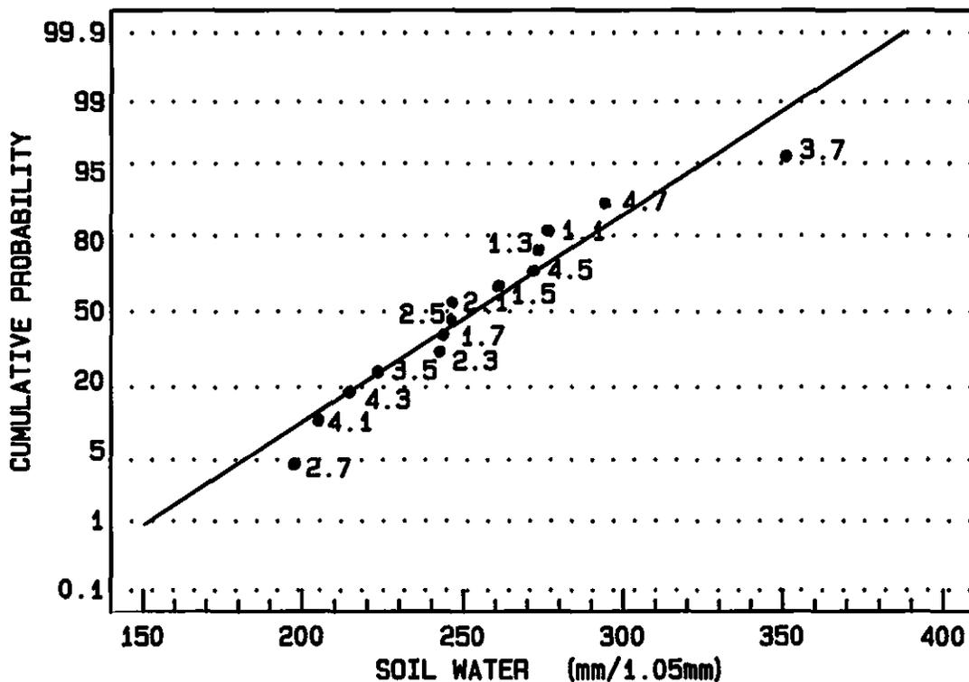
Figure 4.3 Cumulative probability density curve of the soil water content that was gravimetrically determined at 14 sites in a drip irrigated vineyard in May 1987. The numbers are the identification codes for the sampling sites
