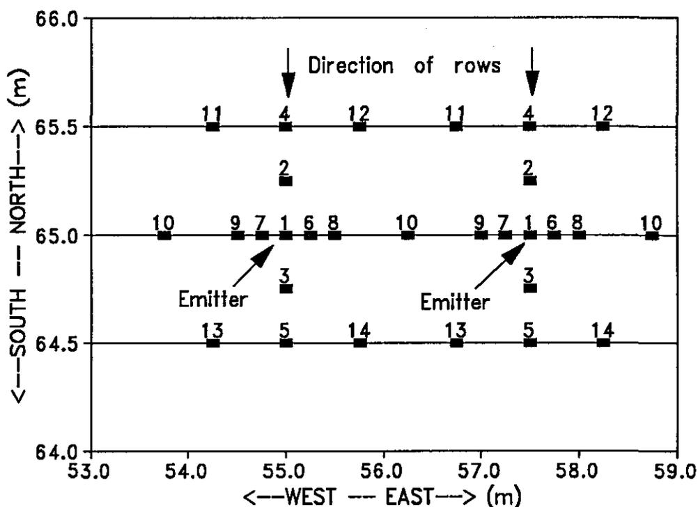
Figure 6.2 Diagram indicating the 14 positions at different directions and distances from two emitters where the soil water content was monitored during November 1988 and 1989
