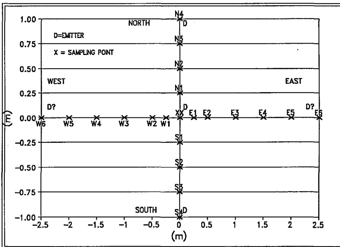
Figure 2.2 Schematic diagram of the sampling scheme used in December 1986; the 21 positions surrounding one emitter is shown (the same scheme was used at sites A1, A2, A3 and A4)
