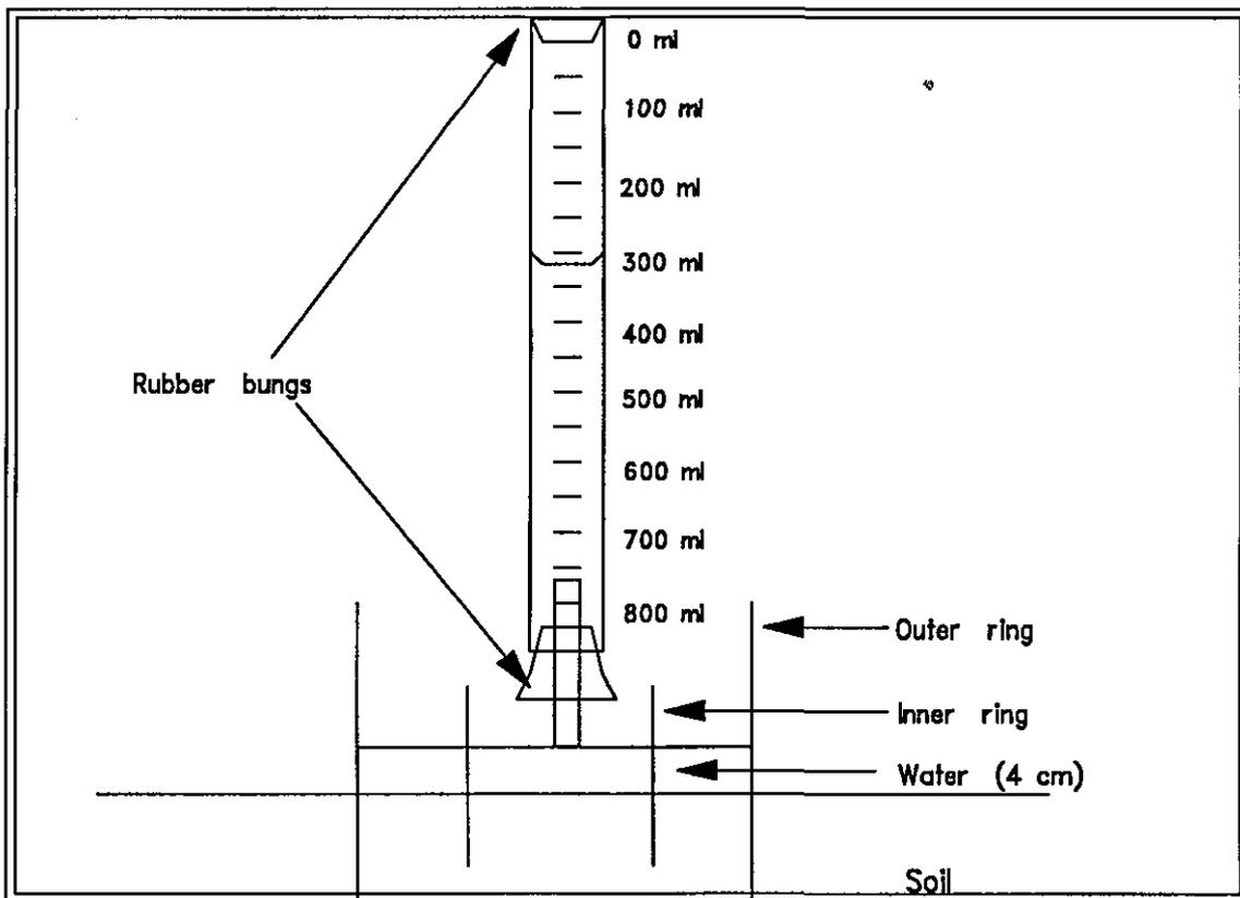
**Figure 2.7** Schematic diagram of the infiltrometer that was used to determine the infiltrability of the soil at Robertson
