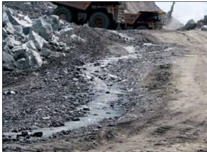
Groundwater inflows into open-pit area.
