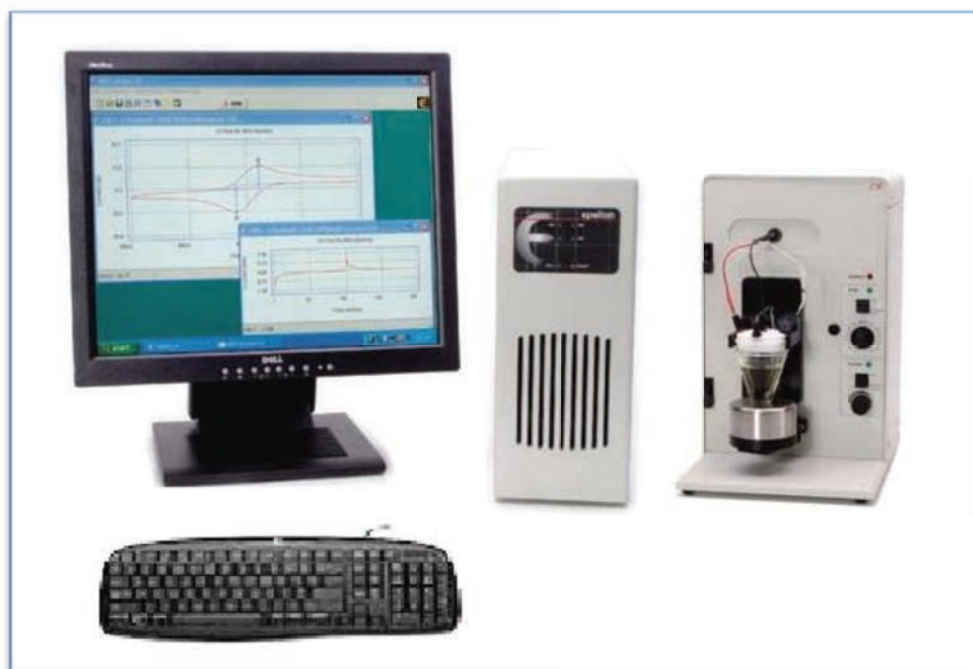
Figure 28. Epsilon electrochemical workstation and analyser, with the batch cell conventional three electrode set-up for the electrochemical determination of metal ions in aqueous solution (Van der Horst, 2011).
