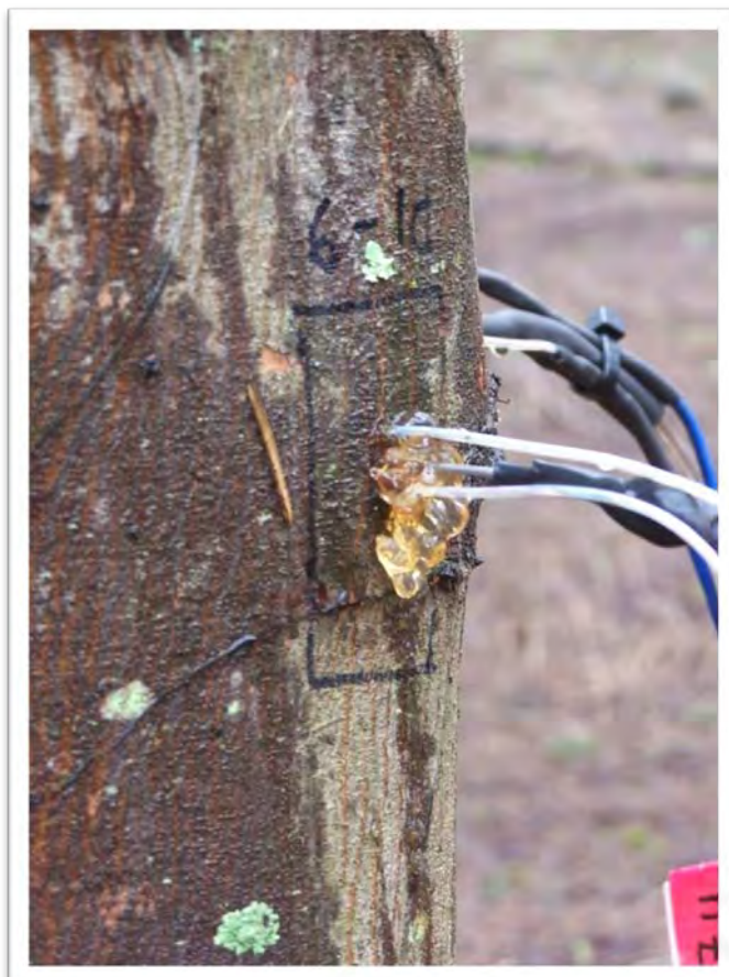
Figure 3.15: At the location of the wounding where the probes are inserted, the A. mearnsii trees produce a gum that is corrosive and can adjust the depth of the probes in the sapwood.
