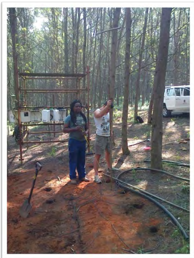
Figure 3.23: Auguring holes for the installation of the TDR UKZN probes at 0.4 m intervals down to 4.8 m.
