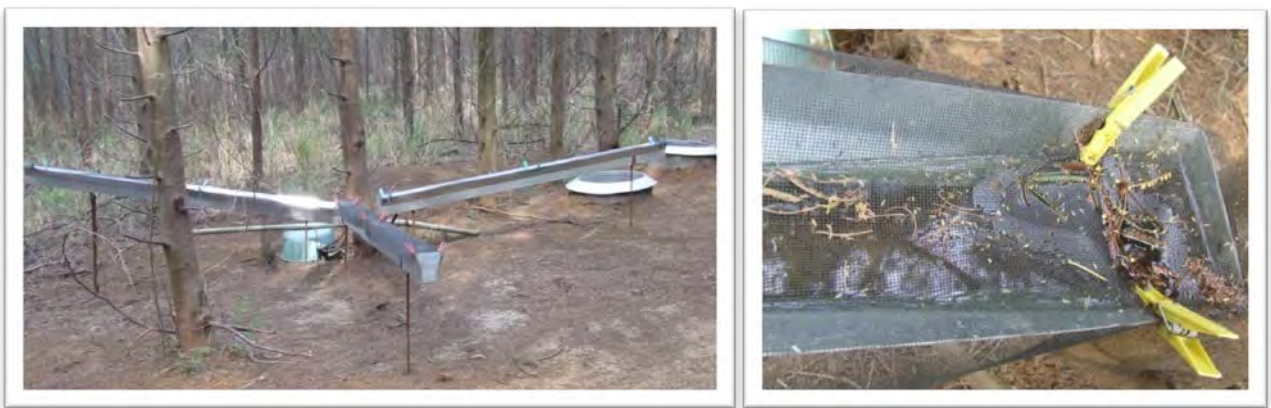
Figure 3.2: Throughfall troughs with a covering of mosquito netting (a) and a blockage due to leaves in the trough outlet (b).
