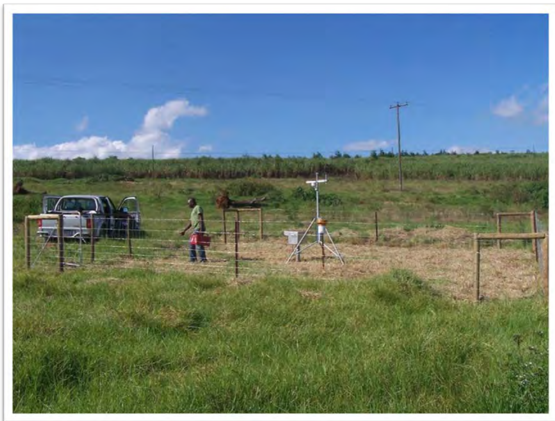
Figure 3.10: Automatic weather station near the Two Streams site established over short grass and used to calculate the short grass ASCE reference evaporation.
