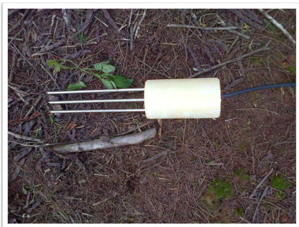
Figure 3.22: The TDR UKZN cylindrical probes have 0.15 m long waveguides.
