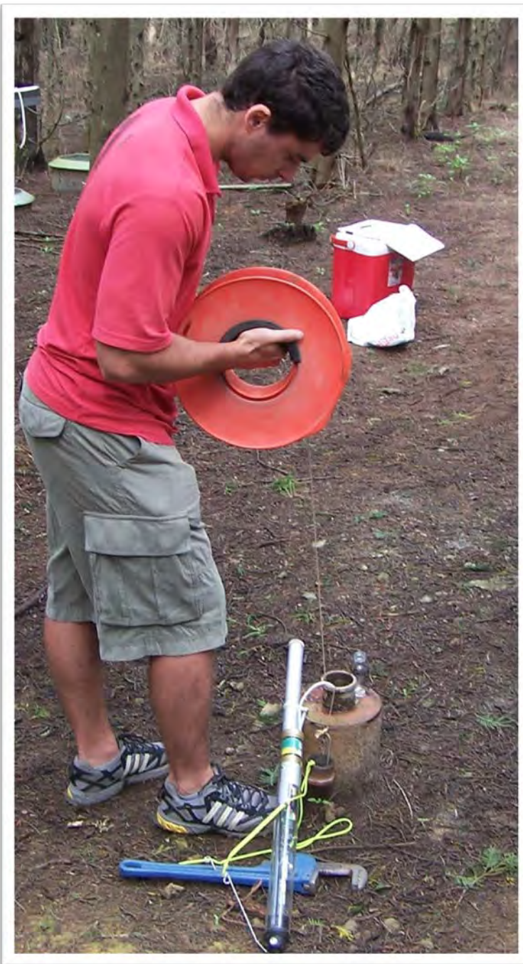
Figure 3.18: The Ott Orphimedes water level logger lies next to the borehole casing while a student collects a groundwater sample.
