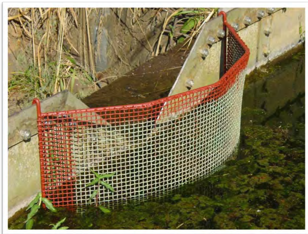
Figure 3.16: The old sieve in the main weir at Two Streams in 2006 kept leaves and branches from getting trapped in the V-notch.
