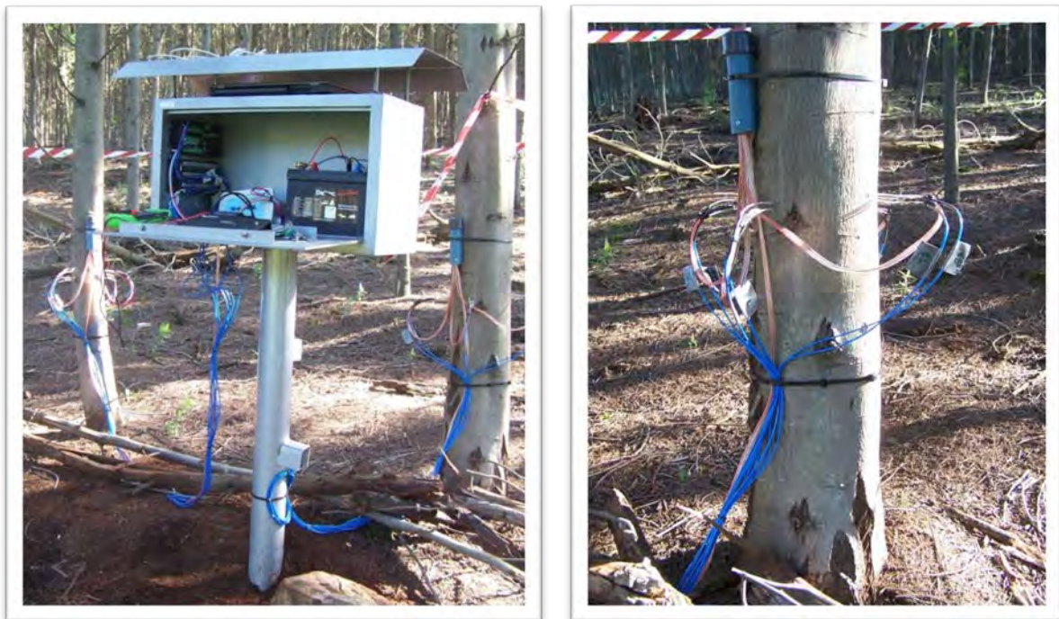
Figure 3.14: A metal security enclosure on the left housed the HPV data logger, multiplexer, relay control module and battery. On the right the thermocouple and heater probes inserted into an A. mearnsii tree.
