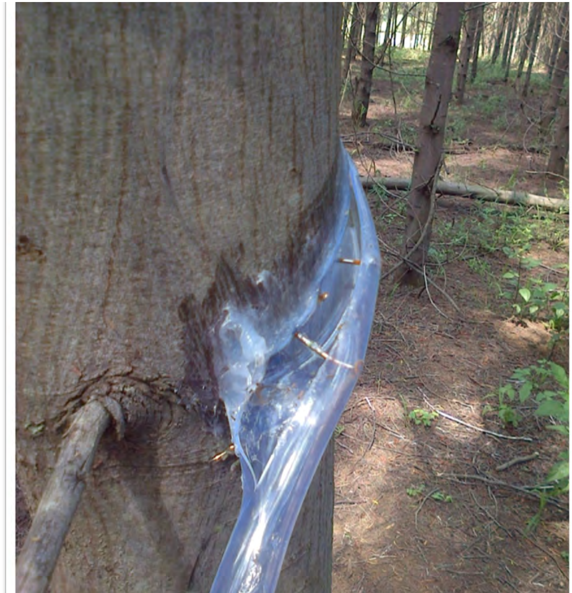
Figure 3.5: A close-up view of the silicone tube glued with silicone sealant to the bark of the stem that collects stemflow.
