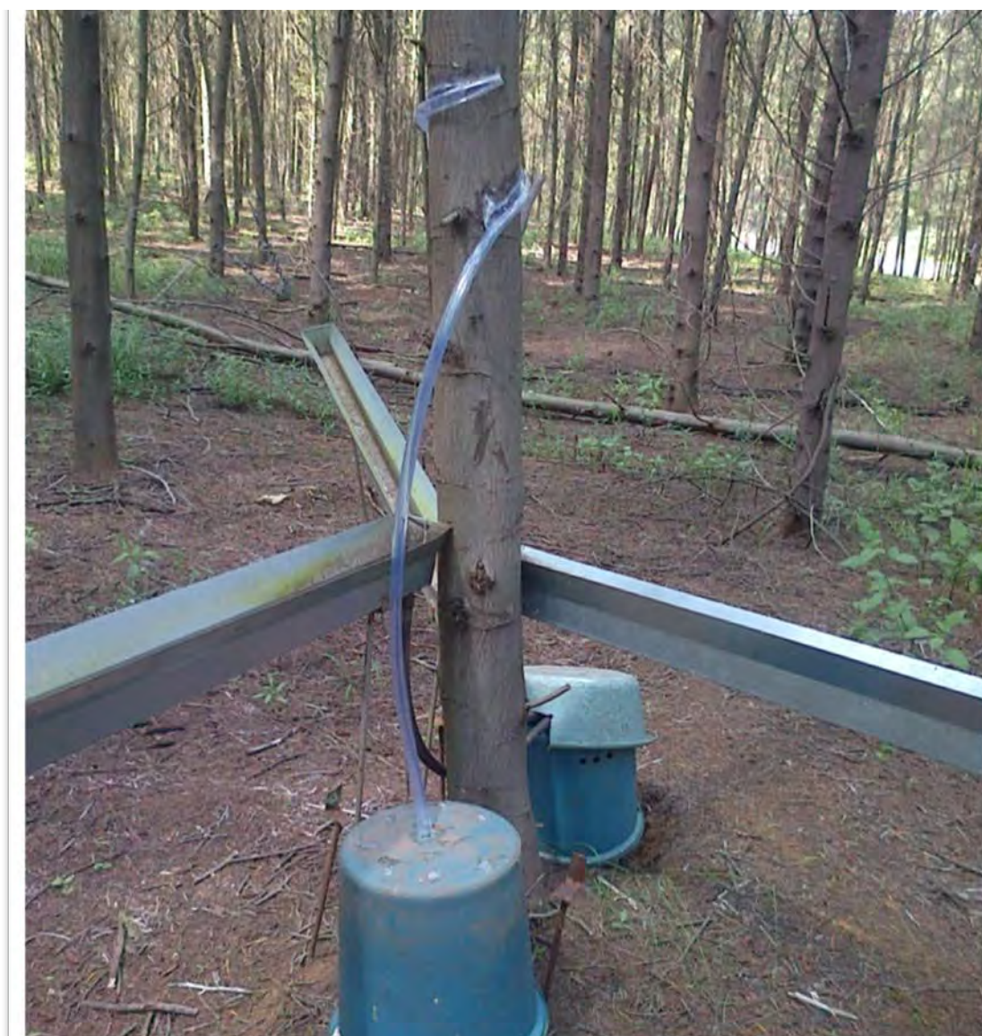
Figure 3.4: Silicon tube and tipping bucket rain gauge to measure stemflow.
