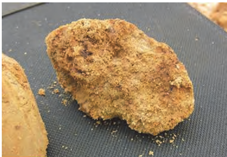
Figure 4-37 Mottled appearance of soil taken from hole drilled for salinity
