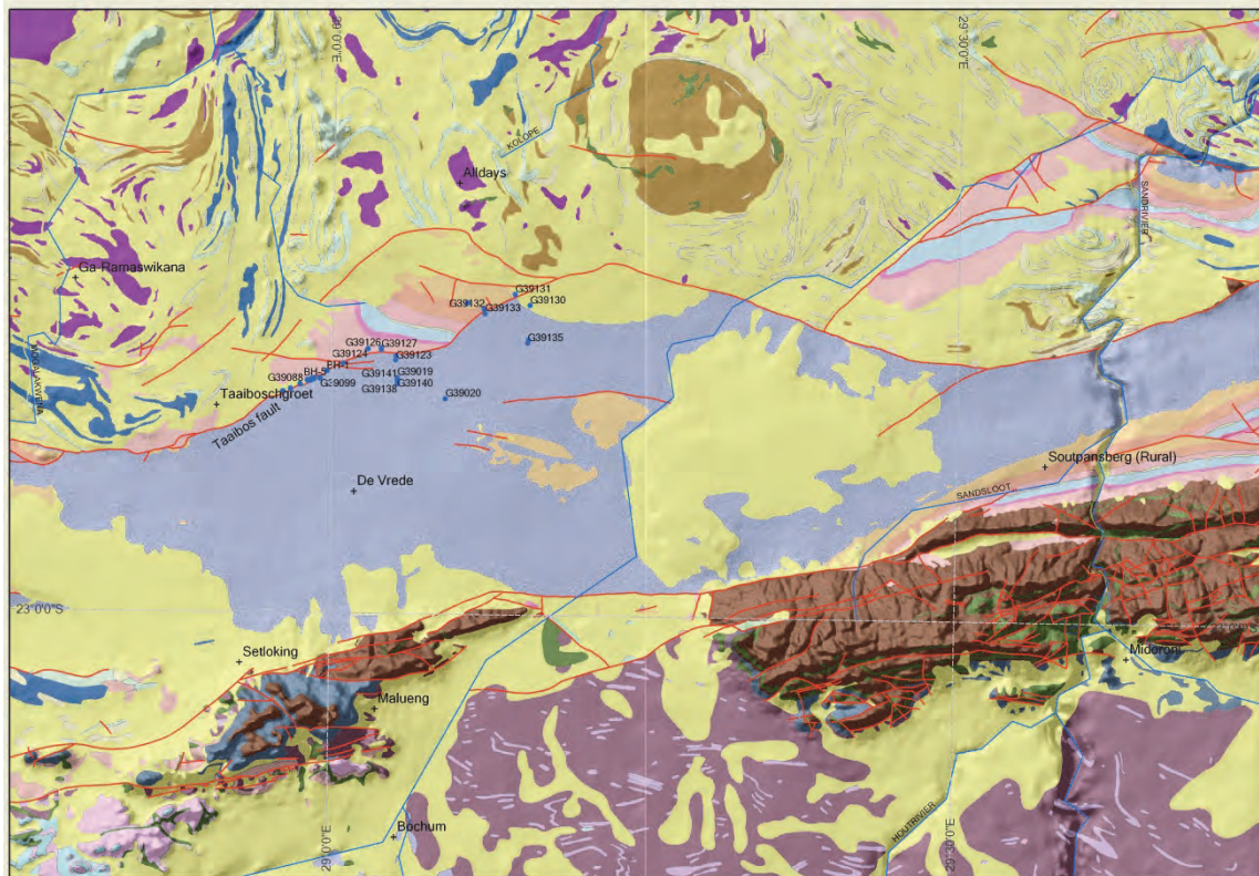
Figure 16 Map showing the Taabos fault and boreholes drilled in the Alldays area
