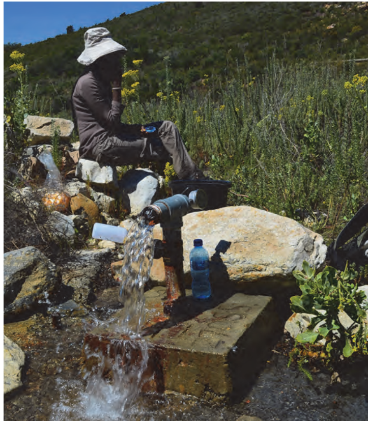
Figure 10 Constant head test at BH-1 on 14 to 16 October 2013
