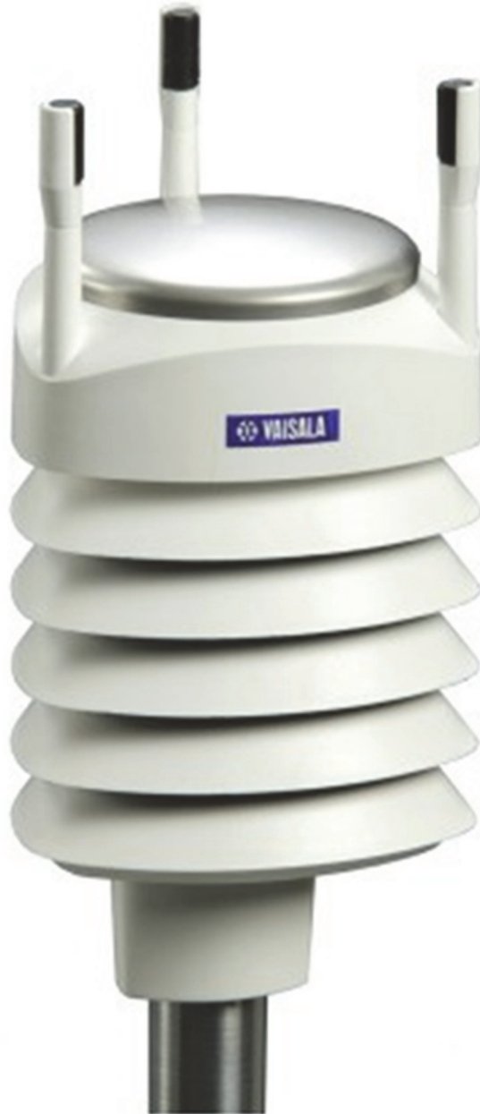
Figure 2.16: The Vaisala WXT520 weather transmitter
