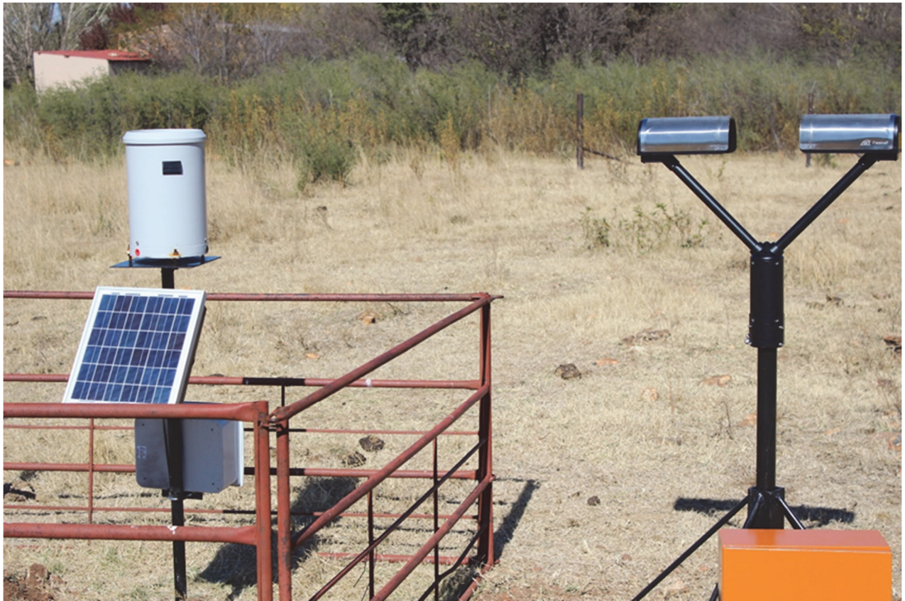
Figure 2.15: The NWU OTT parsivel disdrometer
