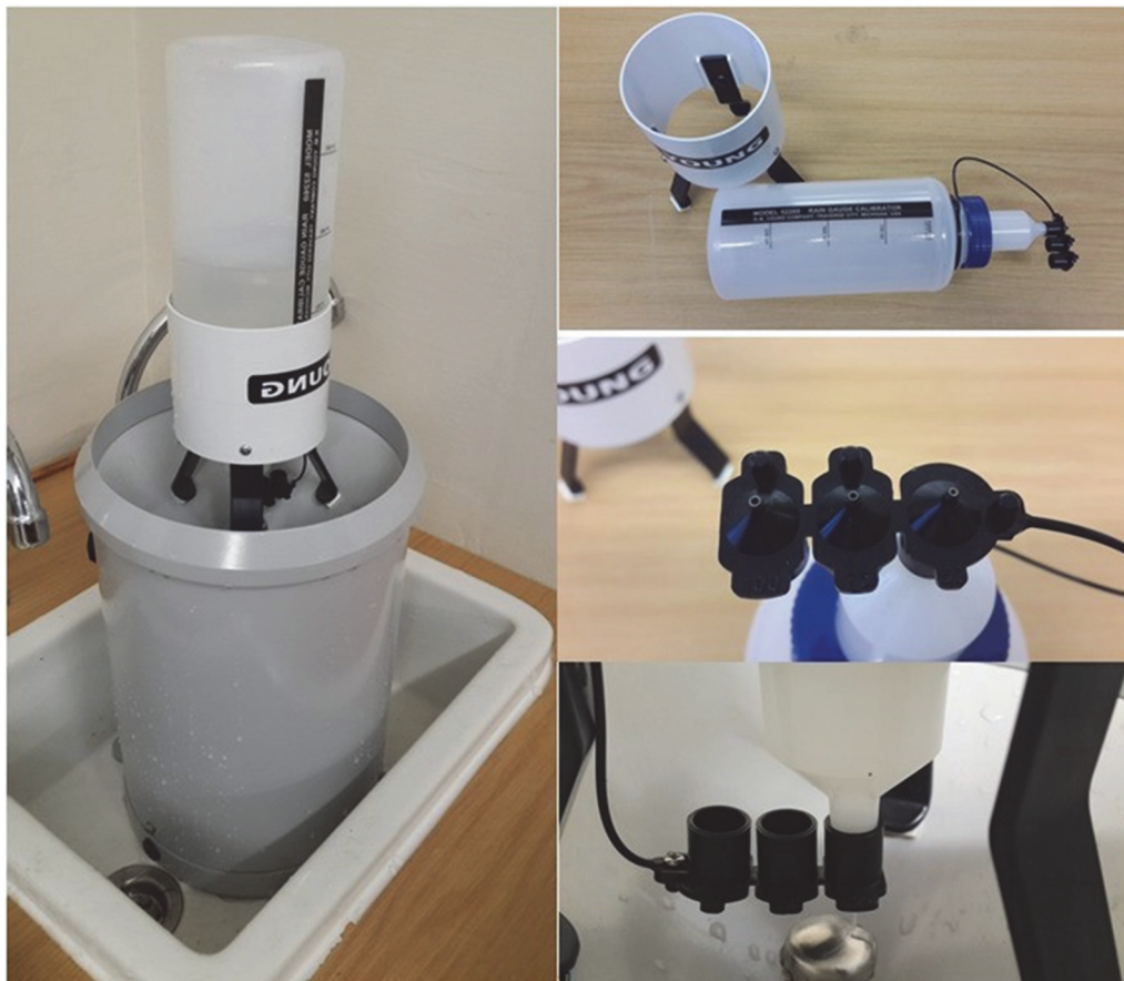
Figure 2.13: The tipping bucket calibration kit
