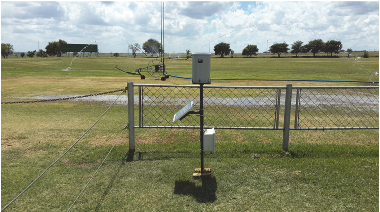
Figure 2.22: The irrigation of a rugby field at Site 10 (Carletonville), causing false data to be recorded by the rain gauge
