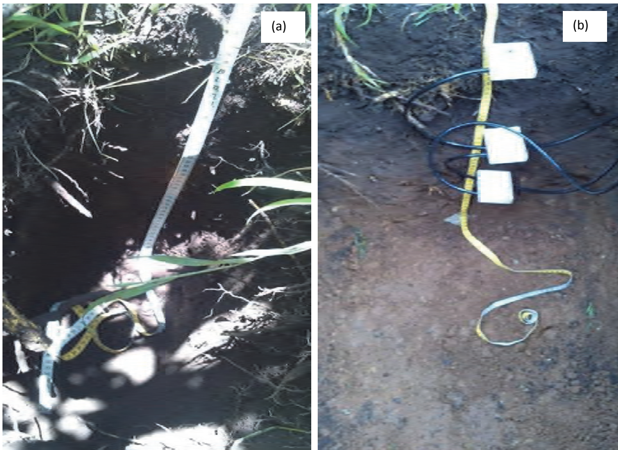
Figure 3.26 Soil profiles at site 1 (a) and 3 (b), with CS 616 probes installed at New Forest
