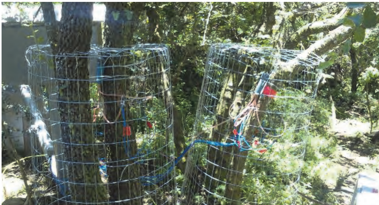
Figure 3.12 HPV system installation of tree 1 ( Searsia pyroides ), 2 ( Maytenus peduncularis ) and 3 ( Leucosidea sericea ) at New Forest farm
