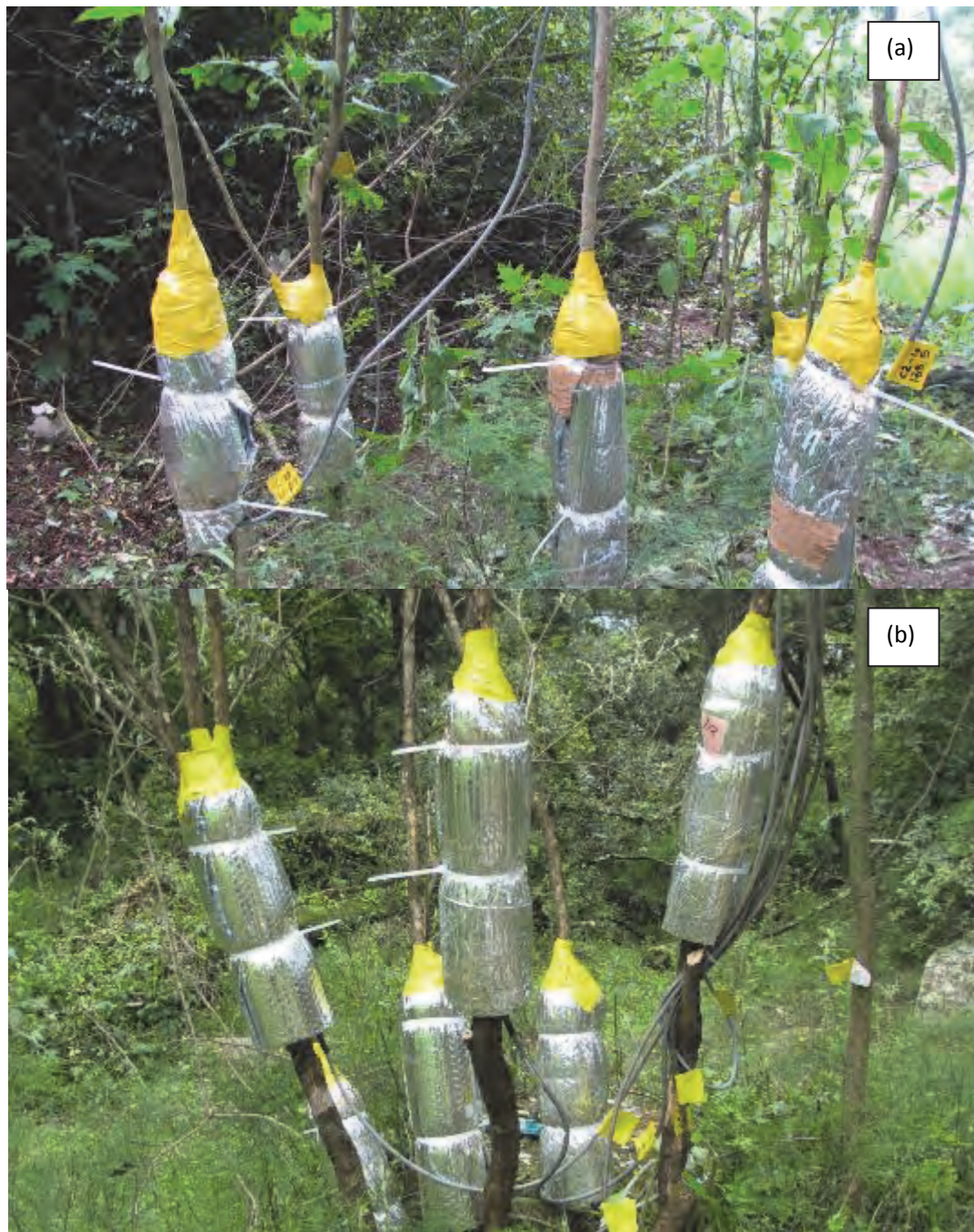
Figure 3.21 Dynamax system installation of Solanum mauritianum (a) and Buddleja salviifolia (b) at New Forest farm
