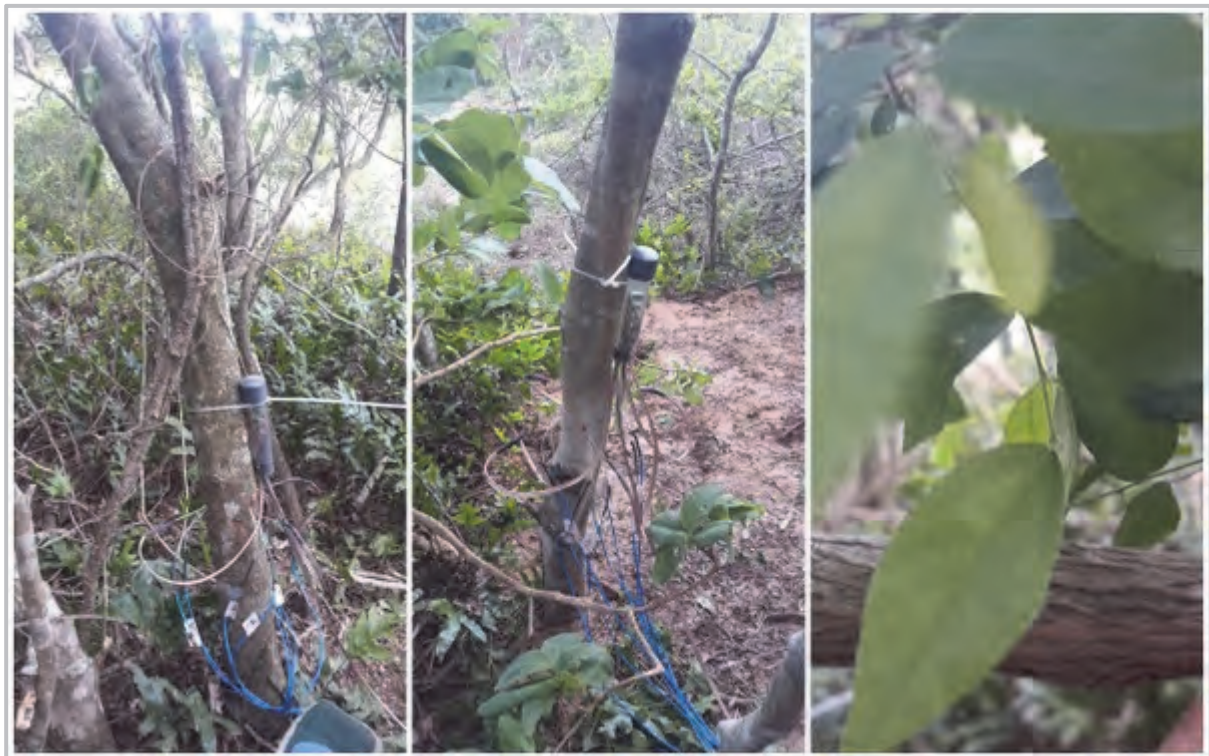
Figure 3.17 HPV system installation of tree 1 ( Shirakiopsis ellipticum ), 2 ( Albizia adianthifolia ) and 3 ( Shirakiopsis ellipticum ) at Vasi North
