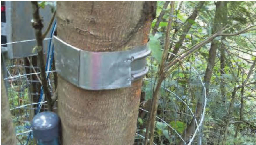
Figure 3.29 Dendrometer collar installed on an Acacia mearnsii at New Forest farm
