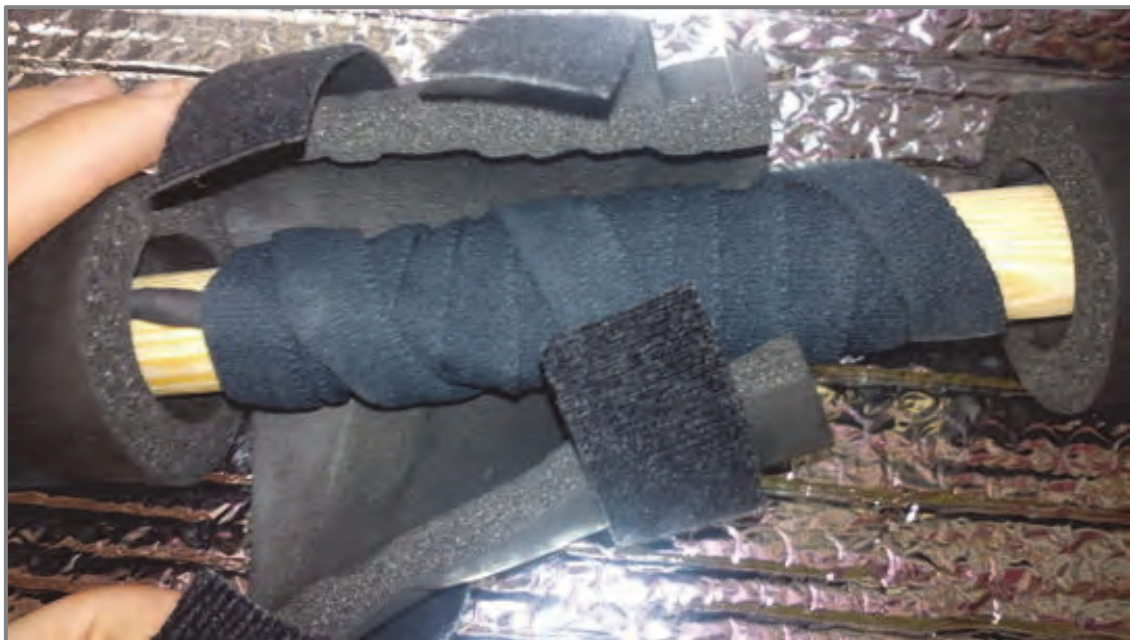
Figure 6.17 Dynamax EXO skin collar used on irregular/asymmetrical stems
