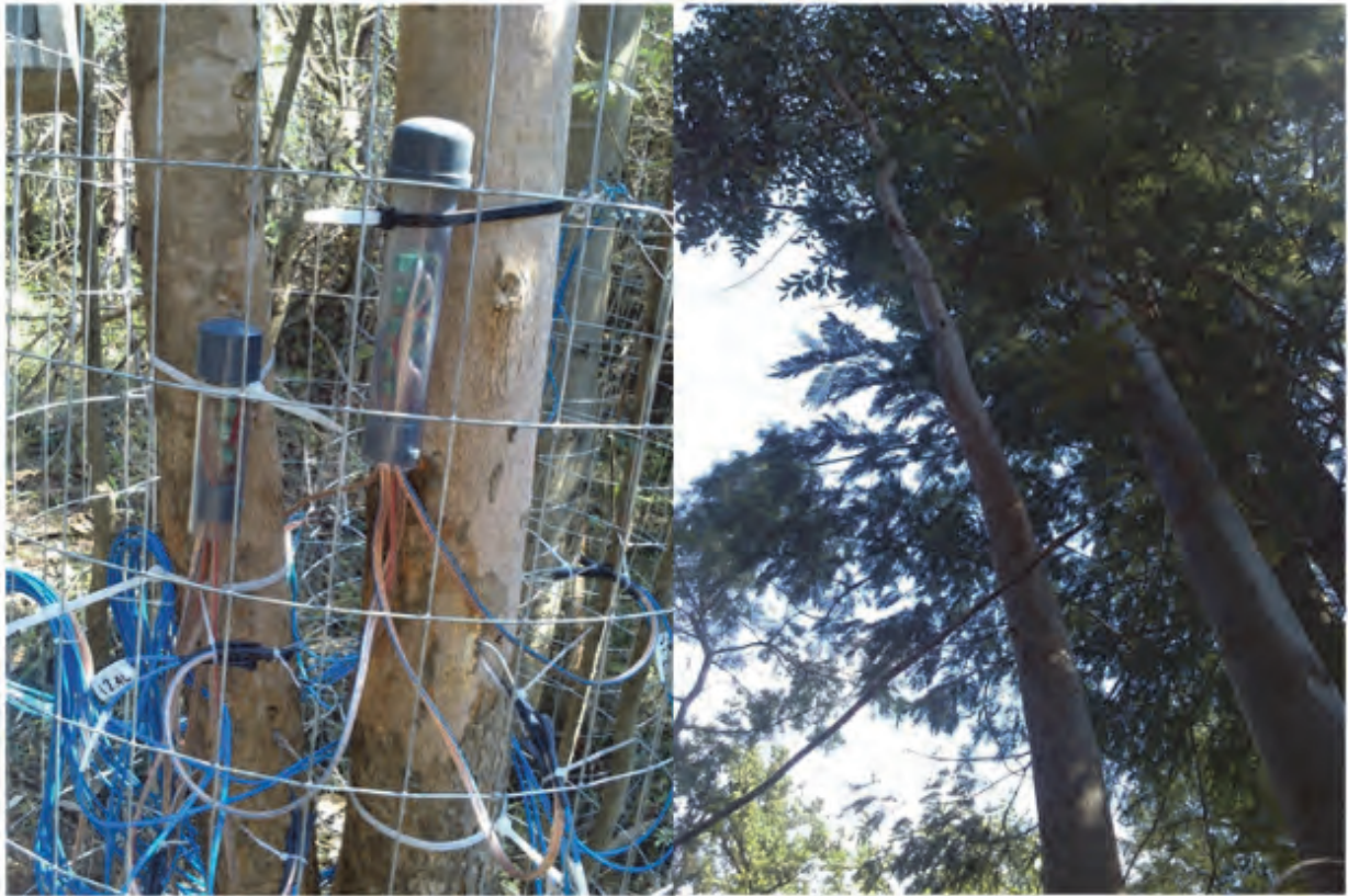
Figure 3.15 HPV system installation of trees 10, 11 and 12 ( Eucalyptus grandis and Acacia mearnsii ) at New Forest farm
