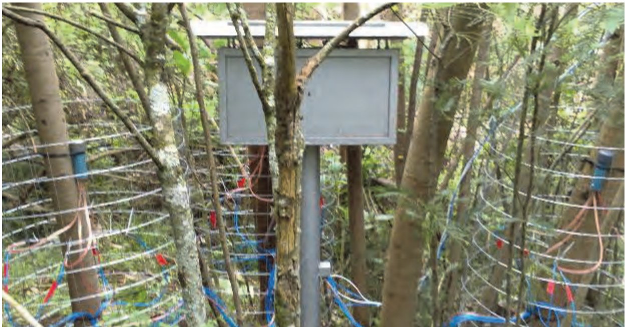
Figure 3.14 HPV system installation of trees 8, 9 and 10 ( Acacia mearnsii ) at New Forest farm
