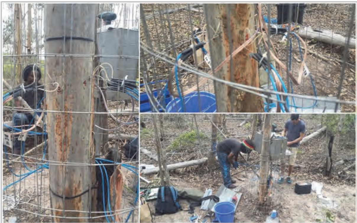
Figure 3.19 HPV system installation of trees 7, 8 and 9 ( Eucalyptus grandis ) at Vasi North
