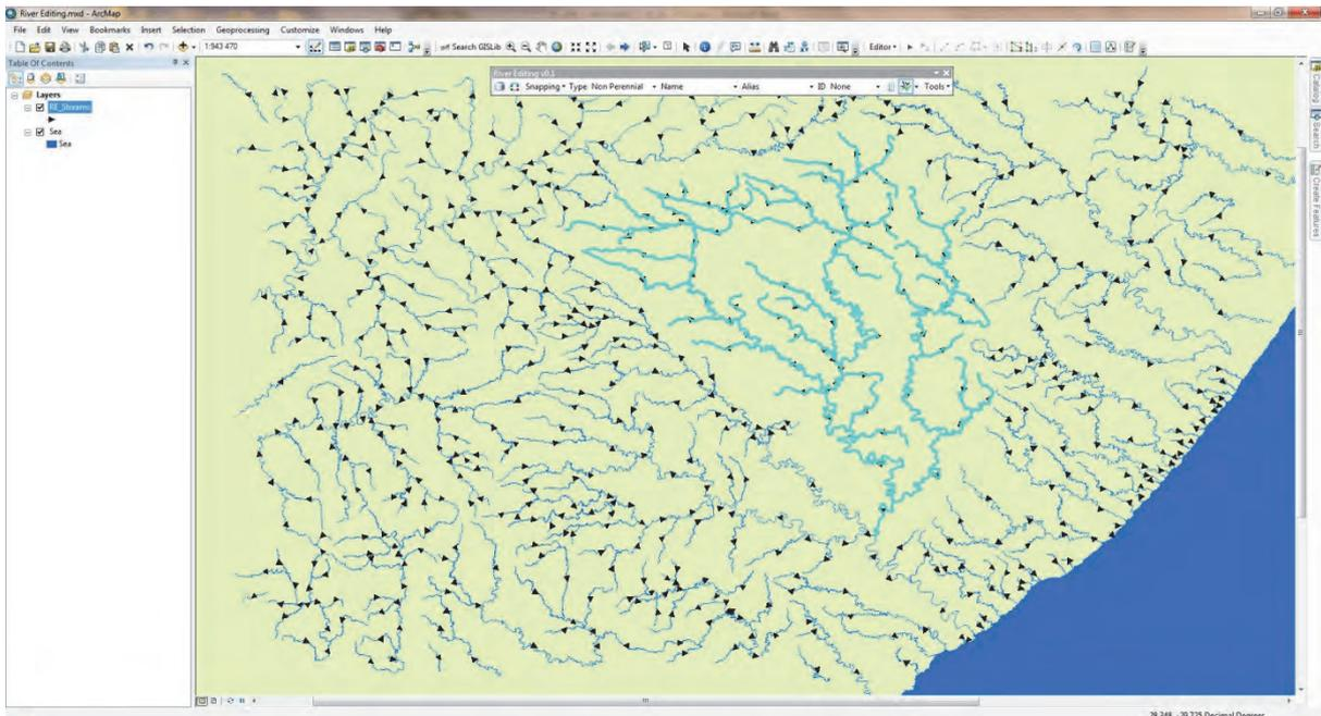
**Figure 42: Rivers that are not pointing downstream highlighted for the purpose of identifying them**
