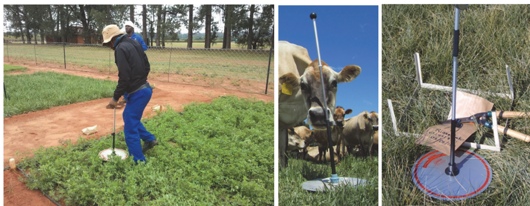
Figure 2.10 Yield measurements using a Rising Plate Meter
