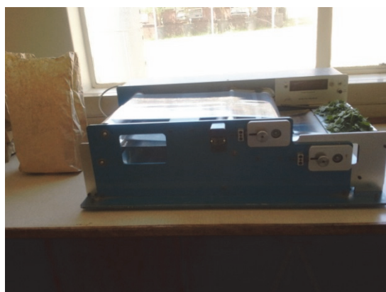
Figure 2.9 Belt driven Licor LAI-3100 for measuring leaf area index
