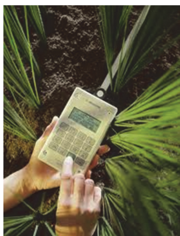
Figure 2.8 Decagon's AccuPAR model LP-80 PAR/LAI Ceptometer for measuring Fractional interception of photosynthetic active radiation
