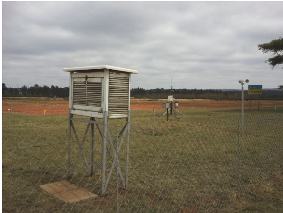
Figure 2.5 The automatic weather station
