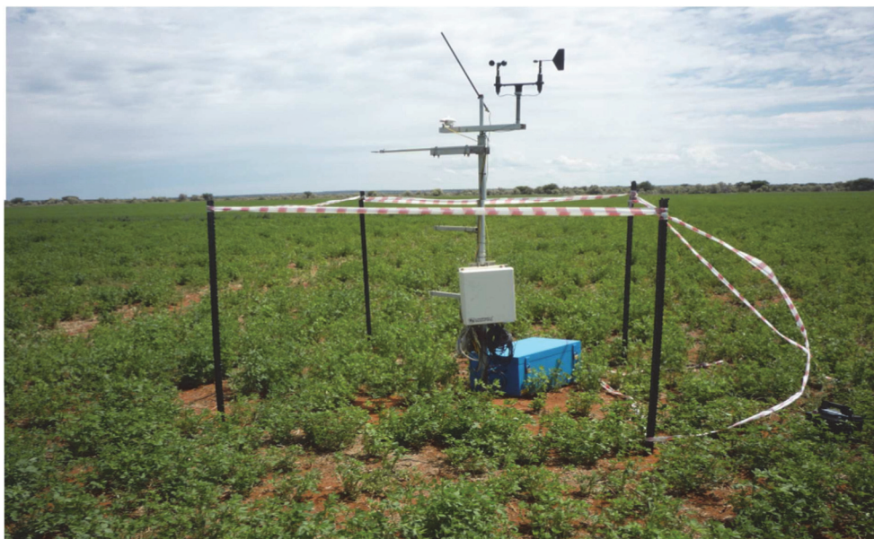
Figure 6.4 Eddy covariance system installed at lucerne field in Douglas
