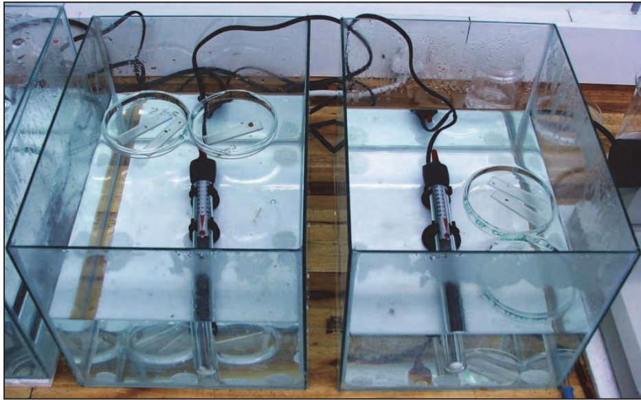
Figure 6.6. Aquarium tanks, heaters and petri dishes for egg hatching experiments
