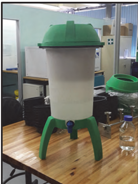
Figure 2.4 Final produced housing unit assembled in the laboratory
