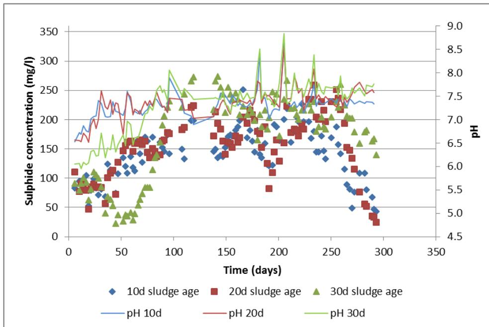
Figure 30 Batch reactor results of sulphide production at 30°C
