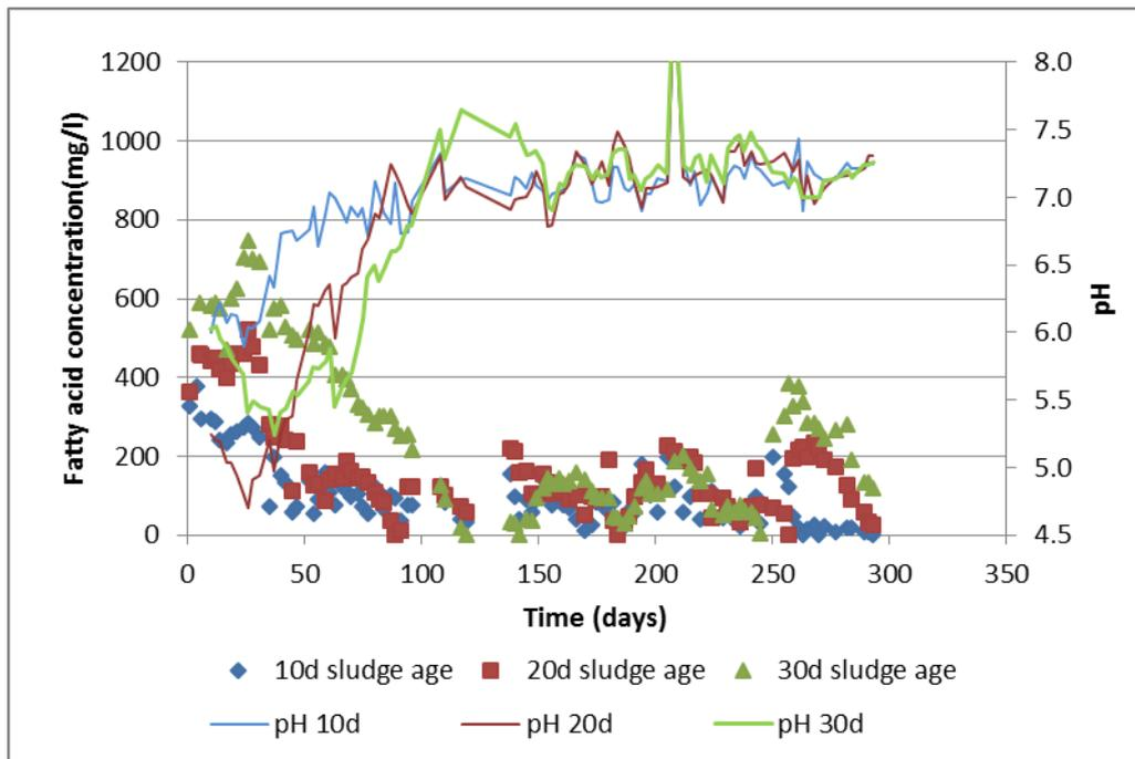
Figure 22 Batch reactor results of VFA at 15°C
