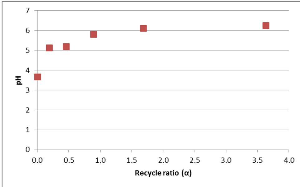
Figure 38 Effect of the recycle ratio on pH
