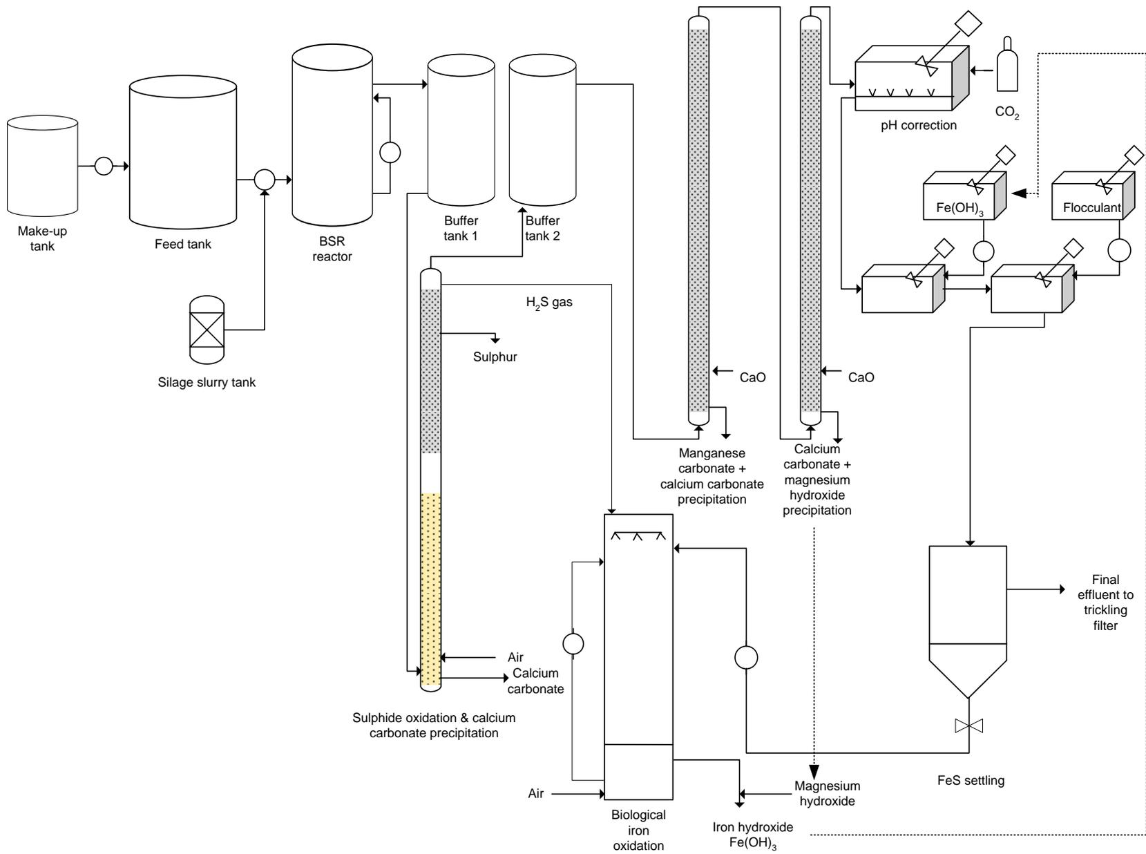
Figure 34 Schematic layout of the pilot reactor, excluding acid neutralization
