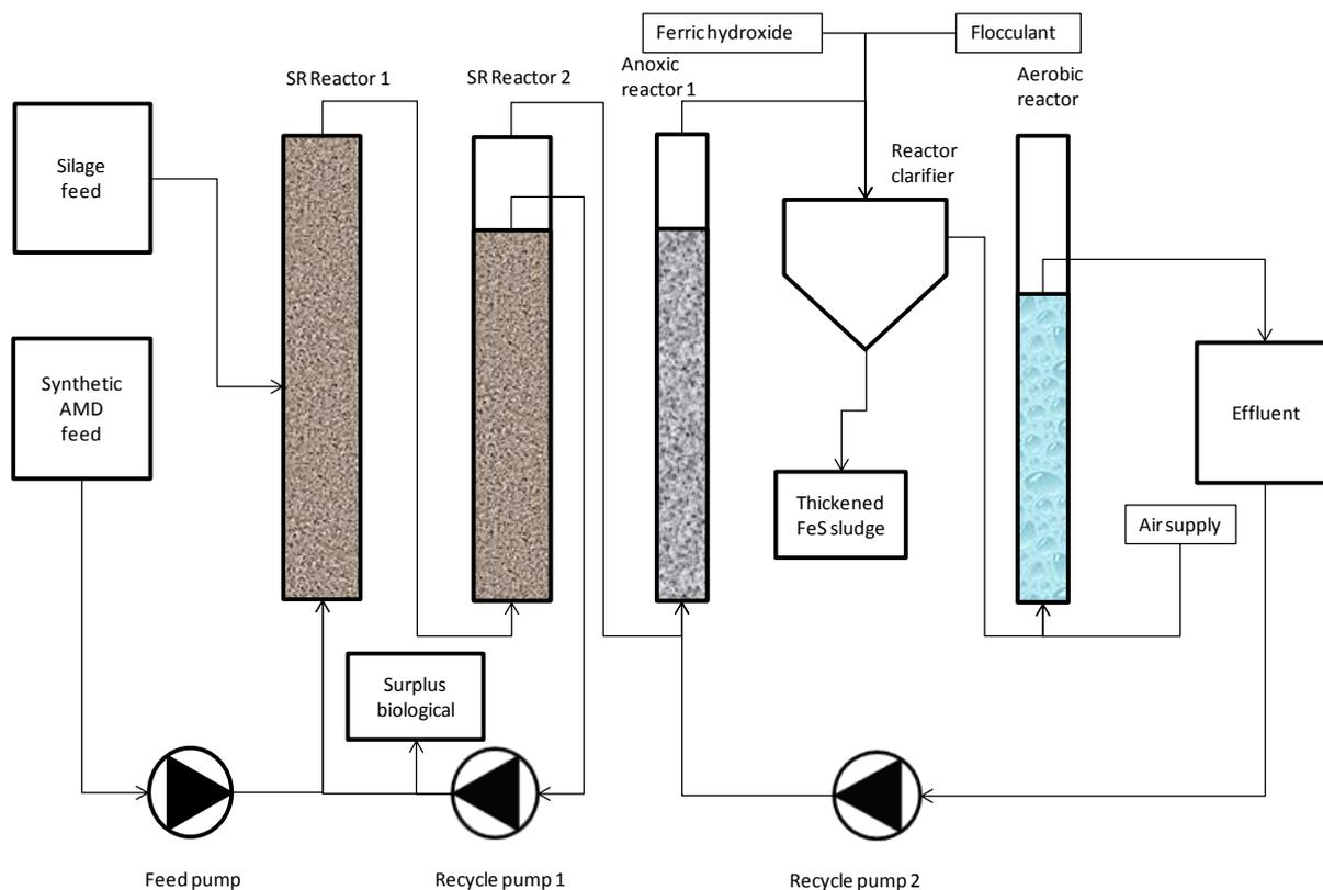
Figure 13 Schematic layout of the 40 L/d continuous process
