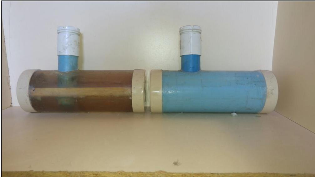
Figure 11 Picture showing the details of the containers. The transparent container on the left-hand side shows how the tube extends into the container. It also shows the baffle inside the container for mixing.
