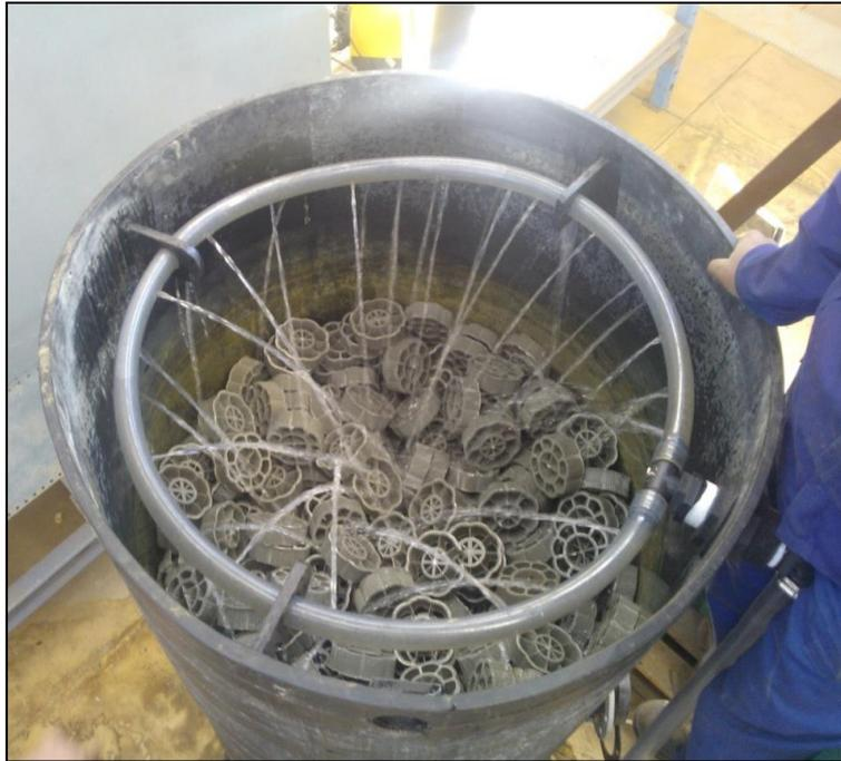
Figure 50 Biological iron oxidation reactor showing the distribution of recycled ferrous sulphate solution on top of the rosettes (right)
