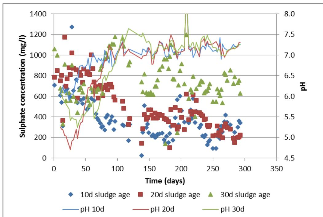
Figure 19 Batch reactor results of sulphate reduction at 15°C
