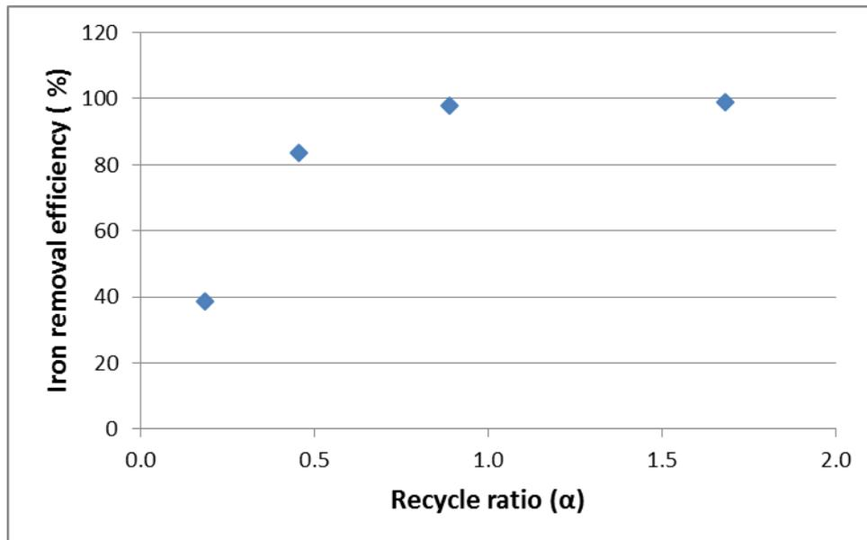
Figure 37 Effect of recycle rate on iron removal
