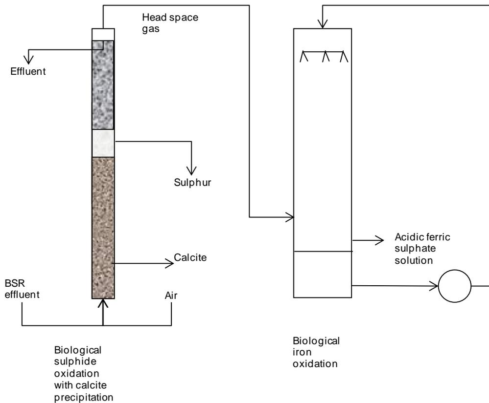
Figure 43 Biological sulphide oxidizing reactor combined with calcite precipitation and integrated with the biological iron-oxidizing reactor
