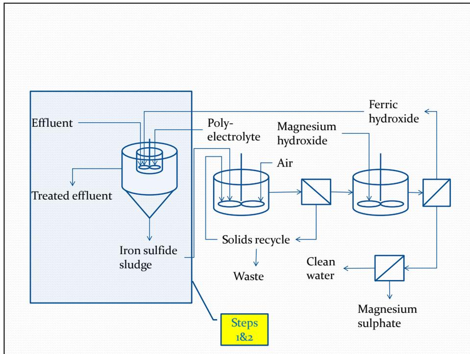
Figure 46 Steps 1 and 2 of the proposed sulphide removal process
