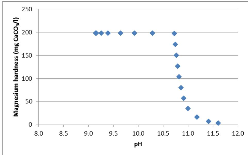
Figure 44 Magnesium hydroxide precipitation as a function of pH
