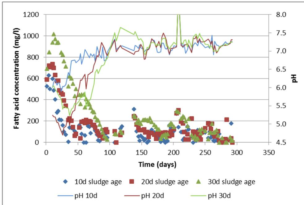
Figure 32 Batch reactor results of VFA (volatile fatty acids) at 30°C
