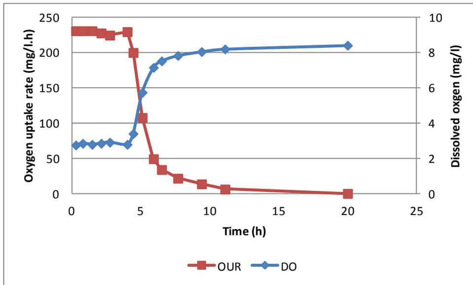
Figure 14 Dissolved oxygen and measured OUR during the chemical oxidation of FeS
