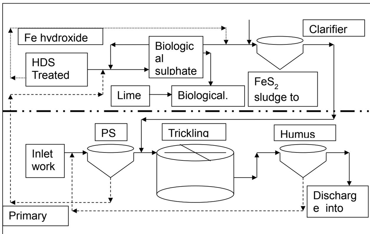
Figure 1 Simplified diagram of the Rhodes BioSURE® Process
