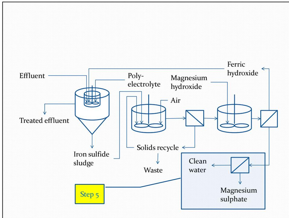
Figure 49 Step 5 of the sulphide removal process
