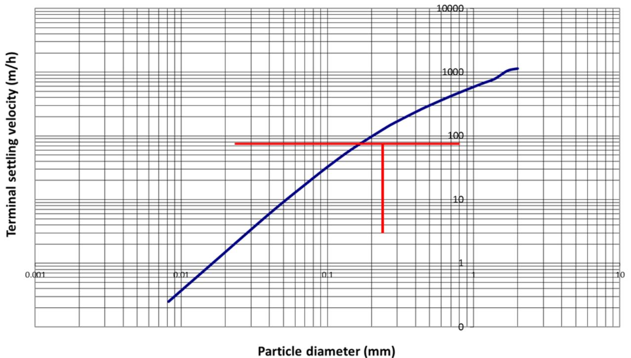
Figure 42 Terminal settling velocity of limestone particles in water as a function of particle size
