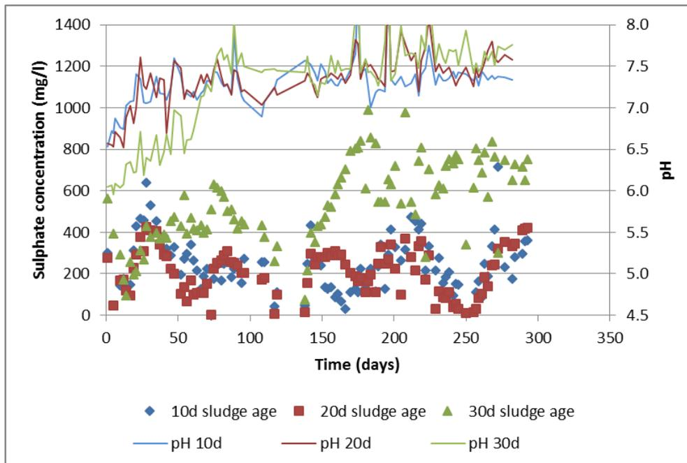
Figure 29 Batch reactor results of sulphate reduction at 30°C
