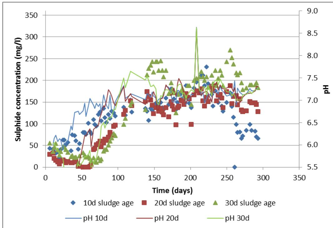
Figure 20 Batch reactor results of sulphide production at 15°C
