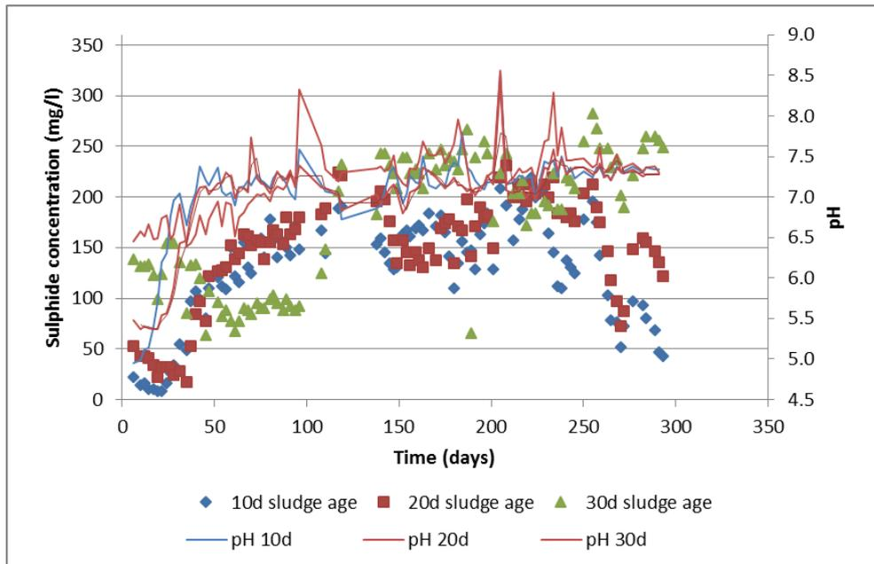
Figure 25 Batch reactor results of sulphide production at 25°C
