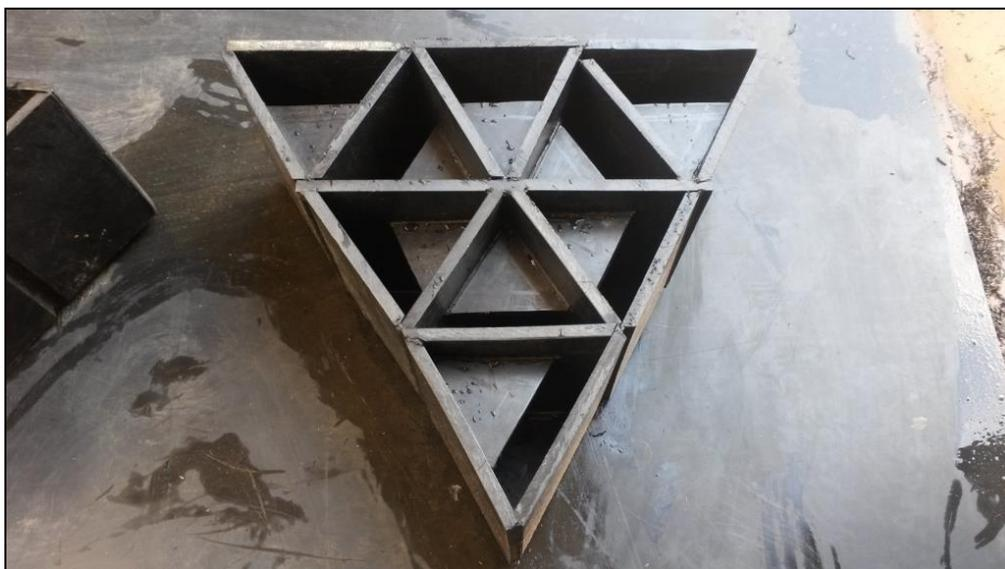
Figure 8 Triangular assembly of 9 reactors shown with the dividing baffles
