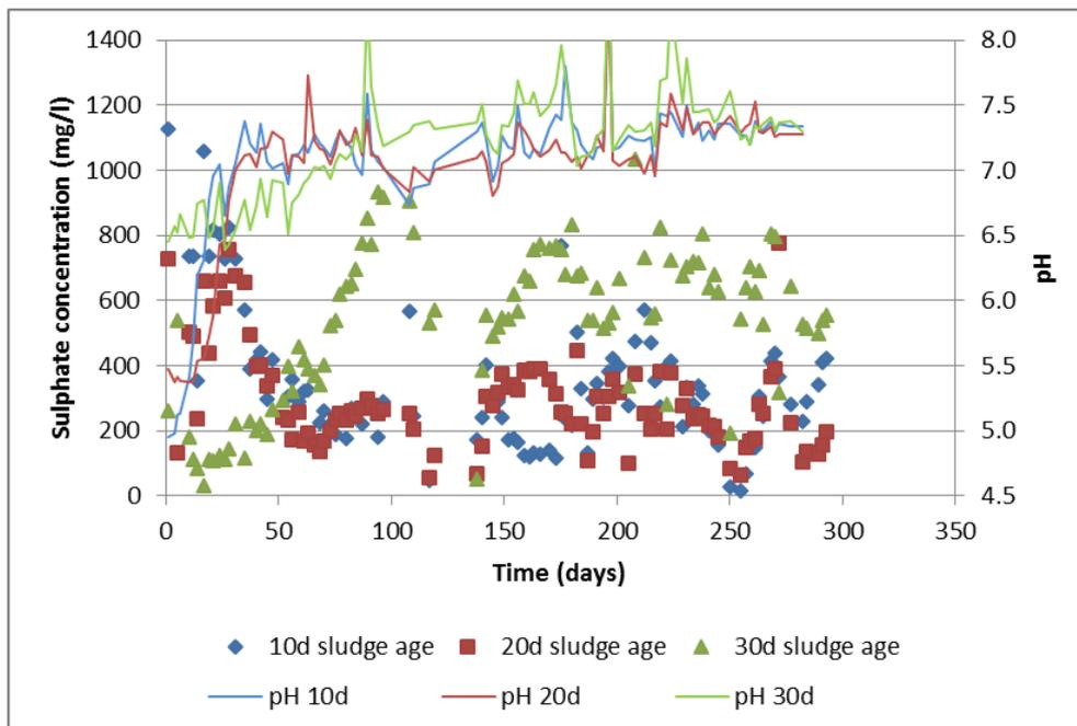
Figure 24 Batch reactor results of sulphate reduction at 25°C
