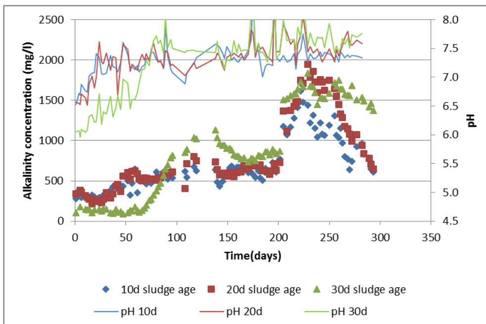
Figure 31 Batch reactor results of alkalinity production at 30°C
