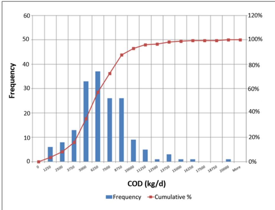
Figure 6 Available primary sewage and humus sludge (as COD) at the Ancor WWTP for the operation of the Rhodes BioSURE® Process
