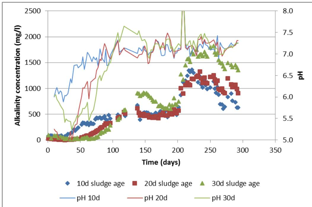
Figure 21 Batch reactor results of alkalinity production at 15°C
