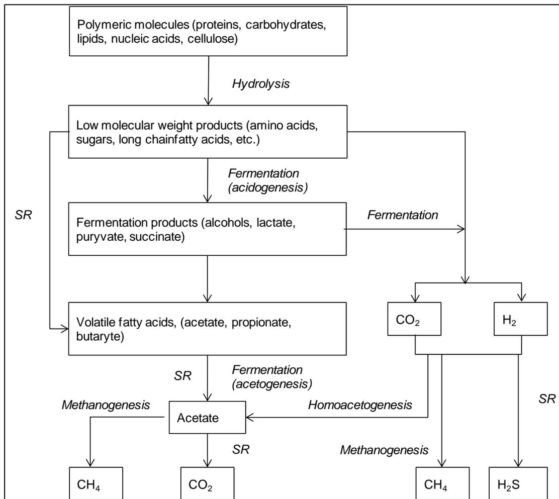
Figure 2 Step-wise anaerobic degradation of organic material and consumption by methanogenic bacteria and SRP (adapted from Nevatalo, 2010). SR = sulphate reduction.
