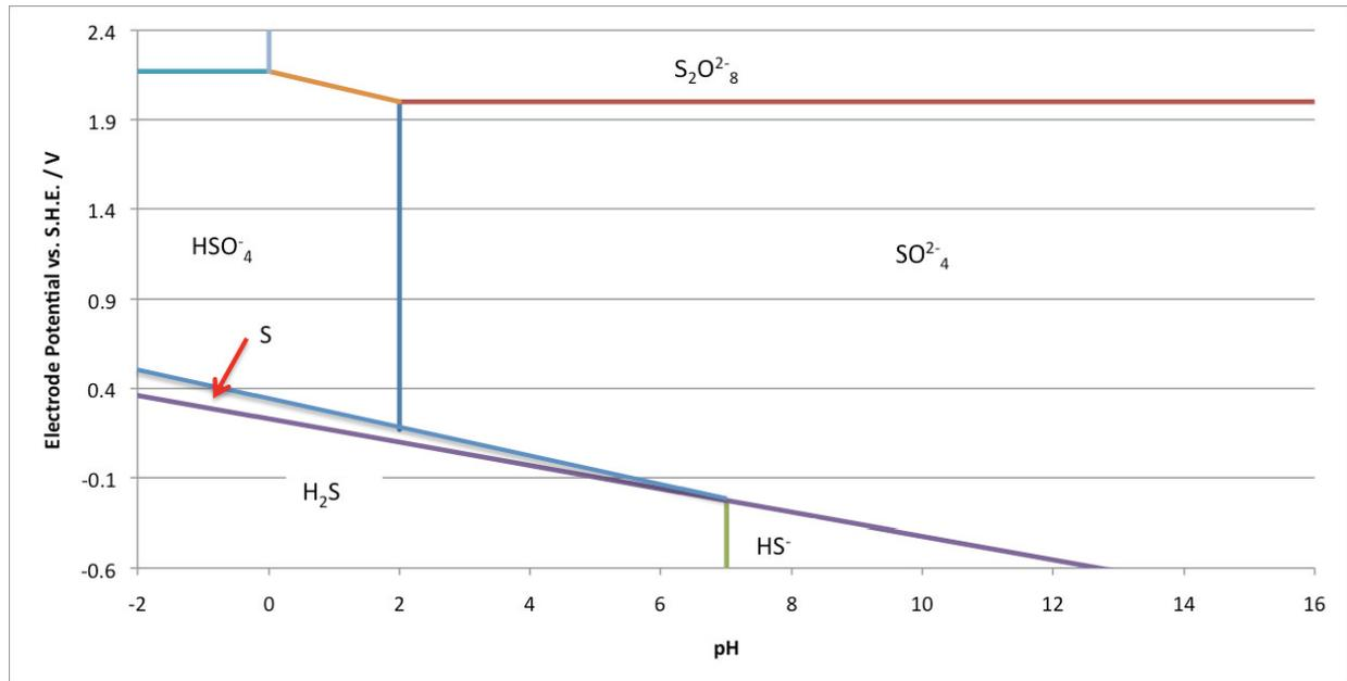
Figure 4: Potential-pH diagram for a sulphur/water system at 298.15 K (Van Hille et al., 2012)
