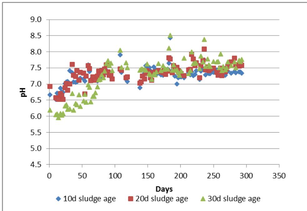
Figure 33 Batch reactor pH at 30°C
