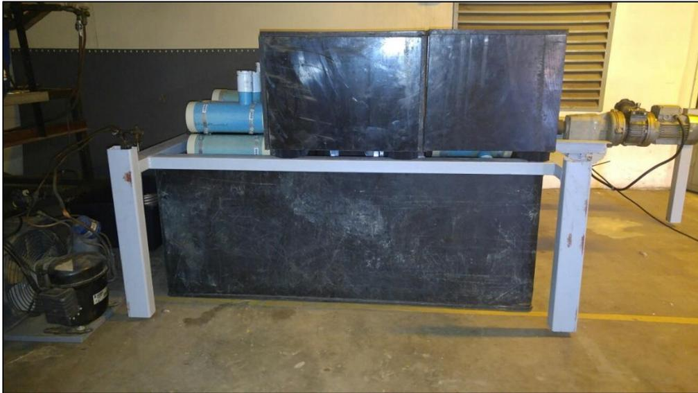
Figure 10 Batch reactors with the cover of one of the three enclosures removed. The temperature in each of the enclosures was independently controlled
