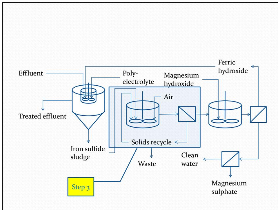
Figure 47 Step 3 of the proposed sulphide removal process
