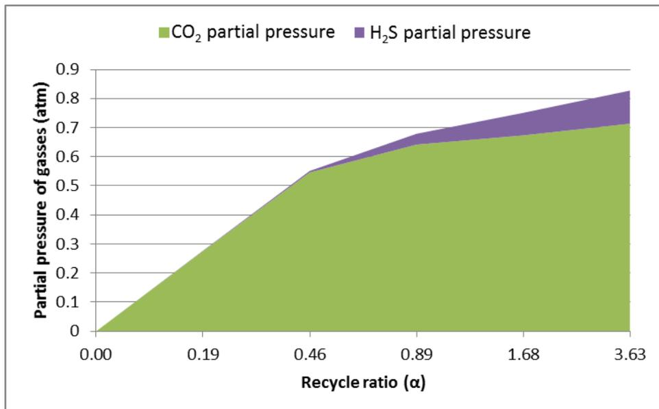
Figure 39 CO<sub>2</sub> and H<sub>2</sub>S partial pressures as a function of the recycle ratio
