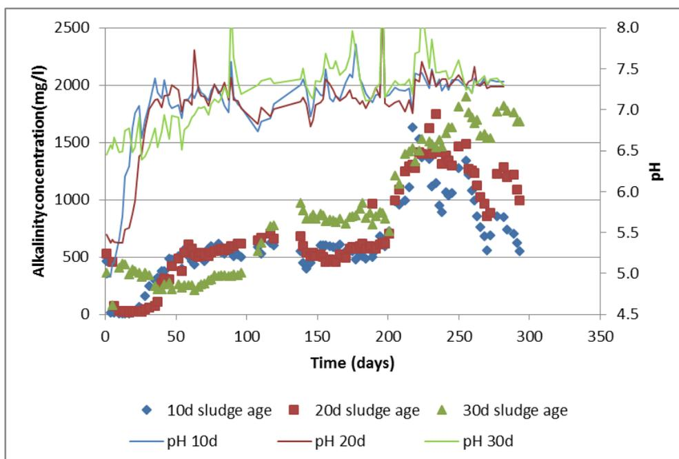
Figure 26 Batch reactor results of alkalinity production at 25°C
