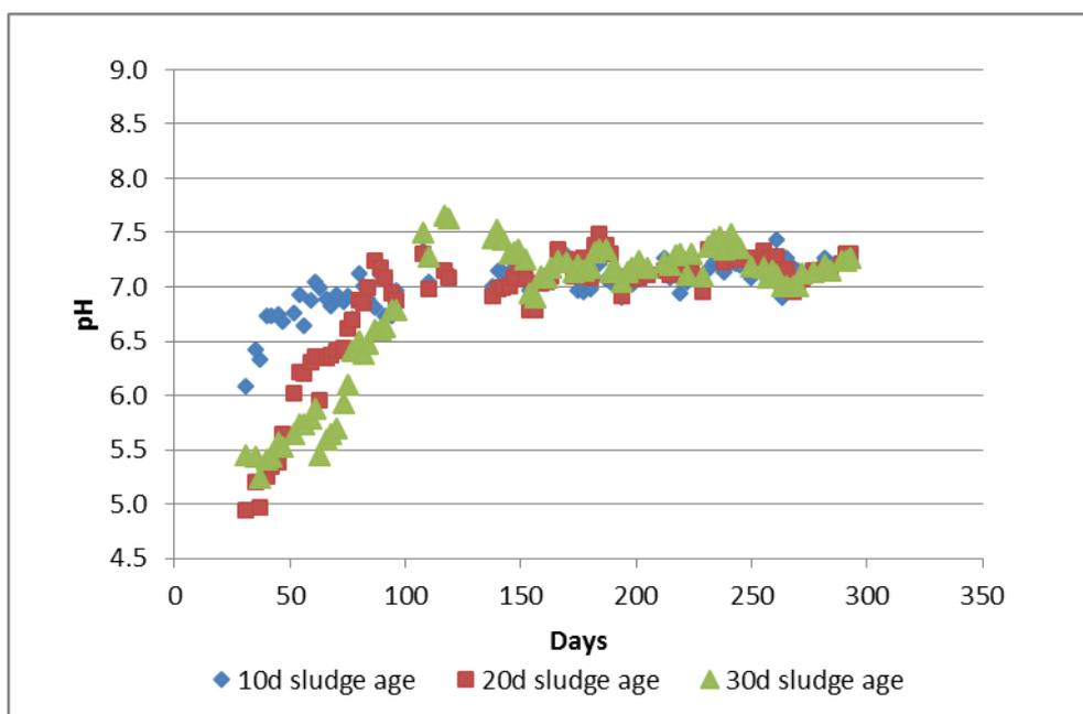
Figure 23 Batch reactor pH at 15°C
