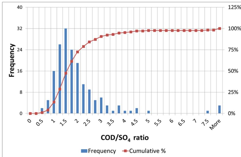
Figure 7 Ratio of primary sewage sludge (measured as COD) to reduce a unit mass of sulphate
