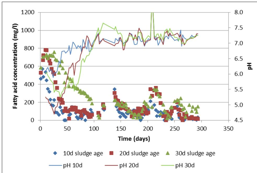
Figure 27 Batch reactor results of VFA at 25°C
