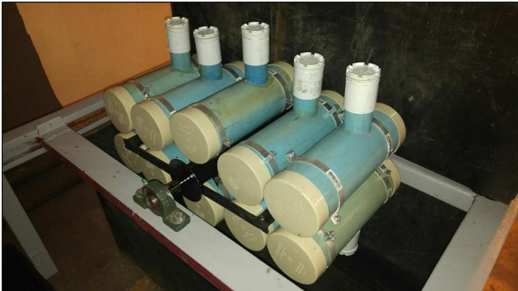
Figure 9 One of three banks with ten containers mounted on a horizontal shaft
