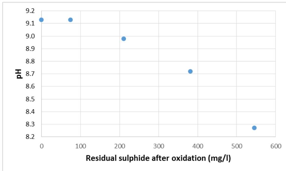
Figure 40 Increase of pH as a result of alkalinity produced during sulphide oxidation
