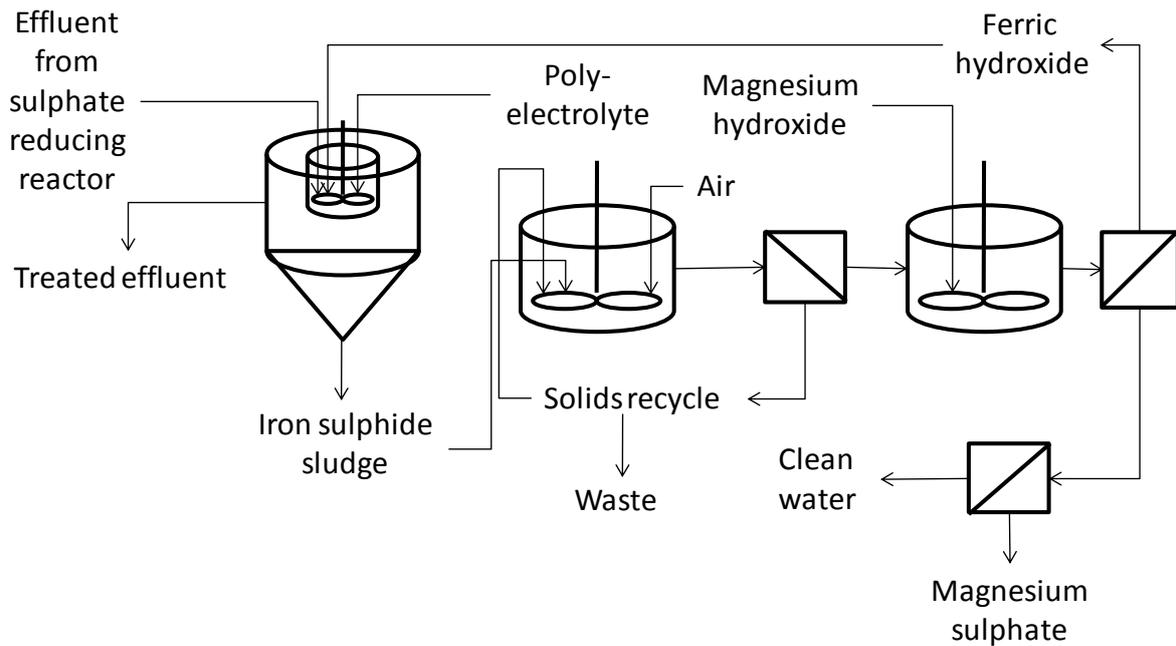
Figure 45 Proposed sulphide removal process
