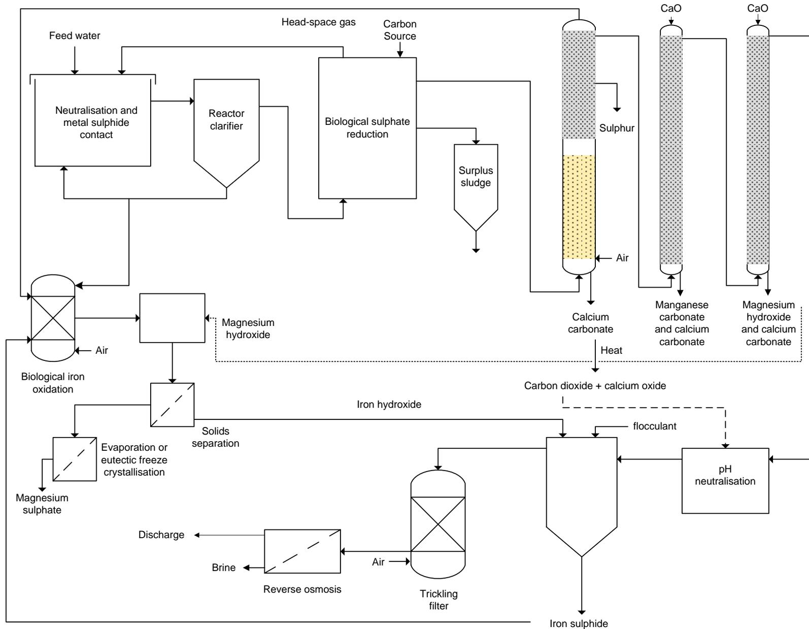
Figure 51 Schematic process layout of proposed demonstration plant
