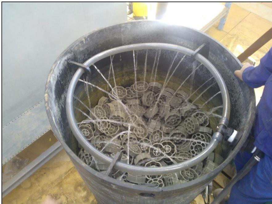
Figure 17 Distribution of recycled ferrous sulphate solution on top of the rosettes
