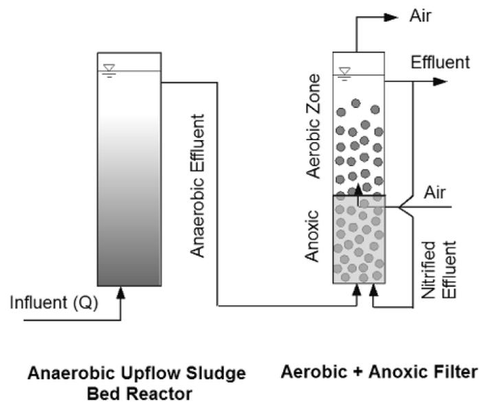
Figure 3 A schematic diagram of the experimental setup of the sulphate reduction, autotrophic denitrification and nitrification integrated (SANI) system (Van den Brand et al., 2013)
