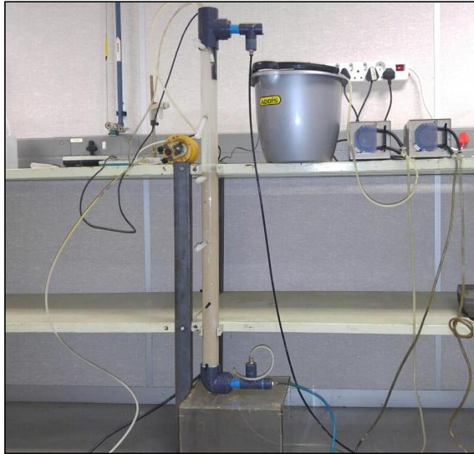
Figure 18 Fluidised bed reactor for precipitation of calcium carbonate pellets
