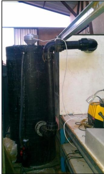
Figure 16 Biological iron oxidation reactor
