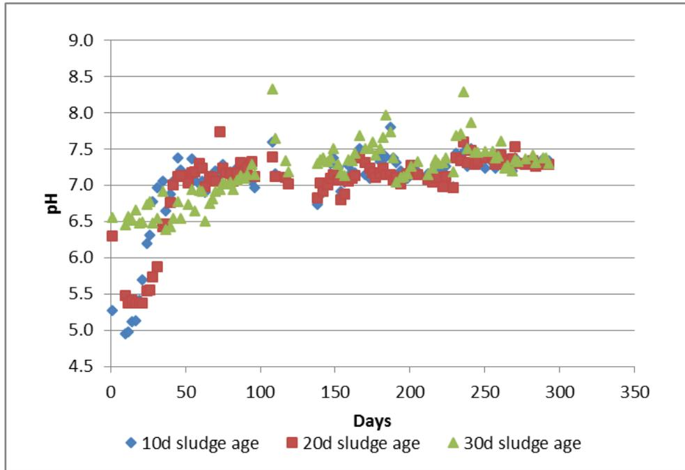
Figure 28 Batch reactor pH at 25°C
