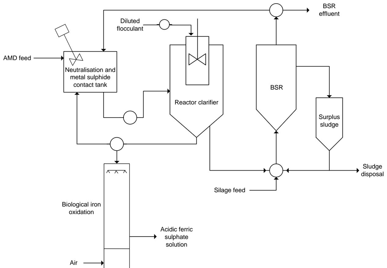
Figure 36 Schematic diagram to illustrate the acid neutralization and FeS precipitation process
