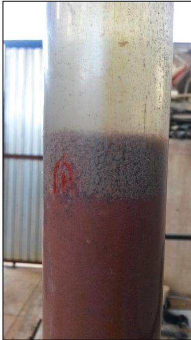
Figure 41 Picture illustrating accumulation of biosulphur particles on top of fluidised bed reactor
