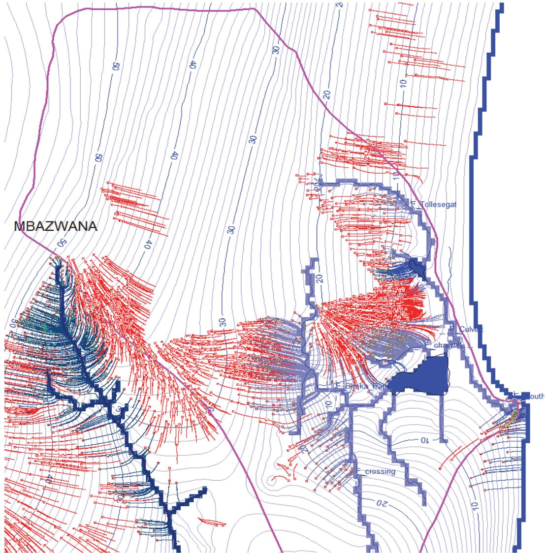
Figure 97. The simulate particle tracks for hypothetical contaminants released into the groundwater at all the dwelling sites in the Mgobezeleni and surrounding catchment.
