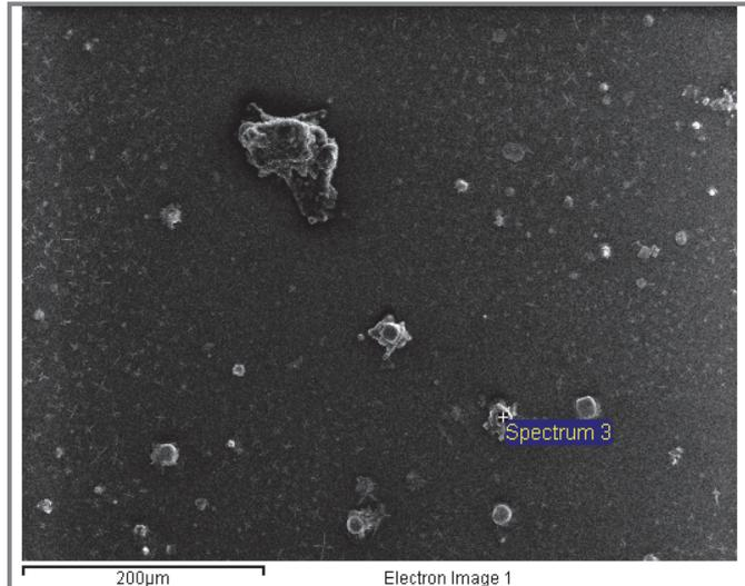
**Figure 52.** Scanning electron microscope image of black (peat) fragments collected from the bottom of the estuary (Note scale) (Photo: S Naidu, UKZN).
