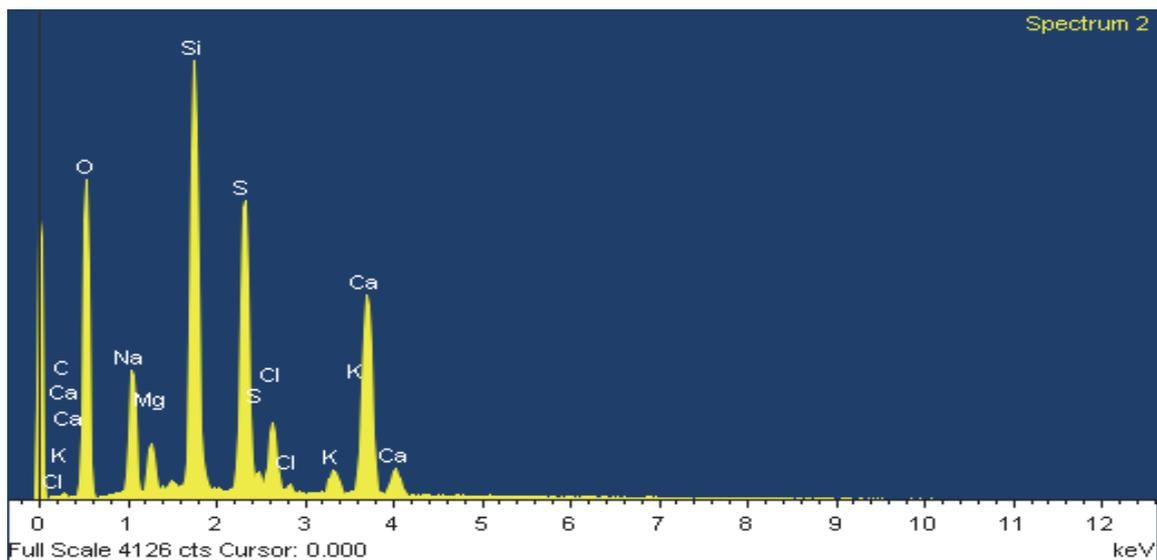
**Figure 53.** EDX elemental analysis report of the estuary particle (Site 3 Spot 2) from Figure 52 above.
