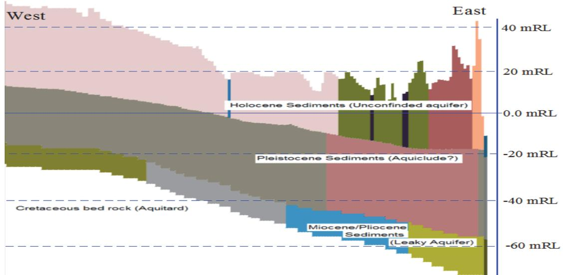
Figure 75. A vertical transect through the model from west to east illustrating the three layers comprising different HSUs.
