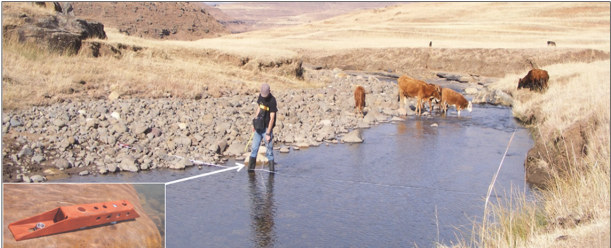
Figure 3.15 Hydraulic site VT1 and underwater image (bottom left) of the level sensor within a metal casing bolted to a large boulder.
