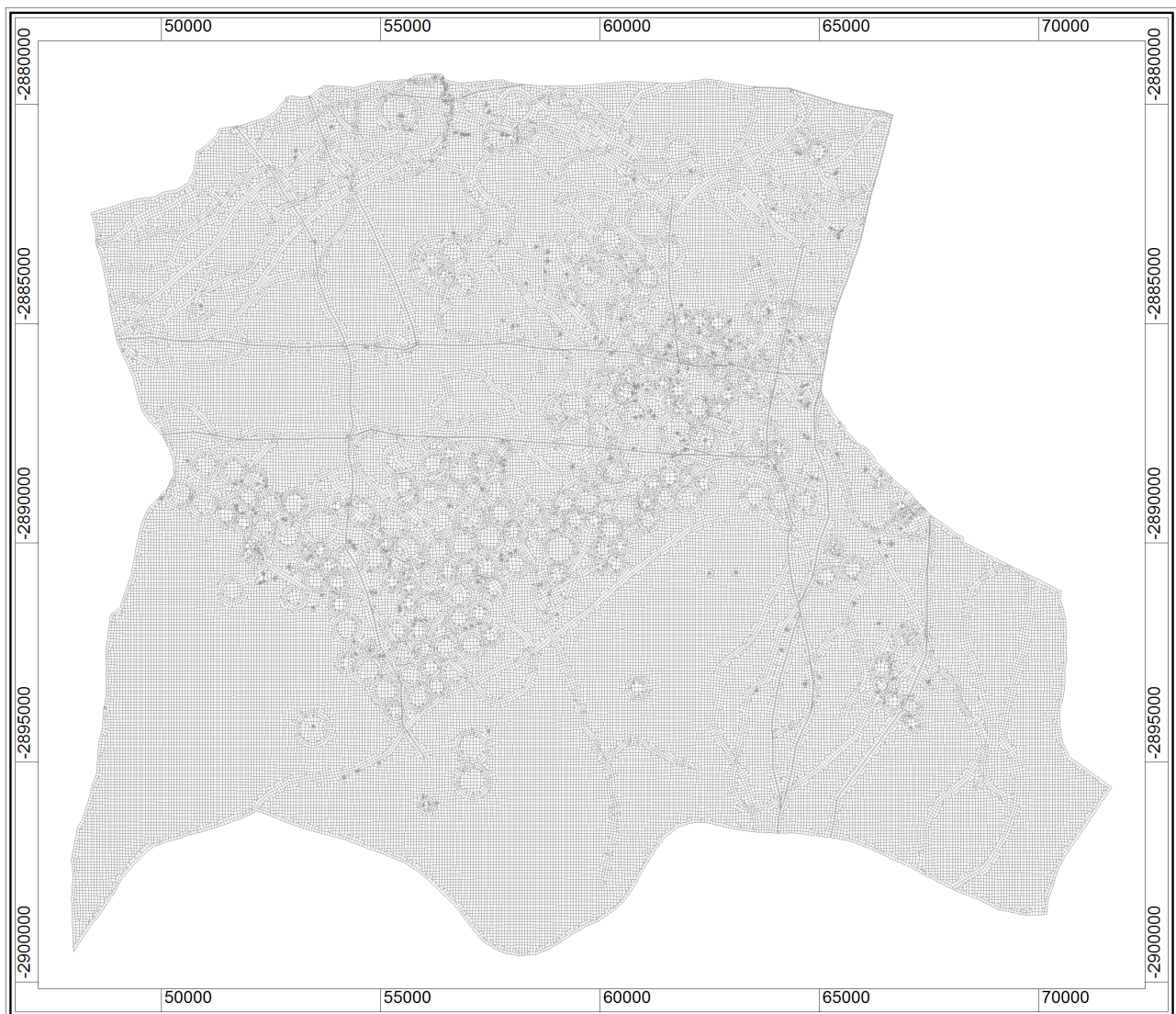
Figure 8-10 Finite-element mesh of the Steenkoppies groundwater model
