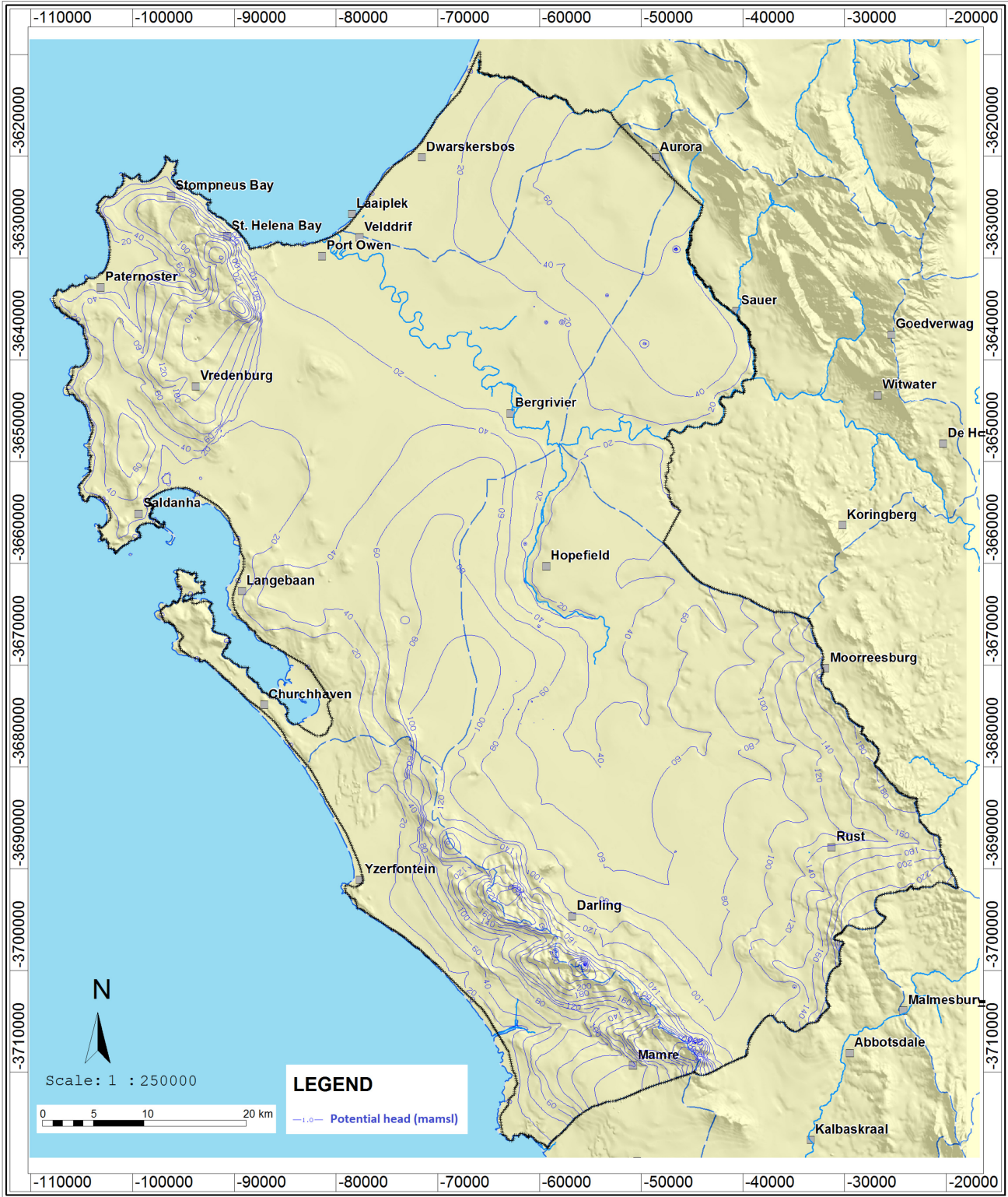
Figure 7-31 Simulated groundwater contours (with simplified location map) for model node layer 1 across the model domain
