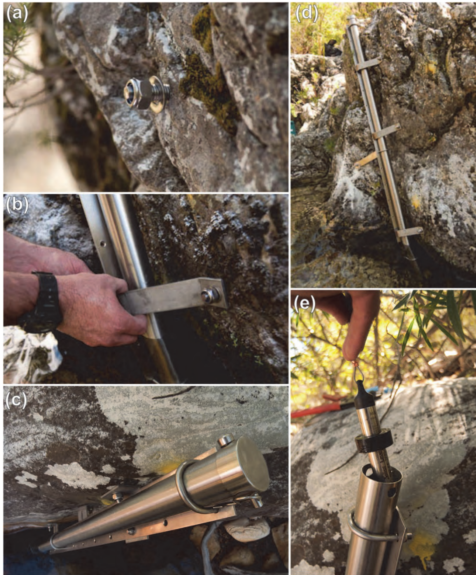
Figure 3.4 (a) Rawlbolt insertion into bedrock , (b) Fitting the mounting bracket to the mounting plate, (c) cap on the stilling well held in place with a bolt and clinch pin (d) installed stilling well with mounting brackets, (e) inserting the Solinst water level logger.
