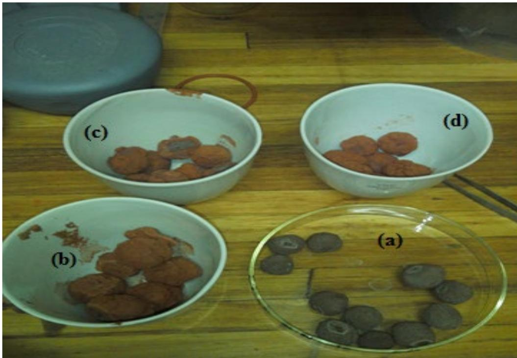
Figure 6.1. Iron(III) oxide modified bentonite-red/black clay soil composite ceramic pellets before (a) and after calcination (b, c and d)
