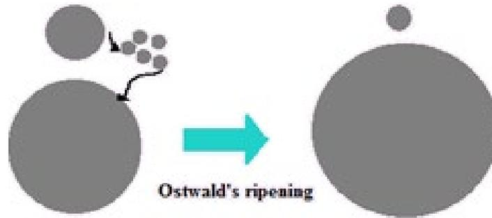
**Figure 4-13: Ostwald's ripening illustrating the aggregated nanocrystals, where the larger cluster grows larger in size, but decreases in number, and the smaller cluster decreases in size and the number of particles**
