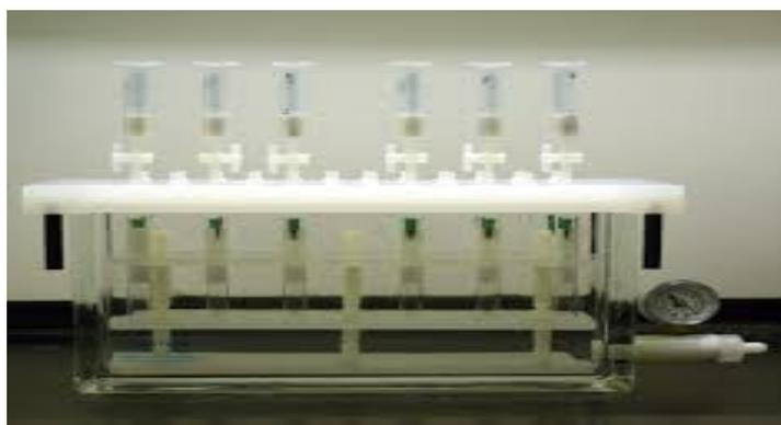
Figure 10-1: SPE column apparatus
