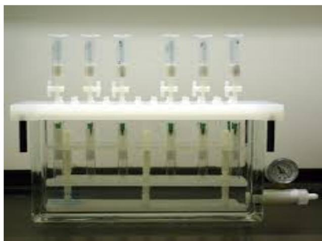
Figure 7-2: A typical experimental set up for  $\text{Pb}^{2+}$  and  $\text{Cd}^{2+}$  adsorption and regeneration (Jeff Dahn, 2011)
