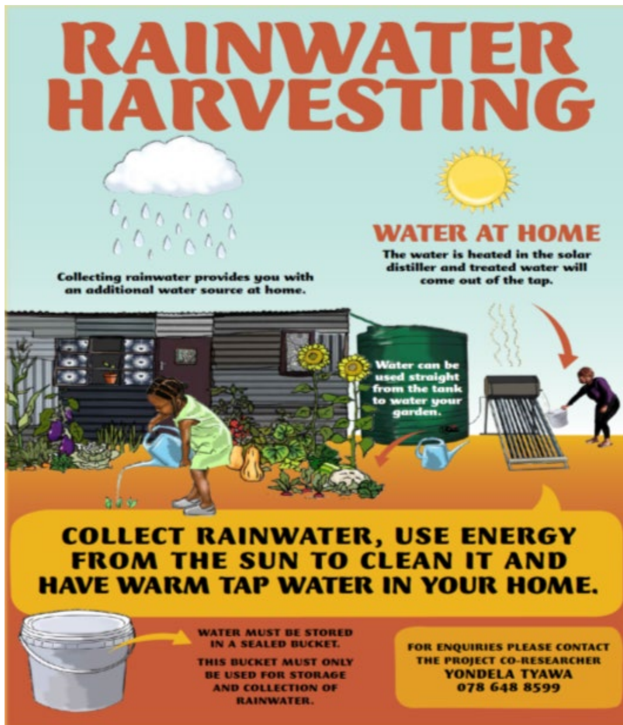
Figure 4.5. The first page of the final English pamphlet guide illustrating the principle of the rainwater harvesting treatment system and its benefits. Information regarding the storage of the rainwater and the contact details of the co-researcher are also provided.
