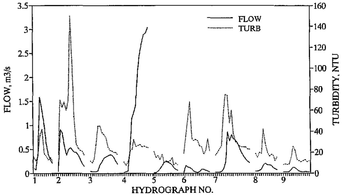
Figure 42: W1H031: Variation in turbidity levels with flow
