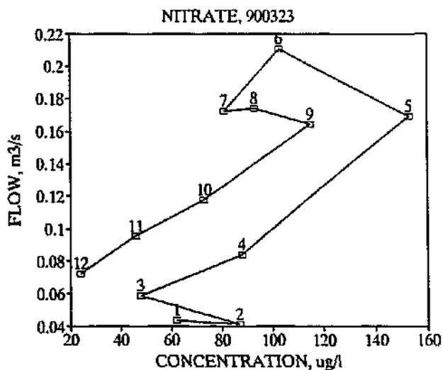
Figure 54: W1H031: Changes in nitrate concentrations during hydrographs
