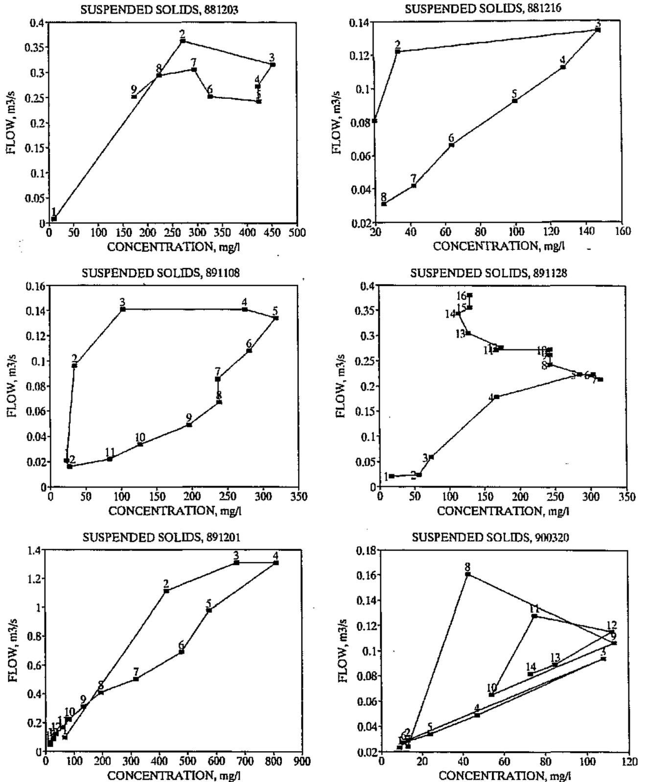
Figure 28: U2H018: Changes in suspended solids concentrations during hydrographs
