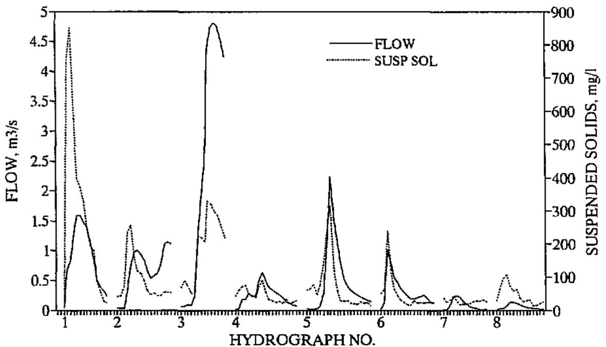
Figure 41: W1H016: Variation in turbidity levels with flow
