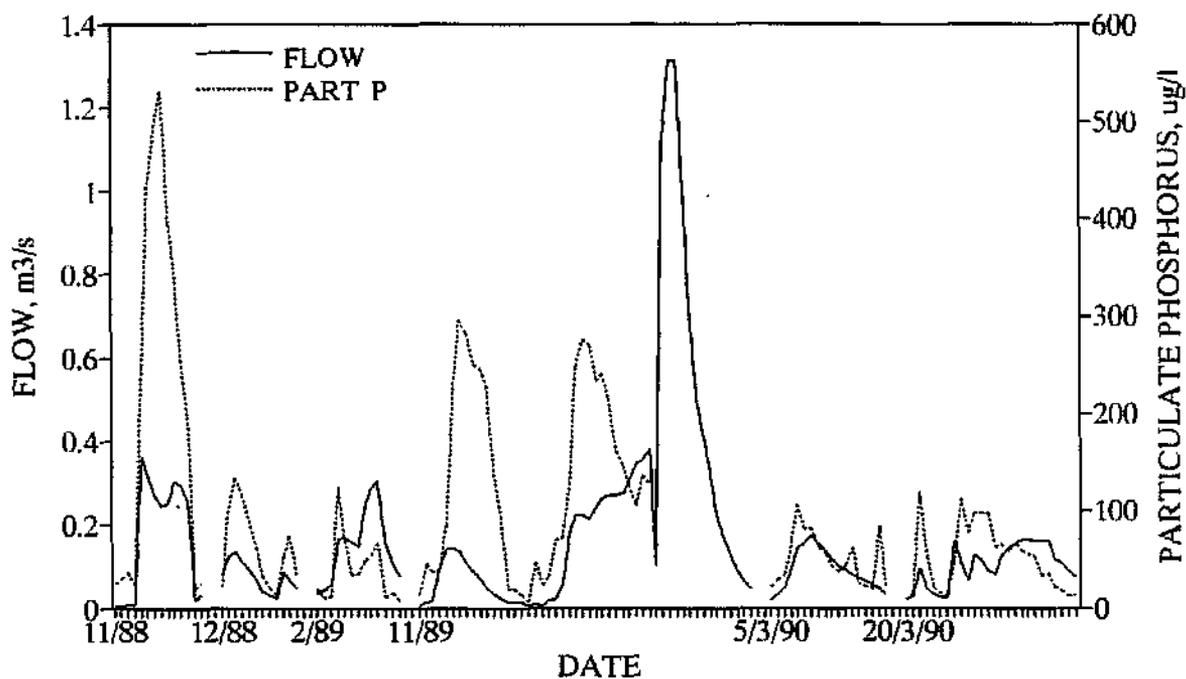
Figure 24: U2H018: Variation in particulate P concs. with flow
