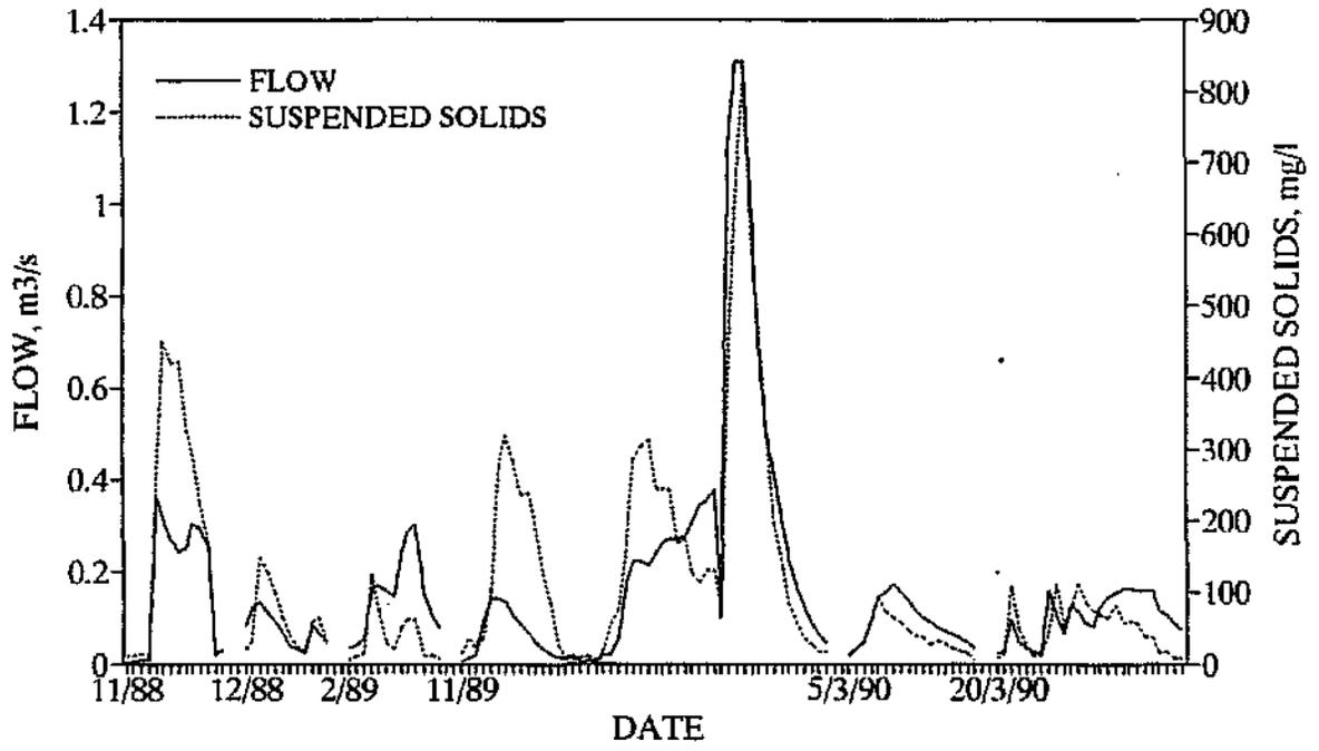
Figure 16: U2H018: Variation in suspended solids concs. with flow
