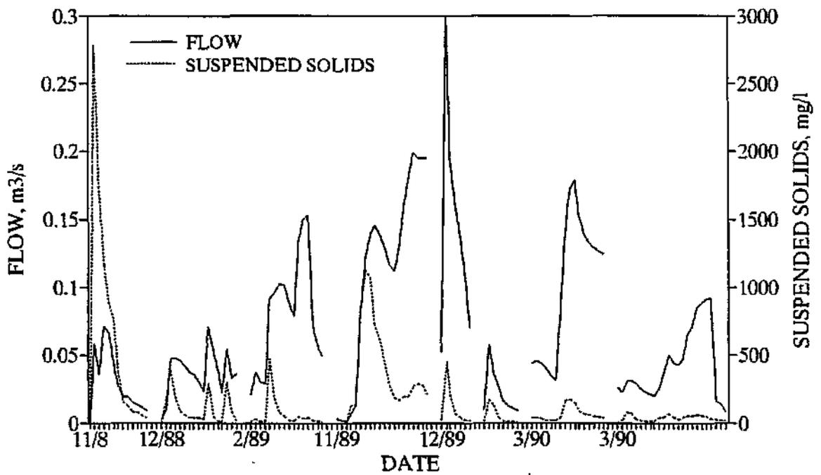
Figure 17: U2H016: Variation in turbidity levels with flow
