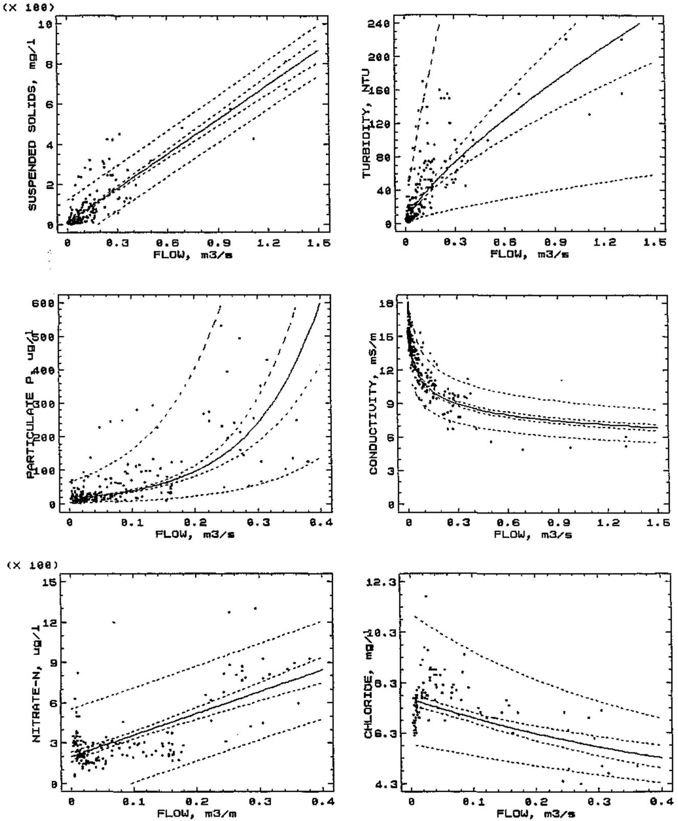
Figure 34: U2H018: Best fit regression curves for variables on flow
