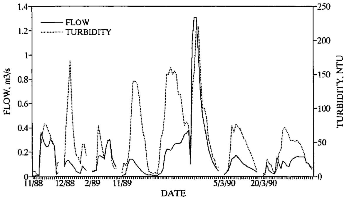
Figure 18: U2H018: Variation in turbidity levels with flow
