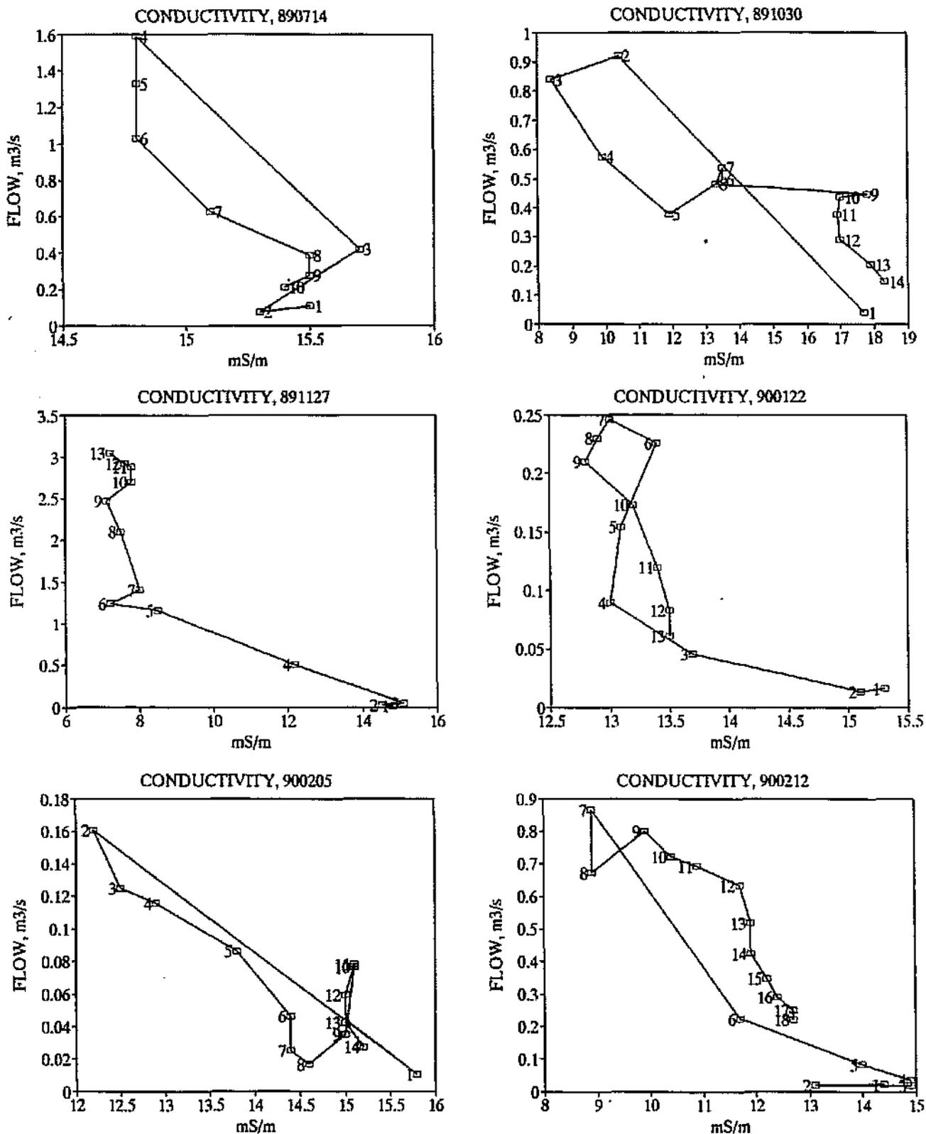
Figure 52: W1H031: Changes in conductivity levels during hydrographs
