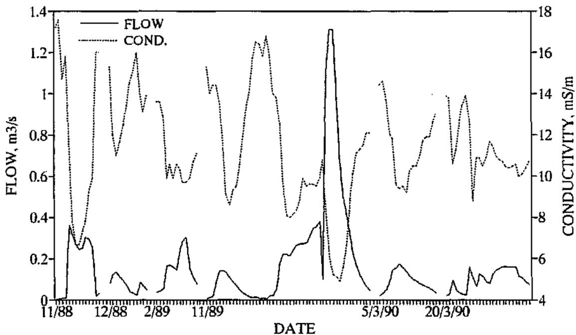
Figure 20: U2H018: Variation in conductivity levels with flow
