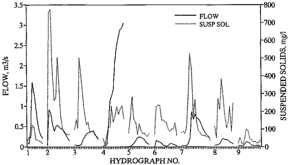
Figure 40: W1H031 Variation in suspended solids concs. with flow
