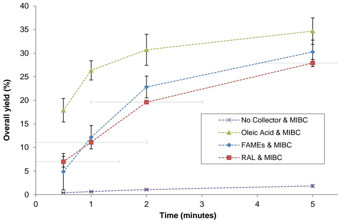
Figure 14: Overall yield achieved in the concentrate as a function of time for Waterberg coal waste tailings flotation using RAL and algal derived FAMEs at a concentration of 2.79 kg/ton of coal waste
