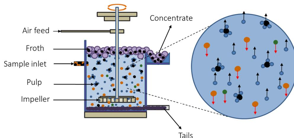
Figure 2: Schematic of a typical flotation setup
