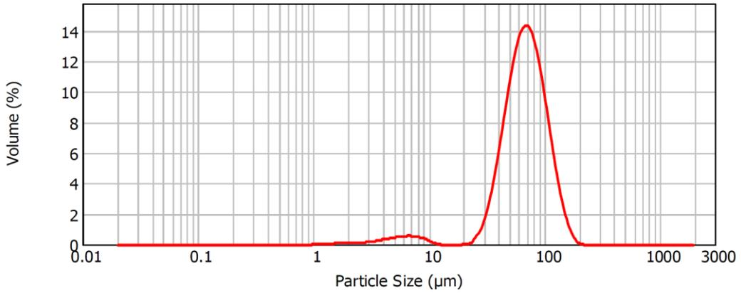
Figure 34: Particle size distribution for quartz sample, generated through a Malvern analysis
