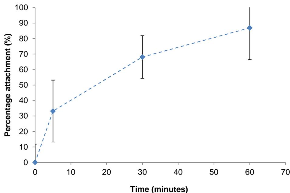
Figure 18: Attachment of a mixed mesophilic culture to pyrite over time. Error bars show a standard deviation variation across triplicate repeats.
