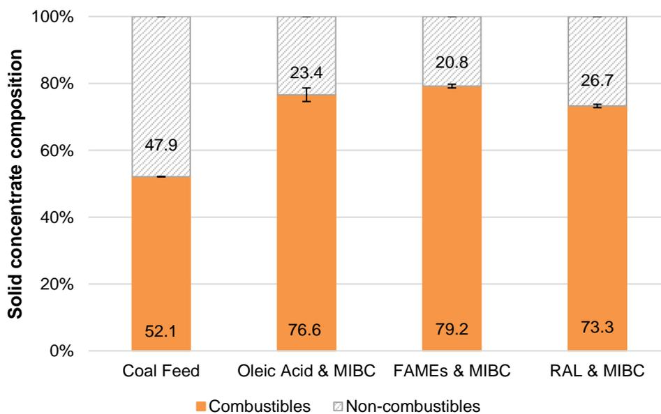
Figure 15: Composition of final cumulative solid concentrates after flotation of Waterberg coal waste tailings using RAL and algal derived FAMEs at a concentration of 2.79 kg/ton of coal waste
