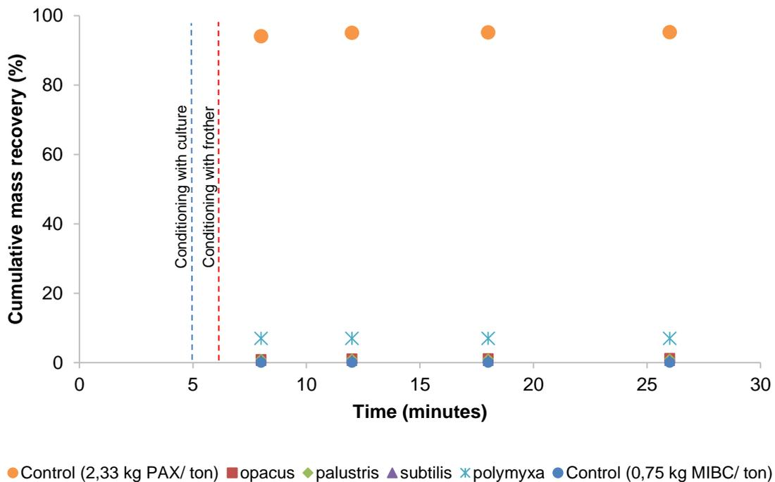
Figure 24: Cumulative mass recovery of pyrite after floating with the *R. opacus*, *R. palustris*, *B. subtilis* and *P. polymyxa* culture at pH 4 with a cell concentration of  $4.2 \times 10^9$  cells/g for all cultures excepting  $2.45 \times 10^9$  cells/g for *P. polymyxa*
