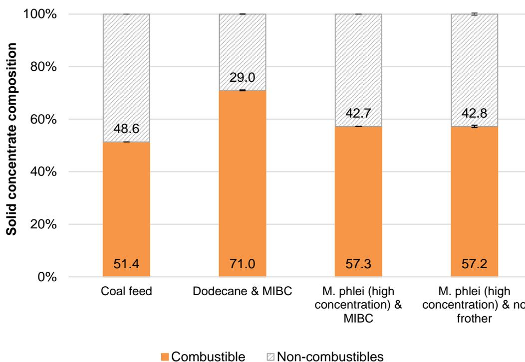
Figure 12: Composition of final cumulative solid concentrates after flotation of Witbank coal waste tailings using *M. phlei*
