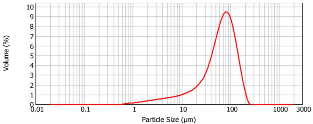
Figure 36: Particle size distribution for Witbank ultrafine coal sample, generated through a Malvern analysis
