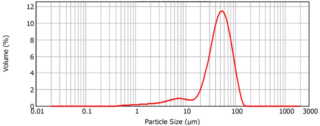
Figure 35: Particle size distribution for pyrite sample, generated through a Malvern analysis
