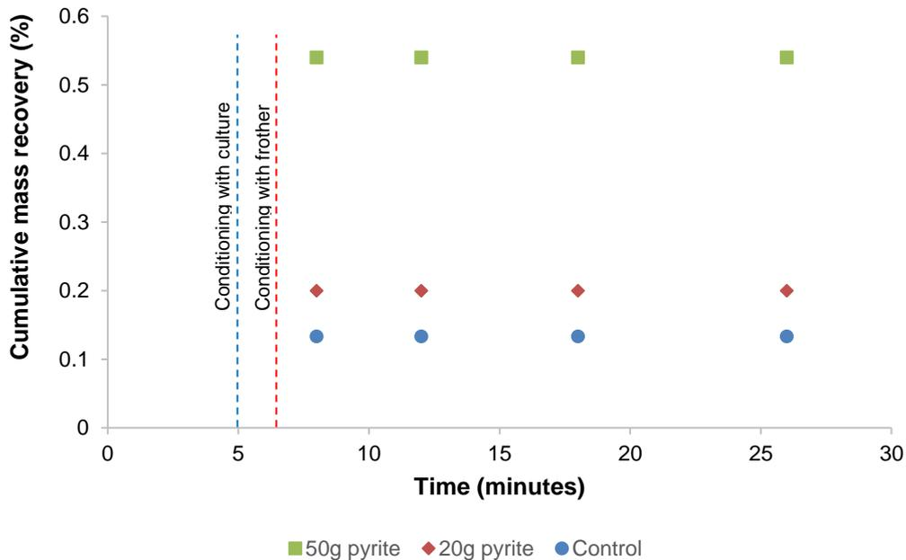
Figure 26: Cumulative mass recovery of pyrite after floating with sulphur oxidizing mixed culture: 50 g of pyrite was treated with a culture containing a cell concentration of  $1 \times 10^9$  cells/g, and 20 g of pyrite was treated with a culture containing a concentration of  $2 \times 10^9$  cells/g
