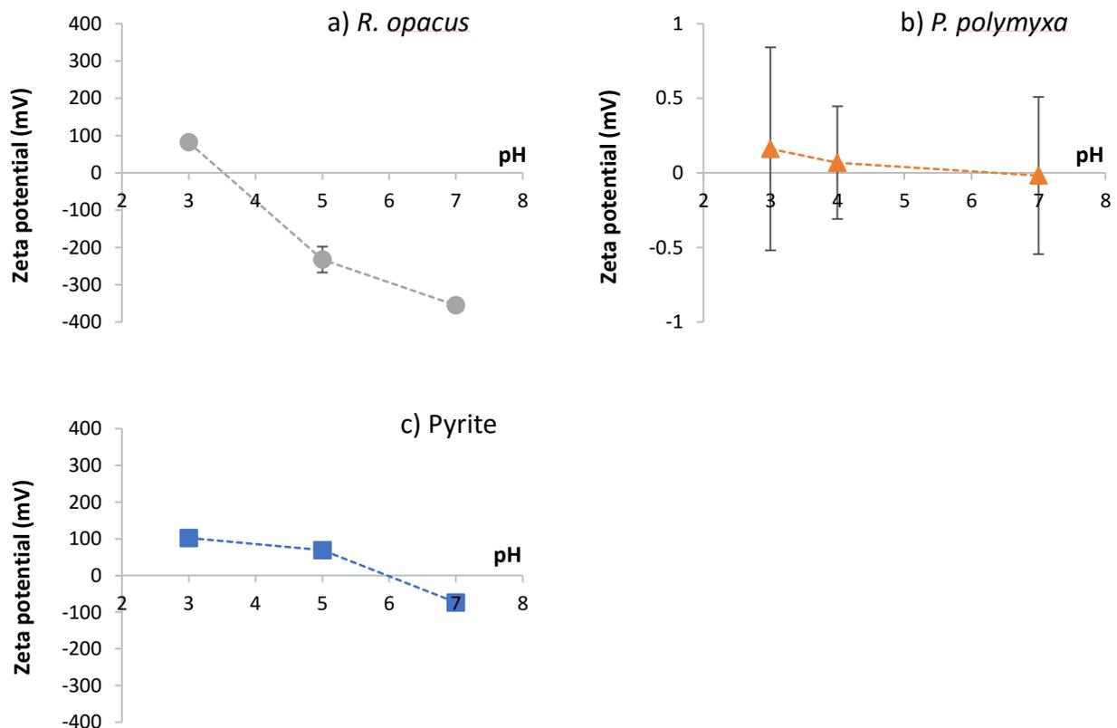
Figure 23: Measured zeta potential as a function of pH for (a) *R. opacus*, (b) *P. polymyxa* and (c) pyrite mineral
