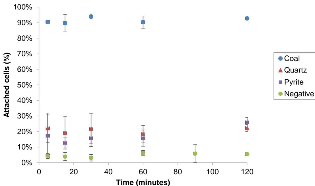
Figure 6: Attachment of *M. phlei* to coal, quartz and pyrite in a 1 g solid per 100 ml suspension containing a cell concentration of  $2 \times 10^7$  cells/ml
