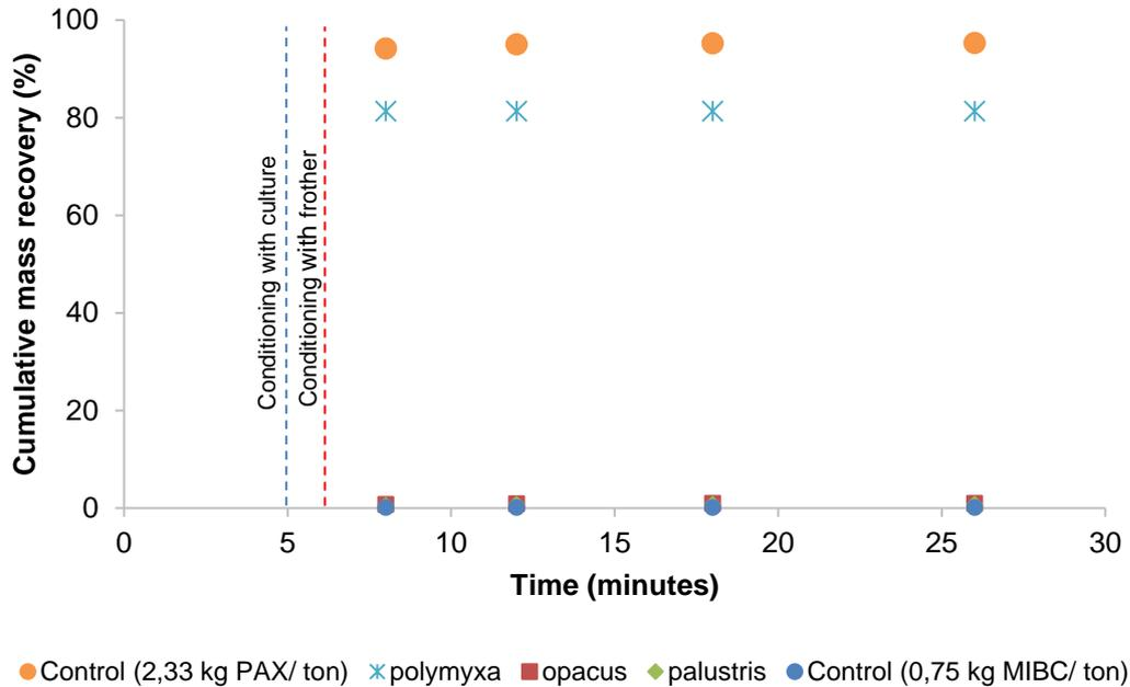
Figure 25: Cumulative mass recovery of pyrite after floating with the *R. opacus*, *R. palustris*, *B. subtilis* and *P. polymyxa* culture at pH 7 with a cell concentration of  $4.2 \times 10^9$  cells/g for all cultures excepting  $2.45 \times 10^9$  cells/g for *P. polymyxa*
