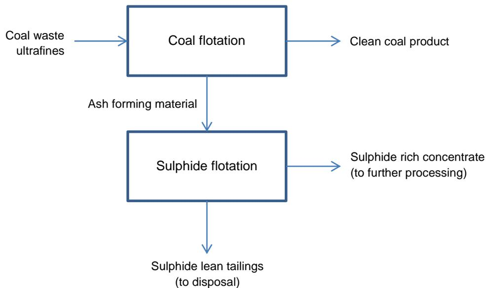
Figure 4: Two stage ultrafine coal waste desulphurization process (adapted from Kazadi Mbamba et al. (2012))
