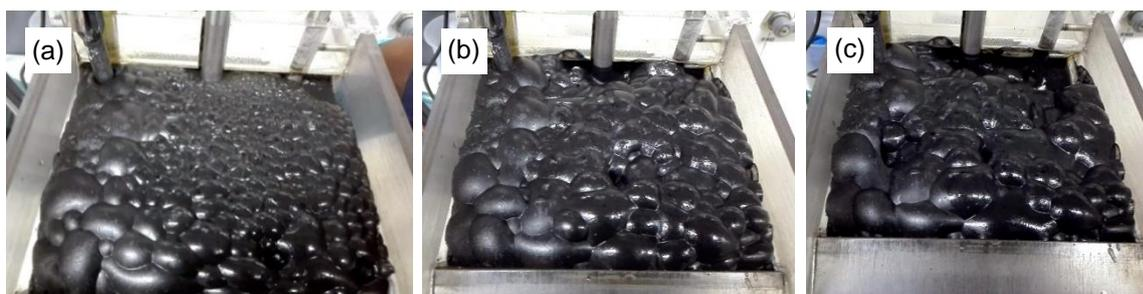
Figure 16: Froth produced in a float using only RAL (a) 2 seconds, (b) 7 seconds and (c) 15 seconds after air on
