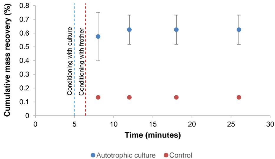
Figure 27: Cumulative mass recovery of pyrite after floating with autotrophic SCN<sup>-</sup> degrading mixed culture; 20 g of pyrite was treated with a culture containing a concentration of  $2 \times 10^9$  cells/g. Error bars show a standard deviation variation across duplicate repeats.
