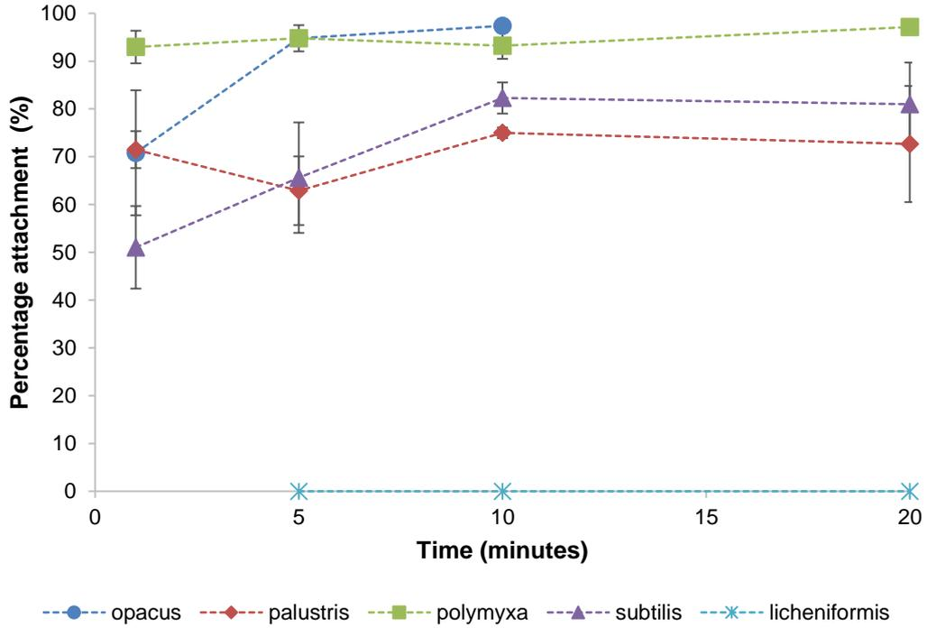
Figure 21: Percentage attachment of *R. opacus*, *R. palustris*, *P. polymyxa*, *B. subtilis* and *B. licheniformis* cells onto pyrite in a 1 g solid per 100 ml suspension containing a cell concentration of  $1 \times 10^7$  cells/ml at pH 7. Error bars show a standard deviation variation across triplicate repeats.
