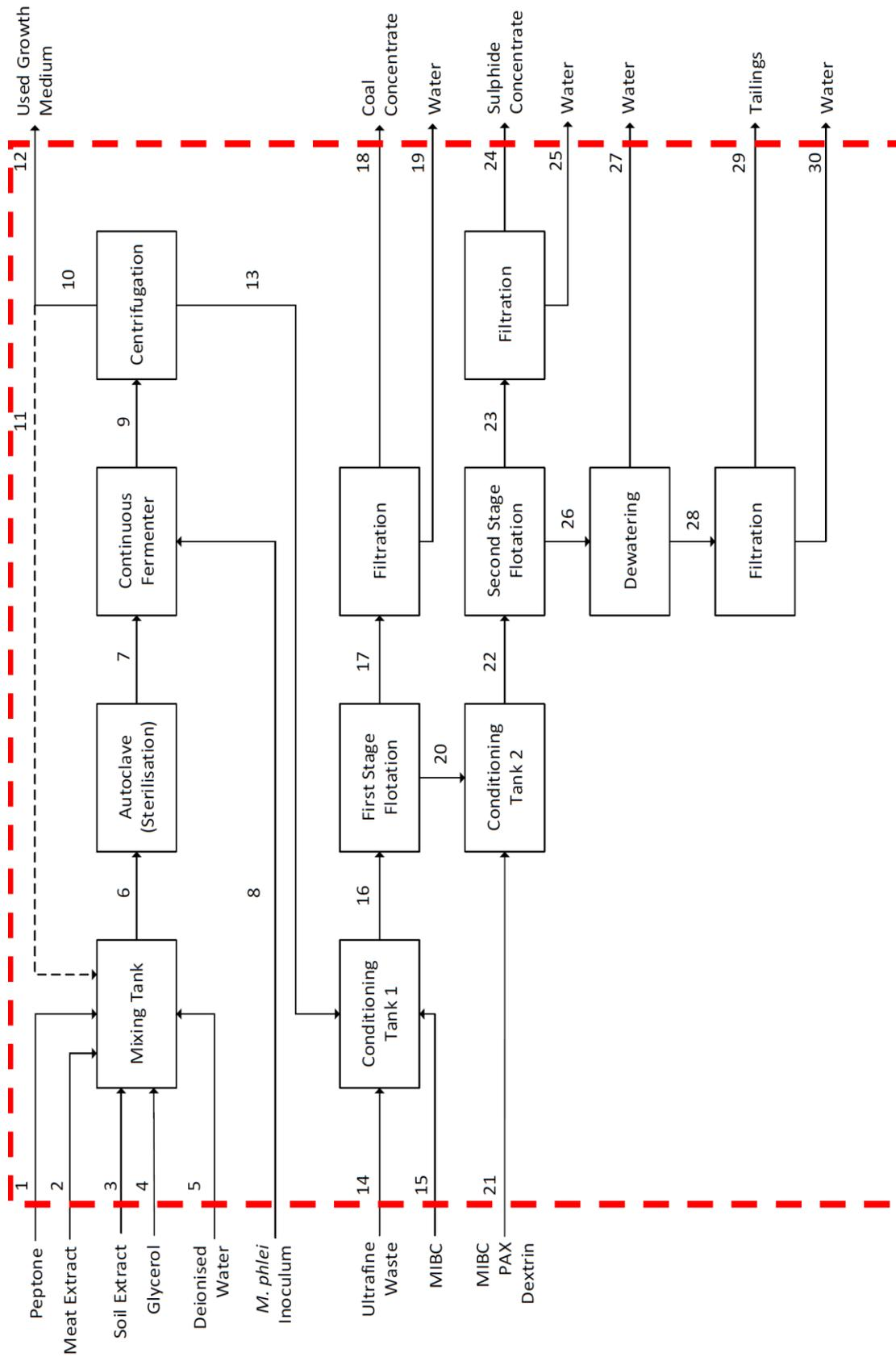
Figure 28: Bioflotation process flowsheet for *M. phlei* usage in the first-stage of the two-stage process
