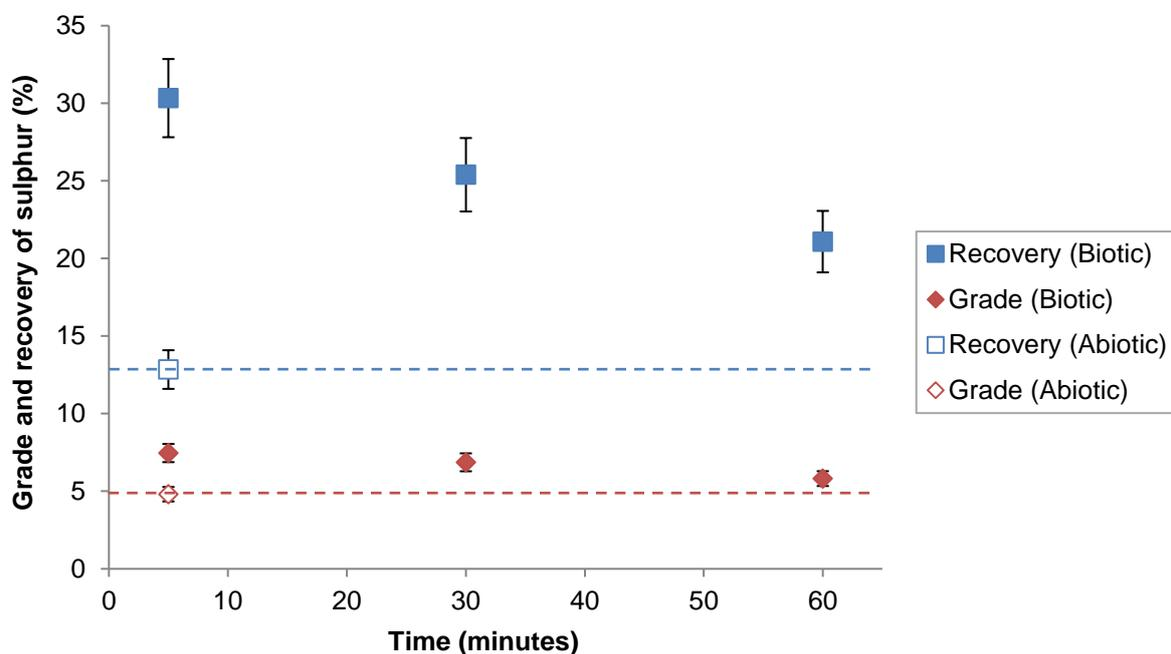
Figure 20: Grade and recovery of sulphur in the concentrate with increased contact time, using  $1 \times 10^8$  cells/g pyrite. Error bars show a standard deviation variation across two repeats.
