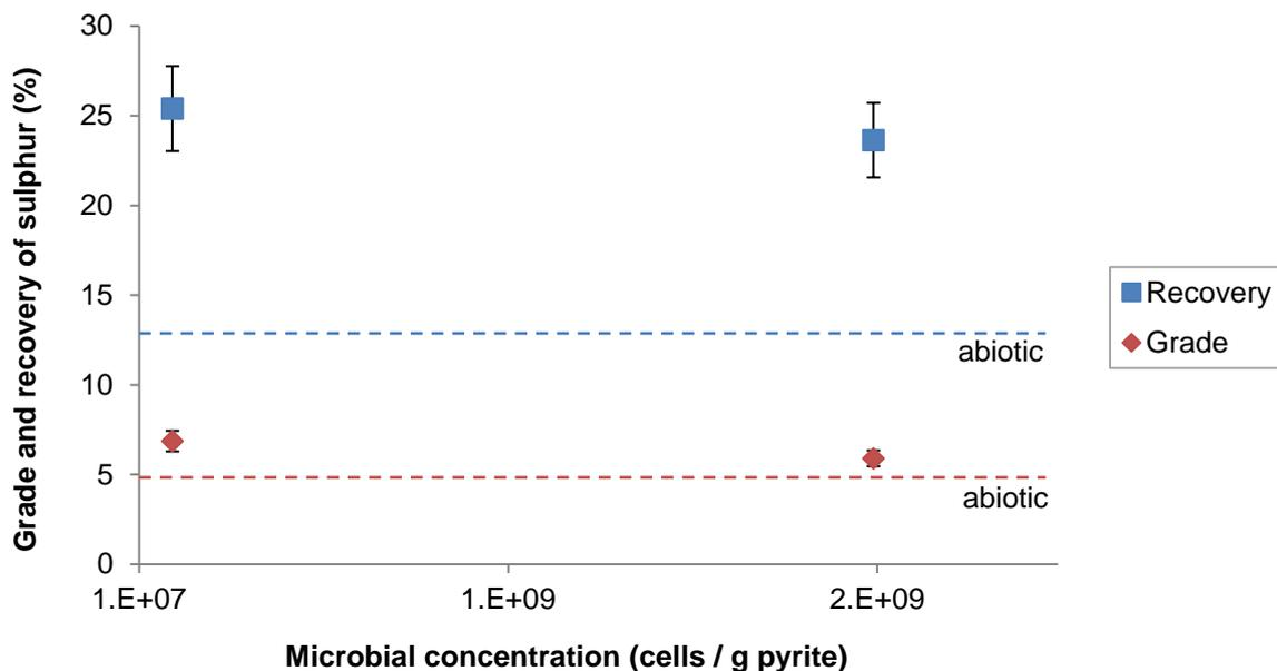
Figure 19: Grade and recovery of sulphur in the concentrate achieved using low and high microbial concentrations, following a 30 minute contacting time. Error bars show a standard deviation variation across two repeats. The dashed lines show the baseline for the negative control.
