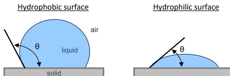
Figure 3: Hydrophobic vs. hydrophilic contact angles
