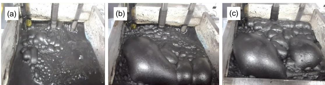
Figure 17: Froth produced in float using only FAME (a) 2 seconds, (b) 7 seconds and (c) 15 seconds after air on
