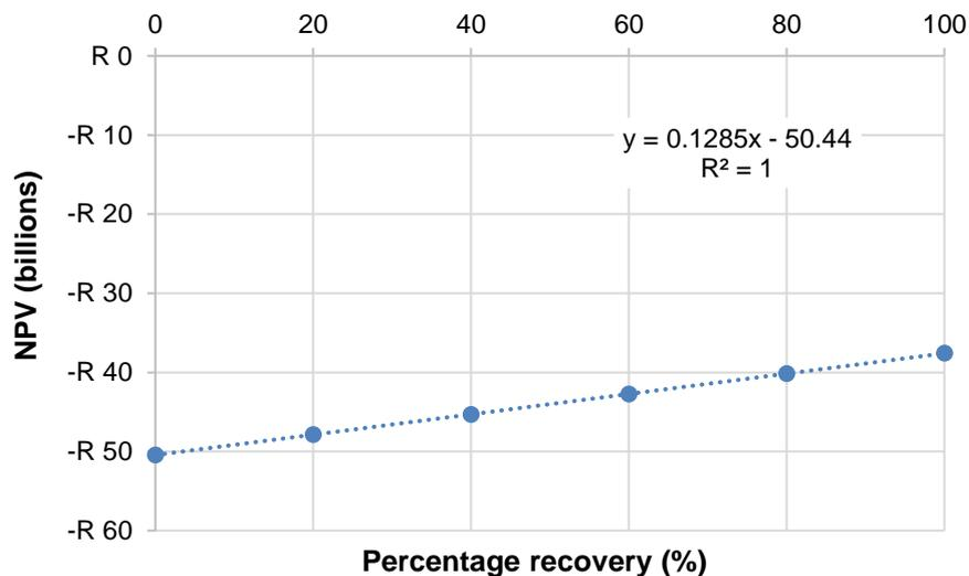
Figure 32: Analysis of the sensitivity of the NPV to coal recovery
