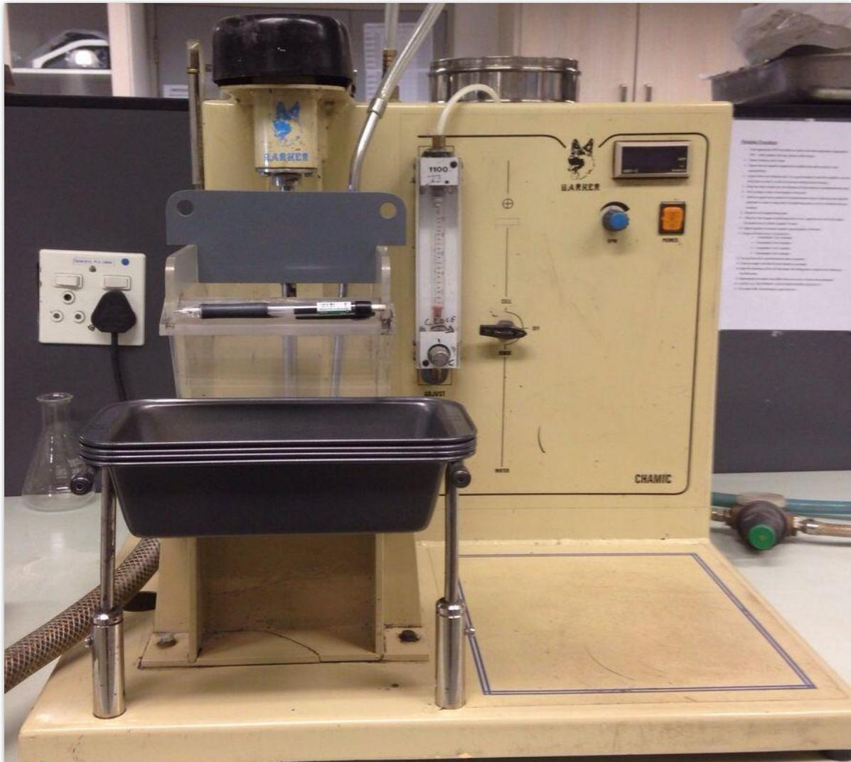
Figure 5: Leeds 3 litre bottom-driven and sub-aeration laboratory scale batch flotation cell
