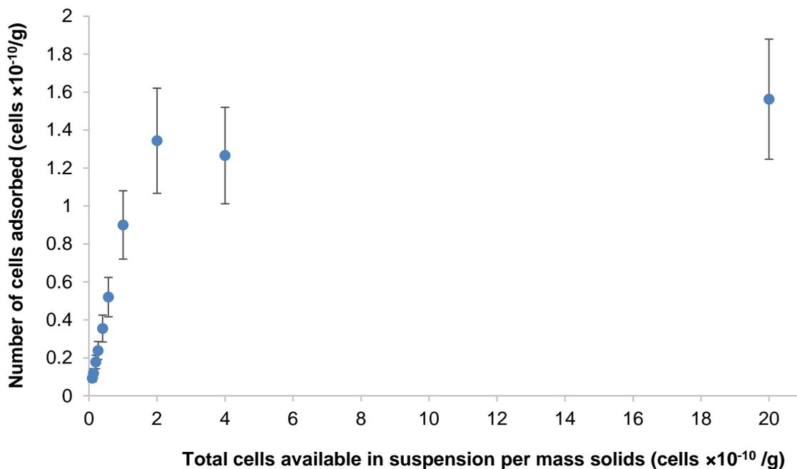
Figure 8: *M. phlei* adhesion to coal adsorption isotherm
