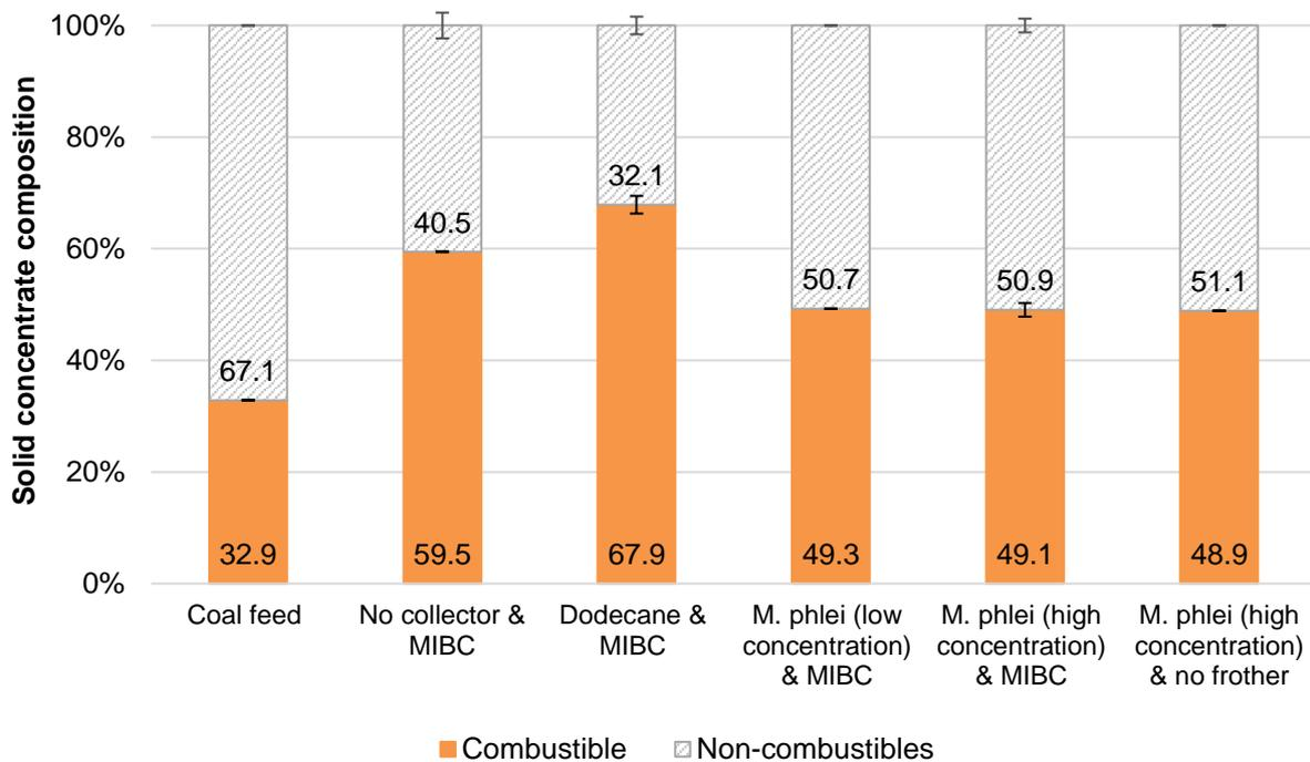
Figure 10: Composition of final cumulative solid concentrates after flotation of the constructed coal waste tailings sample
