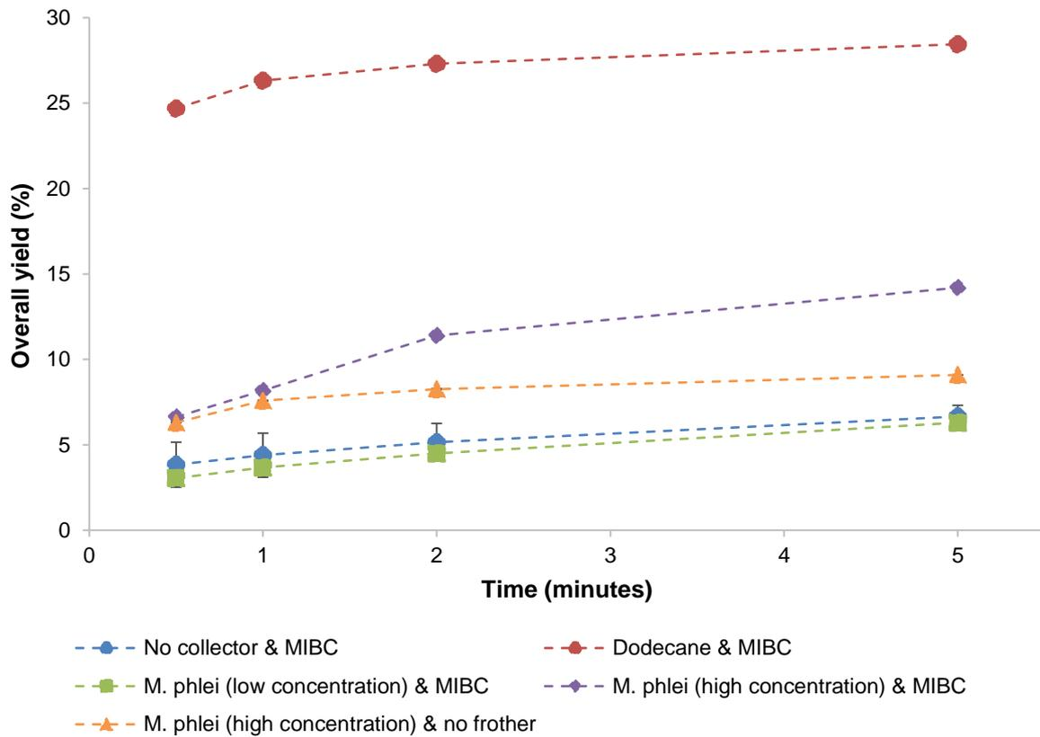
Figure 9: Overall yield achieved in the concentrate as a function of time for the constructed coal sample
