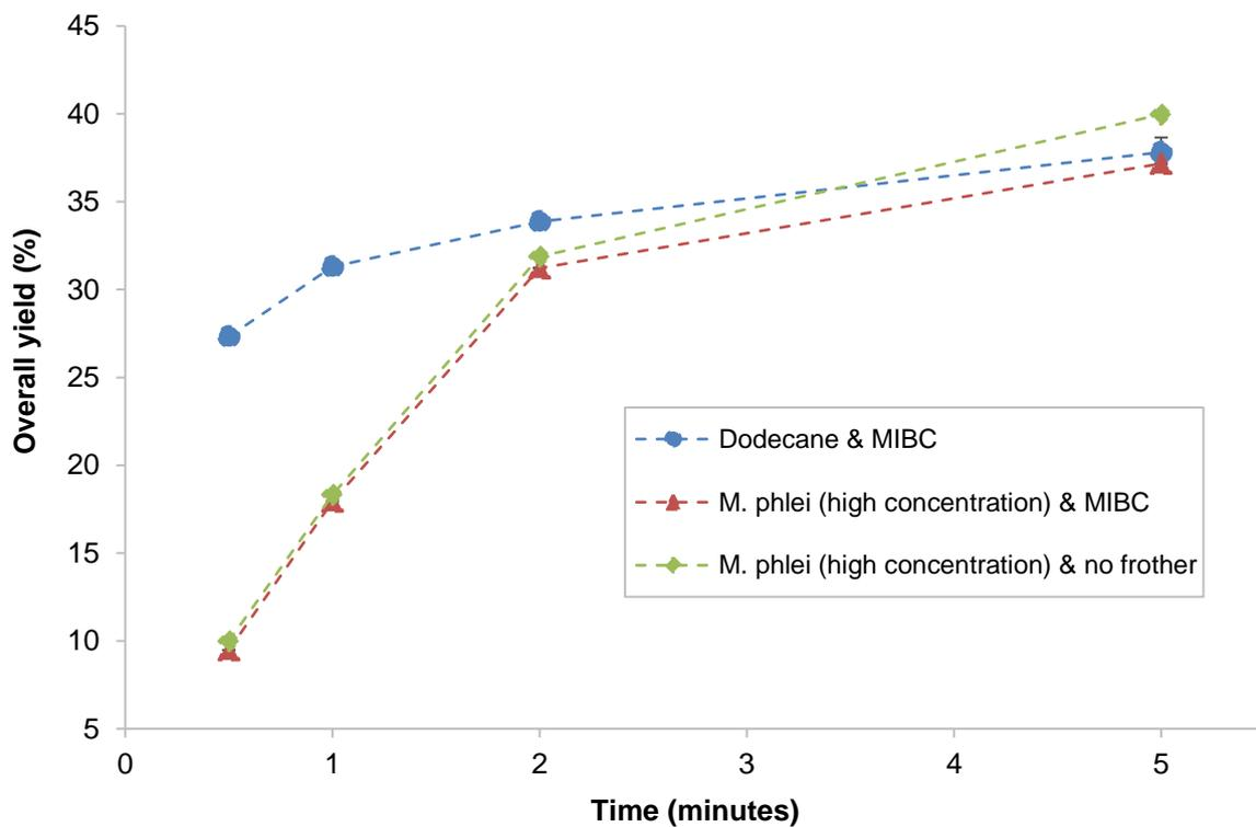
Figure 11: Overall yield achieved in the concentrate as a function of time for Witbank coal waste tailings flotation using *M. phlei*
