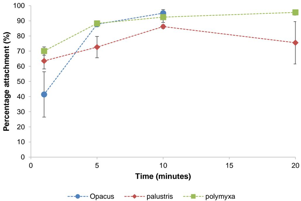
Figure 22: Percentage attachment of *R. opacus*, *R. palustris* and *P. polymyxa* cells onto pyrite in a 1 g solid per 100 ml suspension containing a cell concentration of  $1 \times 10^7$  cells/ml at pH 4. Error bars show a standard deviation variation across triplicate repeats.
