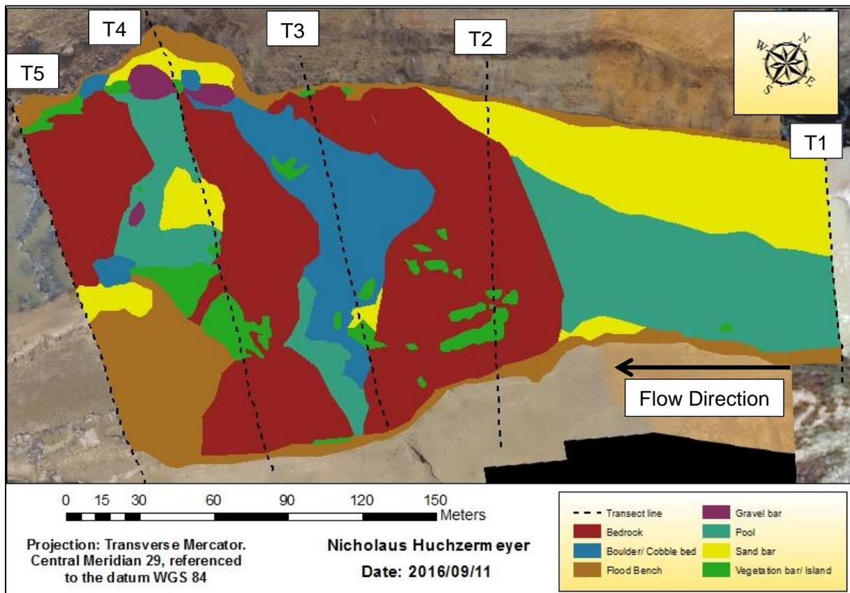
**Figure 6-18: Channel features at a large scale for Site 5.**
