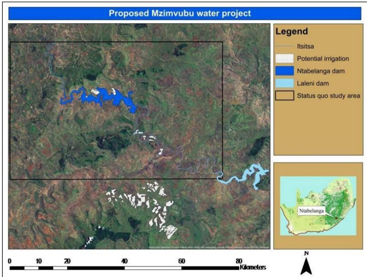
**Figure 2-2: Predicted inundation footprint of Ntabelanga and Laleni dam with proposed irrigation areas.**
