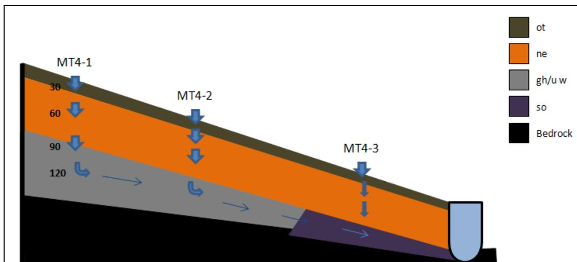
**Figure 5-4: Hydropedological conceptual model of MT4.**
