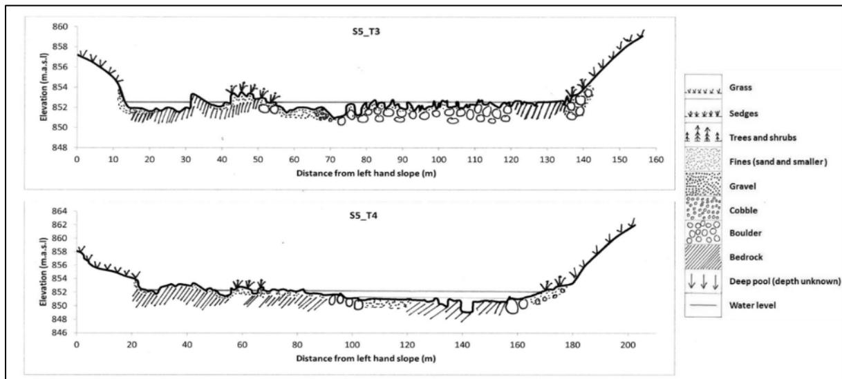
**Figure 6-11: Example of cross-sectional transects with corresponding substrates and geo-habitats, surveyed in July 2015.**
