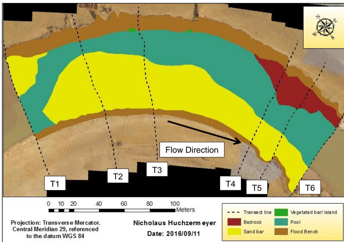
**Figure 6-17: Channel features at a large scale for Site 4.**
