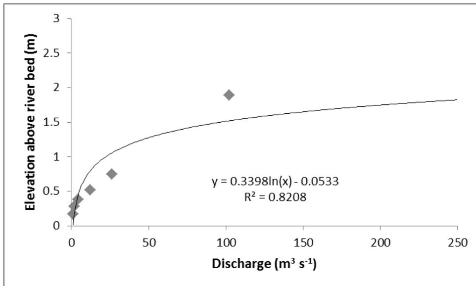
**Figure 6-30: Example of a rating curve for Site 1.**
