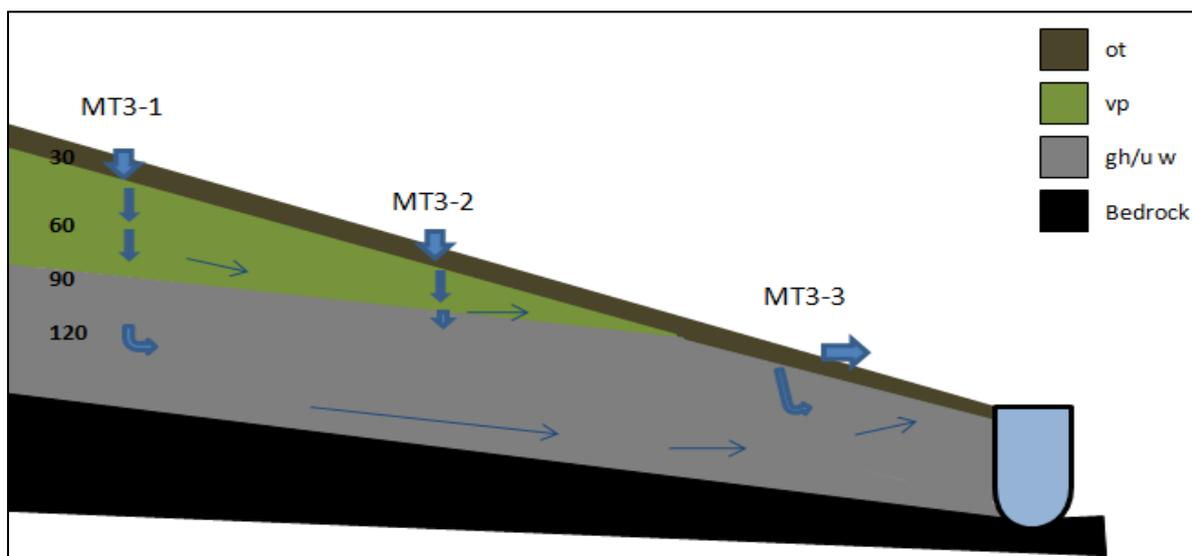
**Figure 5-3: Site 3-Hydropedological conceptual model based on soil morphology.**
