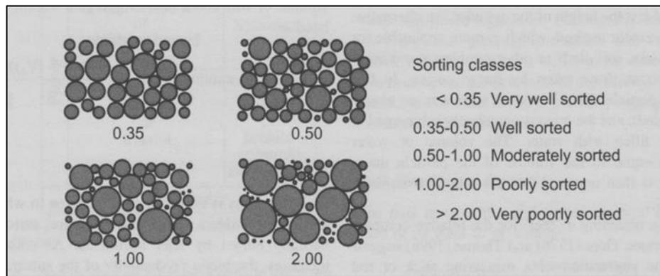
**Figure 3-7: Sorting classes for substrate (Gordon et al., 2004).**
