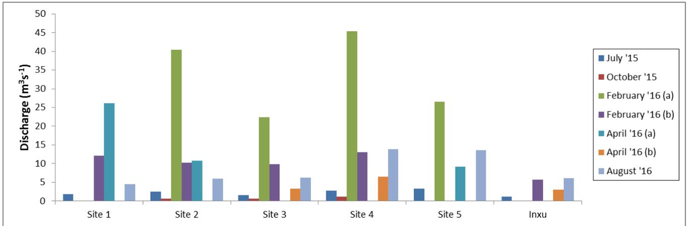
**Figure 6-19: Seasonal variations in measured discharge. a = Rising stage of a flood, b = Receding stage of a flood.**
