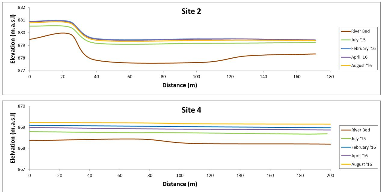
**Figure 6-32: Example of a change in energy slope, with changes in discharge, at sites with different bed gradients.**
