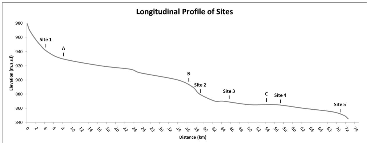
**Figure 6-4: Longitudinal Profile of the selected sites along the Tsitsa River reach ranging from the gorge to below the confluence with the Inxu River. A: End of dam inundation, B: Dam Wall, C: Confluence with Inxu River.**
