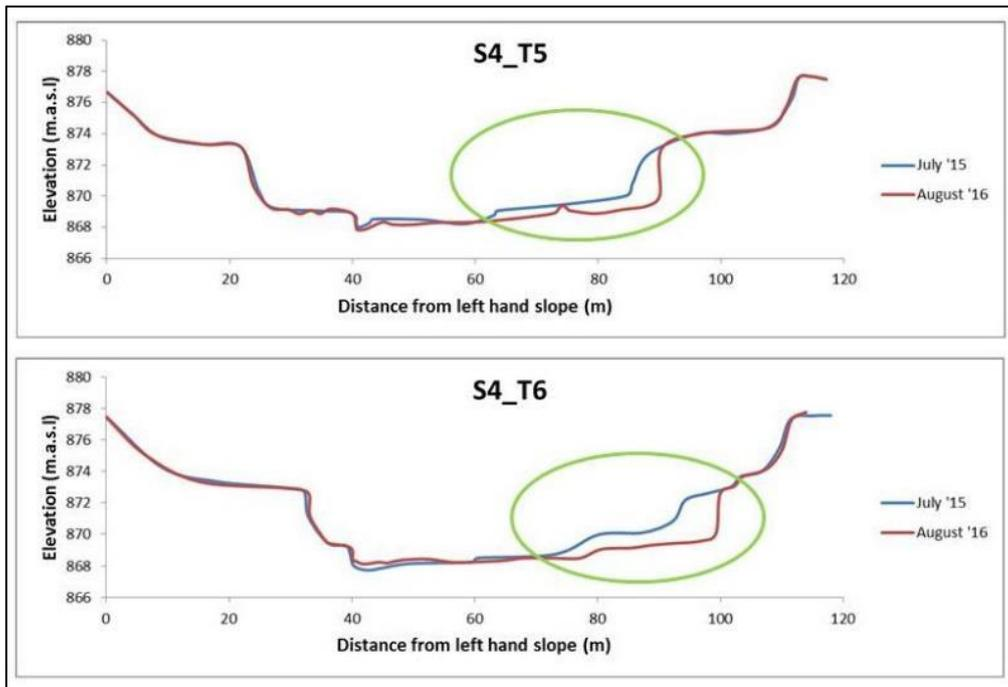
**Figure 6-13: Example of cross-sectional transects that have undergone a seasonal change in topography. In this case changes have occurred due to sand mining at low flows.**
