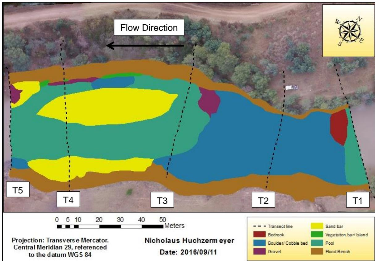
**Figure 6-16: Channel features at a large scale for Site 3.**
