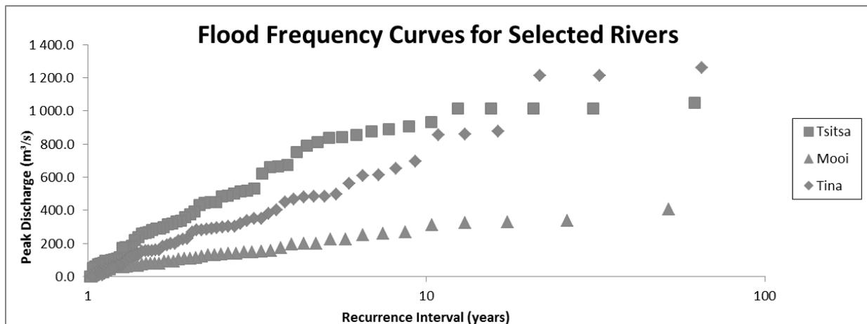
**Figure 6-27: Flood Frequency curves for three rivers in the Mzimvubu catchment.**
