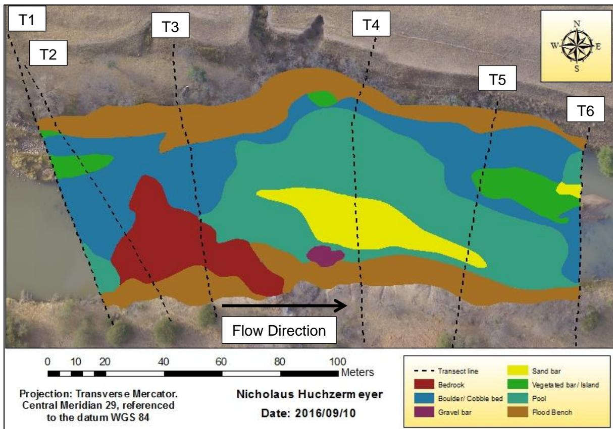
**Figure 6-15: Channel features at a large scale for Site 2.**
