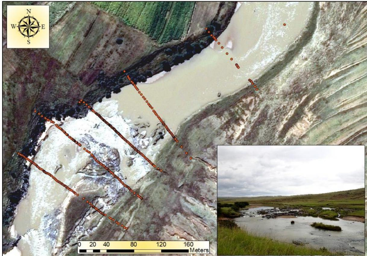
**Figure 3-6: The location of cross-sectional surveys for Site 5, below the confluence with the Inxu, to monitor increased embeddedness of coarse substrate and channel narrowing and or reduction in depth.**
