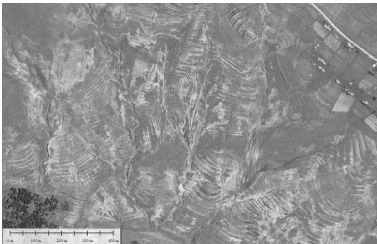
**Figure 2-20: Example of gully erosion commencing on old cultivated lands in land type Ab.**
