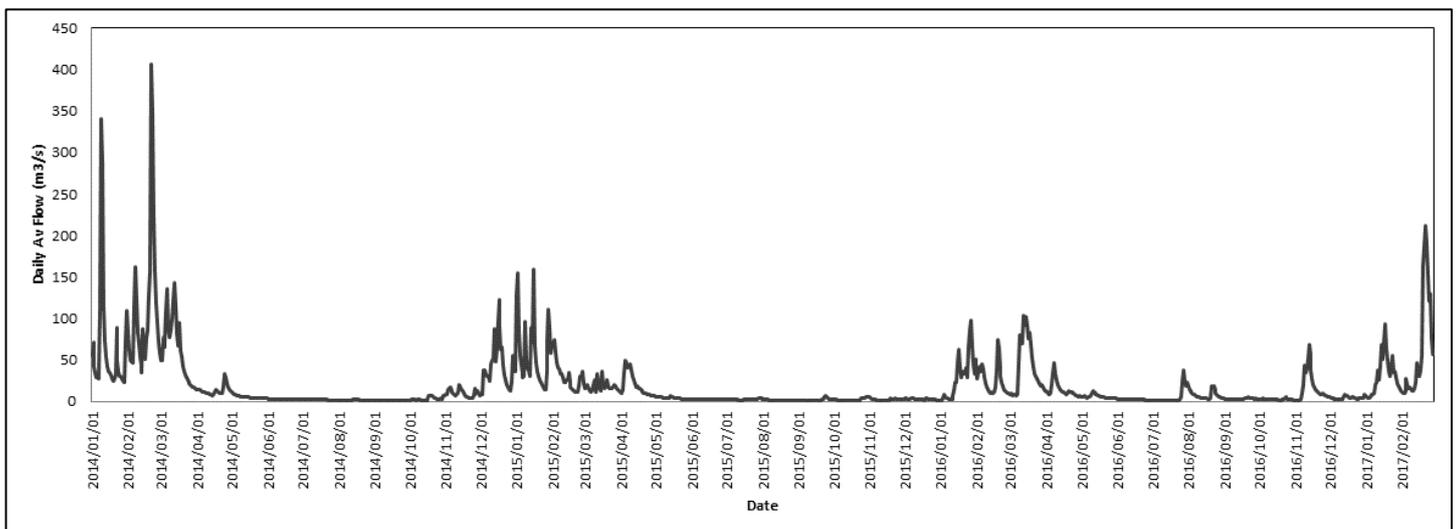
**Figure 2-15: Daily average streamflow ( $\text{m}^3\cdot\text{s}^{-1}$ ) from 2014 to 2017 measured at T3H006 in the Tsitsa River.**
