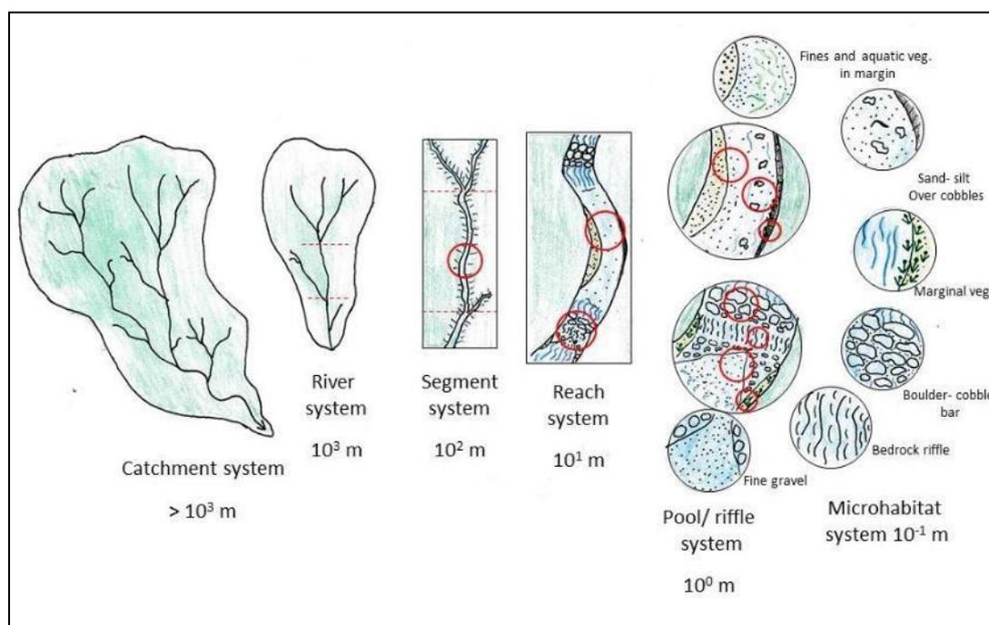
**Figure 6-1: Hierarchical nature of rivers, from a large catchment scale to successively smaller scales of river segments, channel reaches, individual channel units (such as pools and riffles) and microhabitats (Adapted from Allan, 2004).**
