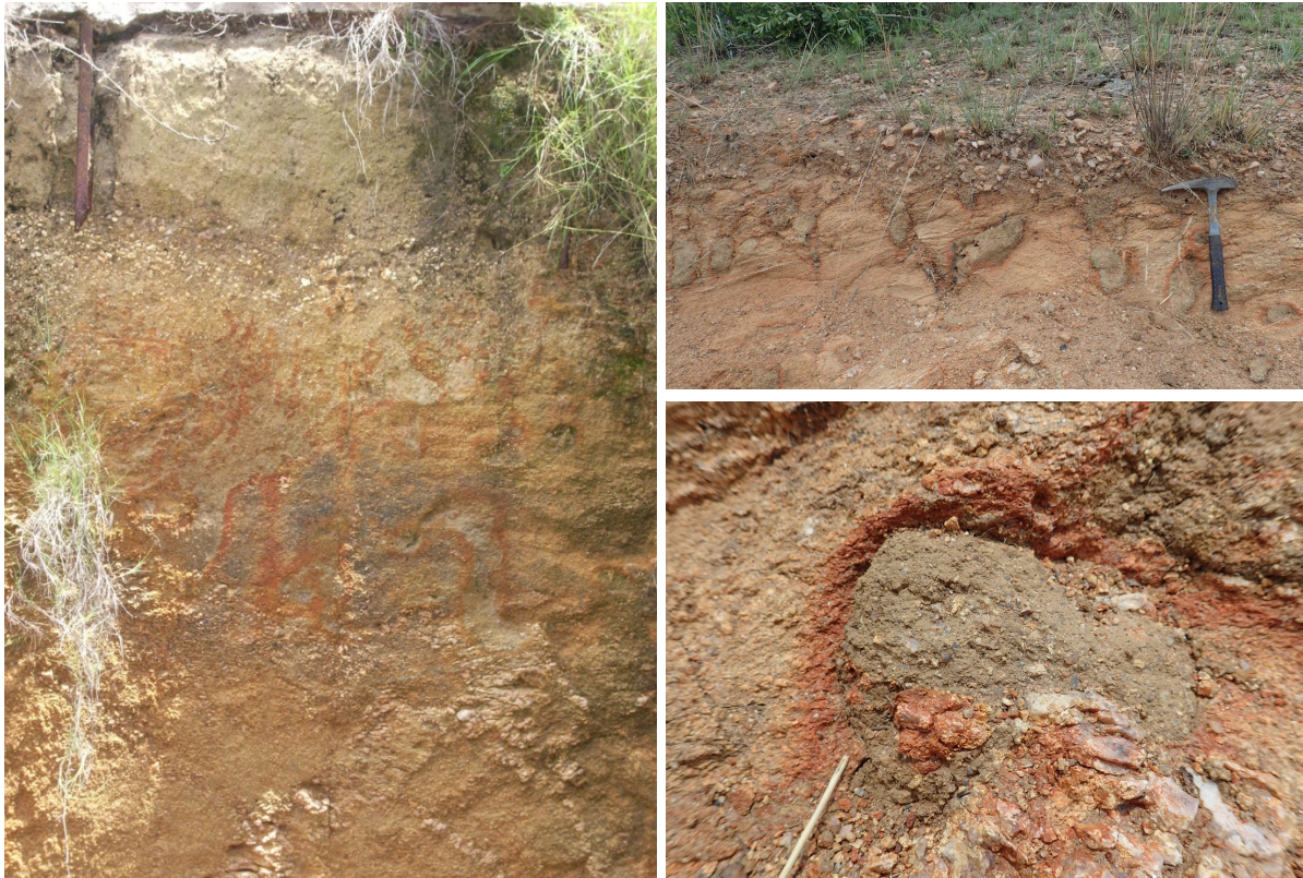
Figure 7.31 Weathering profiles in granite in the form of tongues of bleached material and zones of distinct translocation and accumulation of Fe
