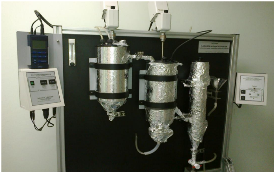
Figure 3.2: The laboratory-scale activated sludge reactor used during this investigation
