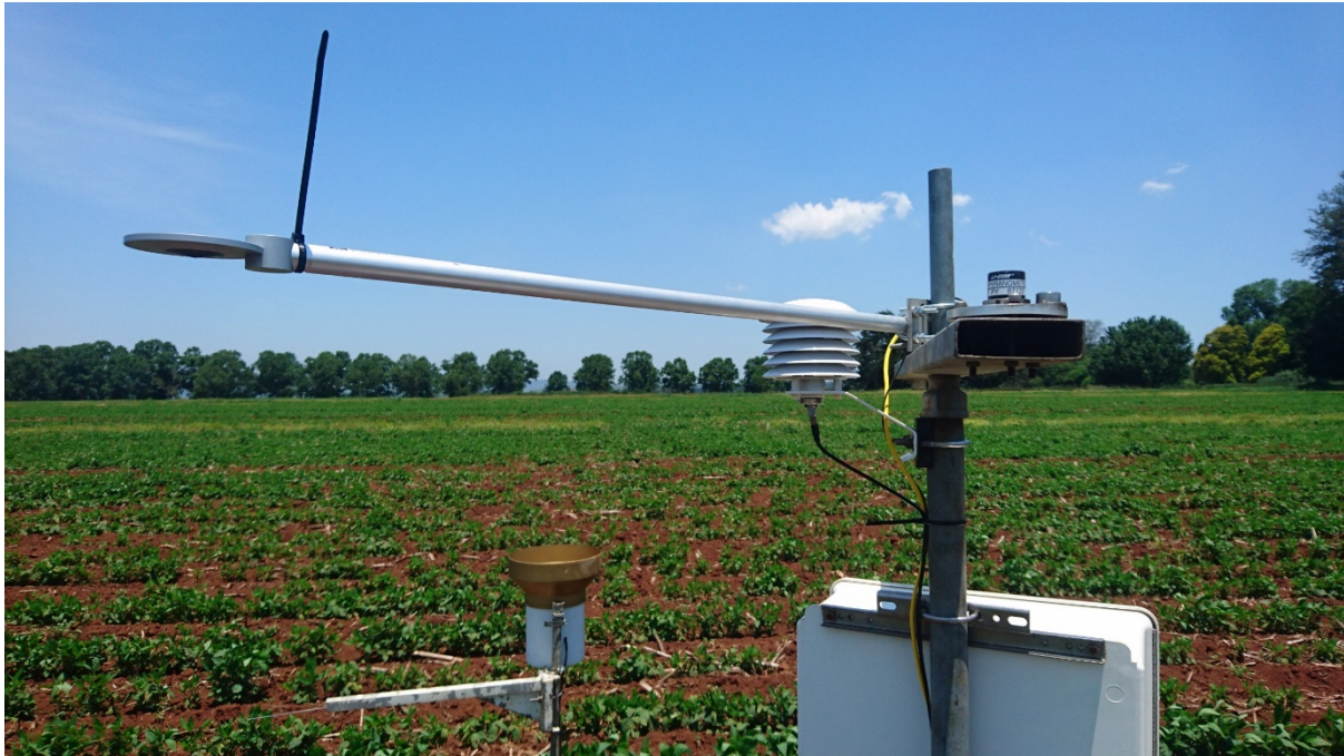
Figure 6.2: NR-Lite2 net radiometer, LI200S pyranometer and Gill radiation shield housing a single air temperature and relative humidity sensor (HMP50), as well as a Texas Electronics tipping bucket rain gauge (Baynesfield Estate: 2016/17 season)
