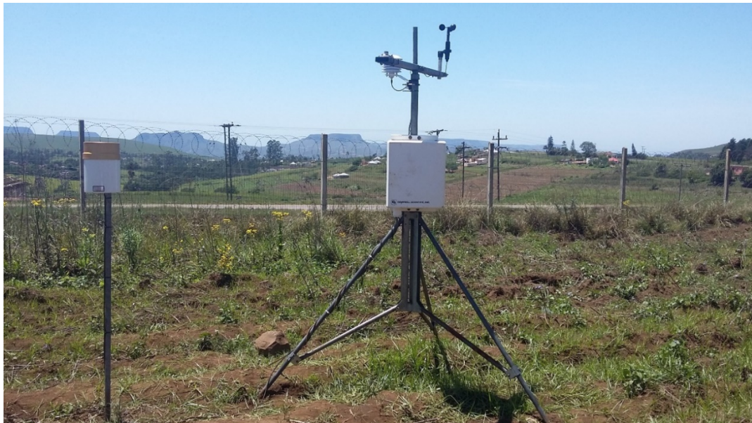
Figure 5.2: Automatic weather station installed at Swayimane during the 2015/16 season
