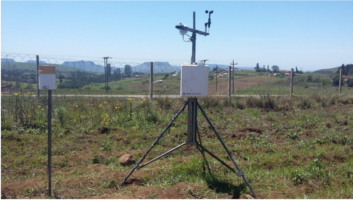
Figure 7.1: Automatic weather station installed at Swayimane in the 2017/18 season
