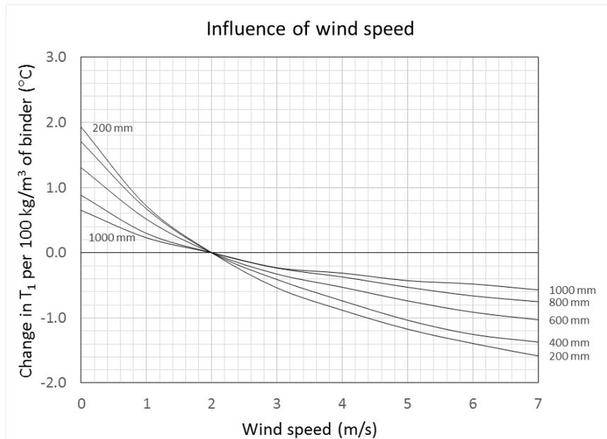
**Figure 2.17: Change in  $T_1$  (per 100 kg/m<sup>3</sup> CEM I) for changes in wind speed**
