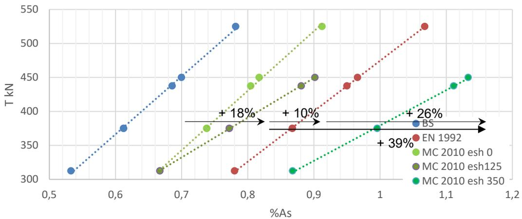
Figure 6.9: Reinforcement ratios for long-term tension,  $w_k = 0.2$  mm
