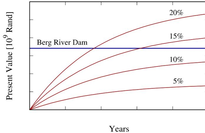
**Figure 8.1: Present value of accumulated savings resulting from sustained reductions of 5 to 20% in water loss volumes, calculated using consumption figures relevant to the City of Cape Town, and assuming a discount rate of 5%. The estimated replacement value of the Berg River Dam (adjusted to 2019 values) is shown for comparison.**
