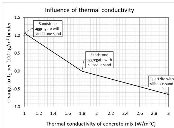
**Figure 2.18: Change in  $T_1$  (per 100 kg/m<sup>3</sup> CEM I) for changes in thermal conductivity**
