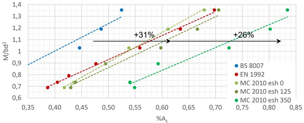
Figure 6.7: Reinforcement ratios for long-term bending,  $w_k = 0.2$  mm
