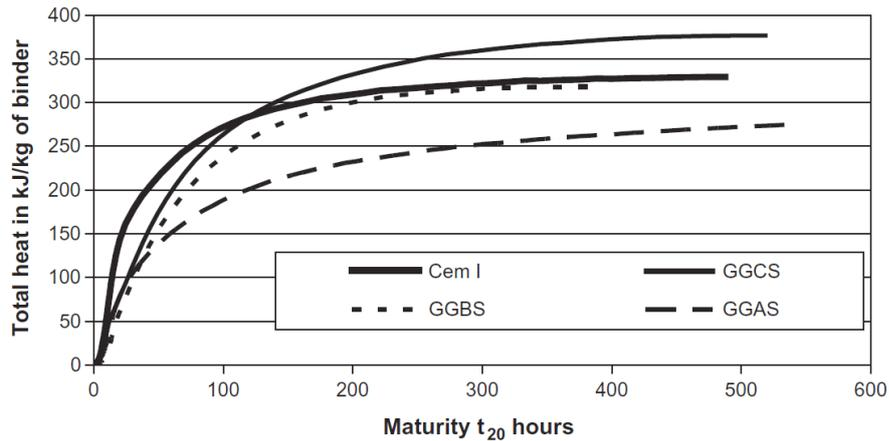
**Figure 2.6: Adiabatic heat curves of different South African mortar blends (Beushauzen et al., 2012)**
