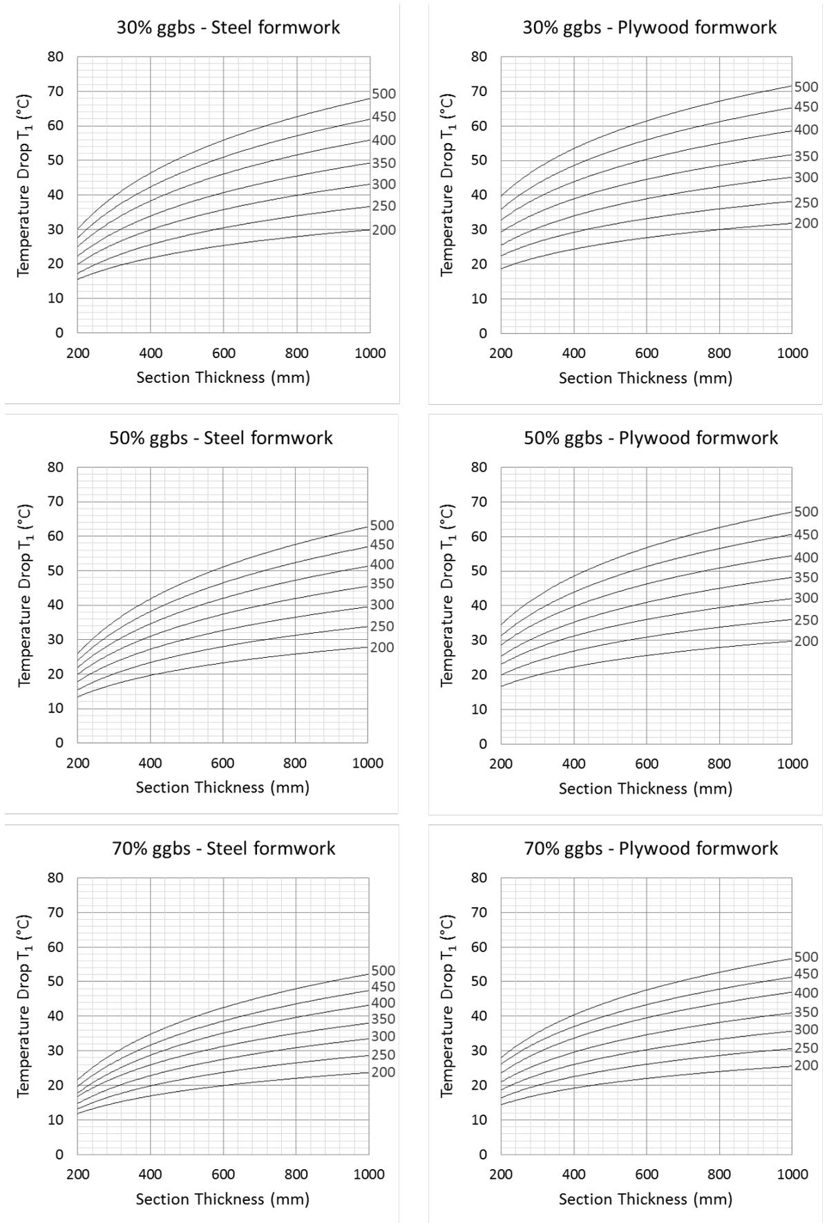
Figure 2.12: The  $T_1$  values for walls with concrete (of different binder content) containing GGBS
