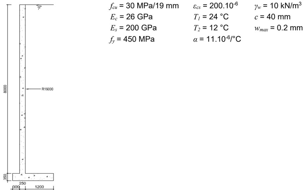
Figure 3.6: Wall of 6 Mℓ reservoir
