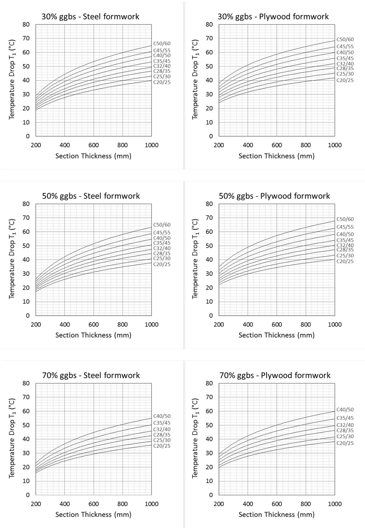
Figure 2.13: The  $T_1$  values for walls with concrete (of different strength classes) containing GGBS
