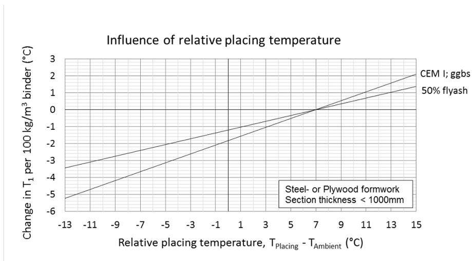
**Figure 2.16: Change in  $T_1$  (per 100 kg/m<sup>3</sup> binder) for changes in relative placing temperature, including active cooling**
