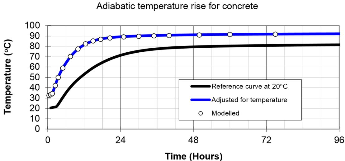
**Figure 2.8: Adiabatic temperature rise curve for a concrete mix of 100% CEM I with 400 kg/m<sup>3</sup> binder content, a specific heat of 1 kJ/kg °C and a wet density of 2,400 kg/m<sup>3</sup>**
