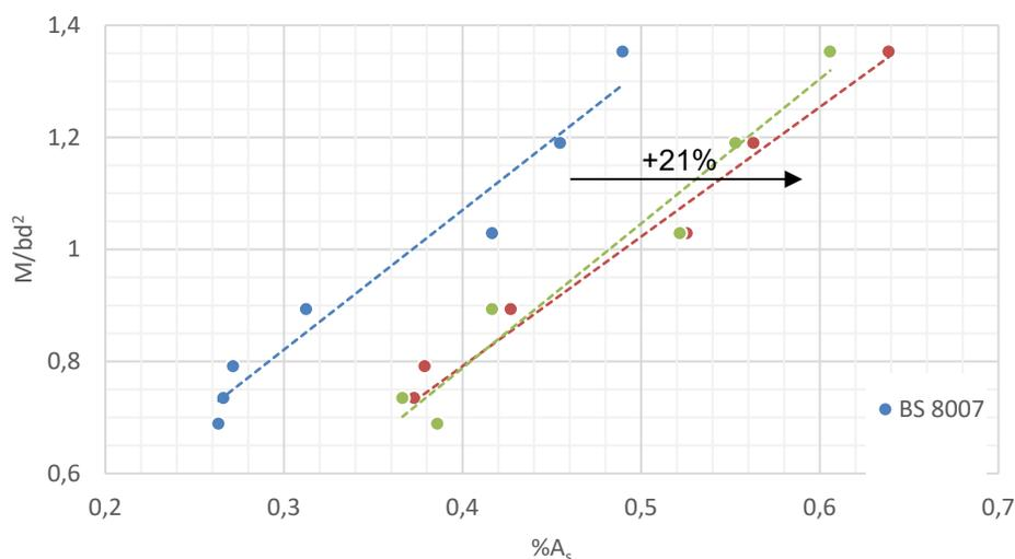
Figure 6.6: Reinforcement ratios for short-term bending,  $w_k = 0.2 \text{ mm}$
