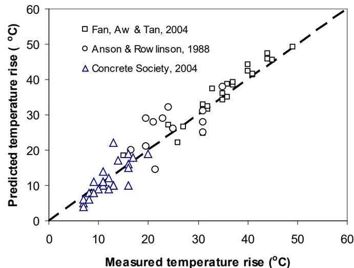
**Figure 2.1: Measured temperature rise values compared to Bamforth’s predictions (Bamforth, 2007)**
