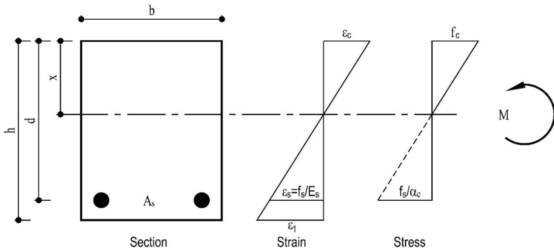
**Figure 3.2: Assumed stress and strain diagram for cracked section, elastic design**
