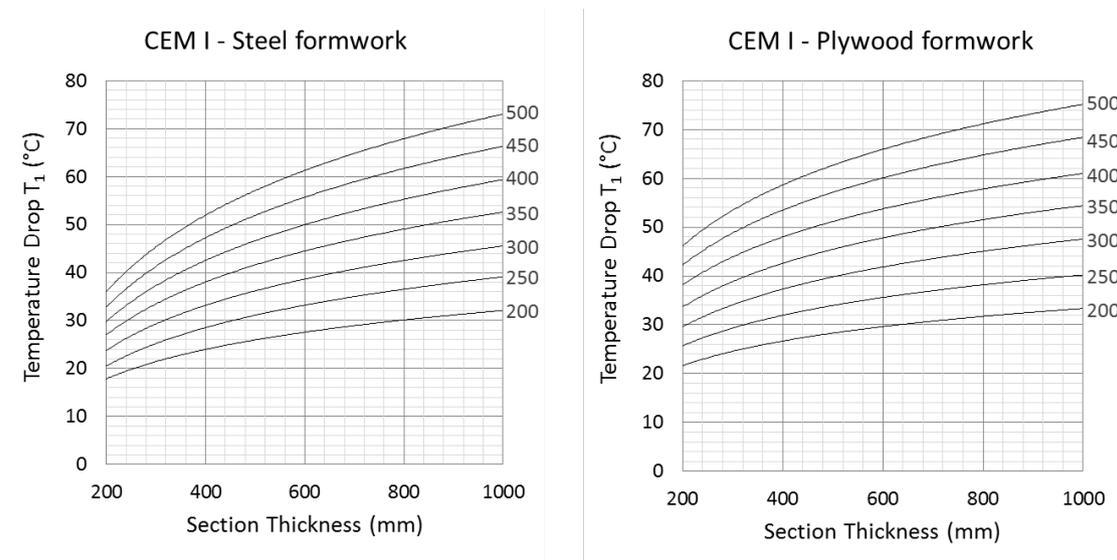
**Figure 2.10: The  $T_1$  values for walls of CEM I concrete (of different binder content)**
