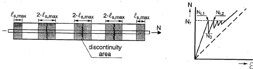
**Figure 6.1: Behaviour of a reinforced prismatic bar subjected to imposed deformation (crack formation stage)**
