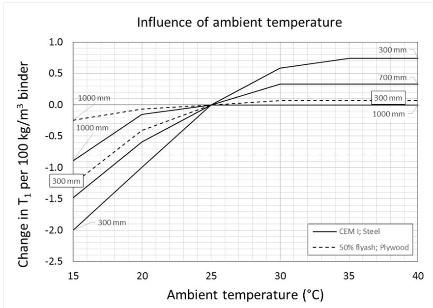
**Figure 2.19: Change in  $T_1$  (per 100 kg/m<sup>3</sup> binder) for changes in mean ambient temperature**
