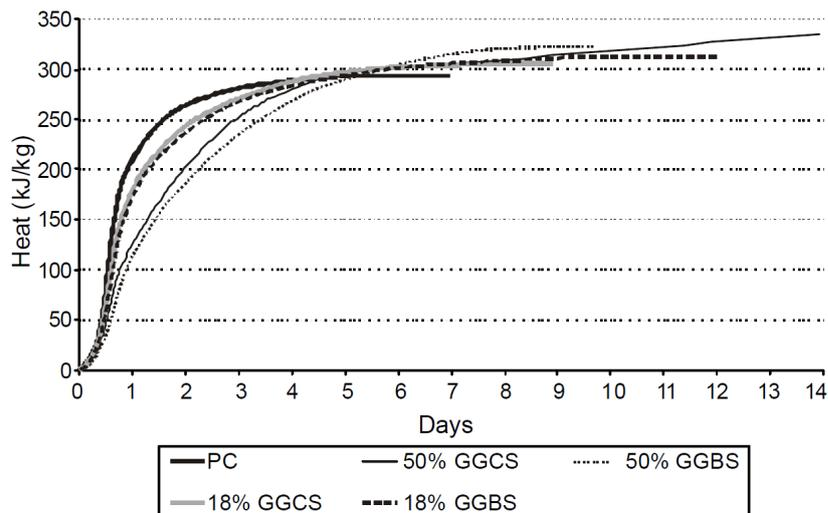
**Figure 2.5: Adiabatic heat curves of different slag binder combinations available in South Africa (Alexander et al., 2003)**
