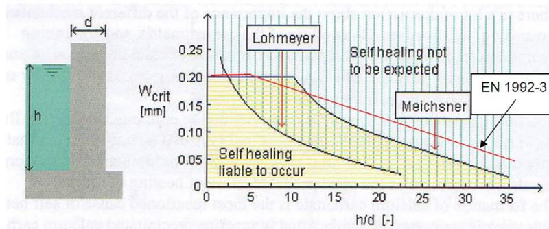
**Figure 6.10: Comparison of EN 1992-3 through crack width limits to research findings (from Jones, 2008)**
