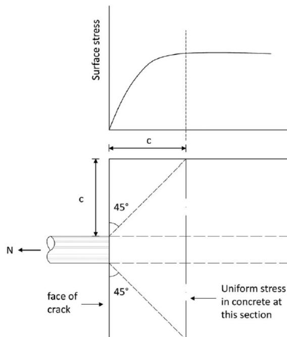
**Figure 6.3: No-slip mechanism of cracking: relationship between  $c$  and transfer length (from the old British Code for structural concrete, CP 110)**
