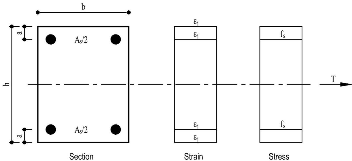
**Figure 3.4: Section under direct tension, assumed stress and strain diagram**
