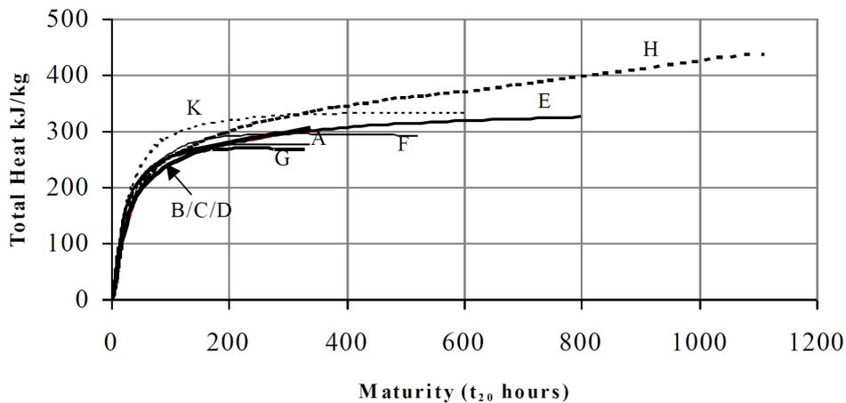
**Figure 2.2: Adiabatic heat curves of different clinker cements (Ballim and Graham, 2004b)**
