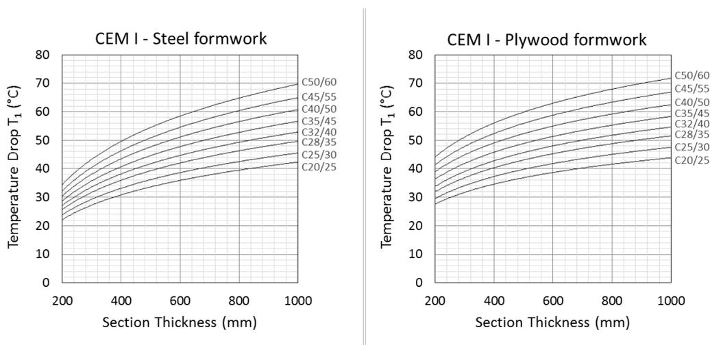
**Figure 2.11: The  $T_1$  values for walls of CEM I concrete (of different strength classes)**
