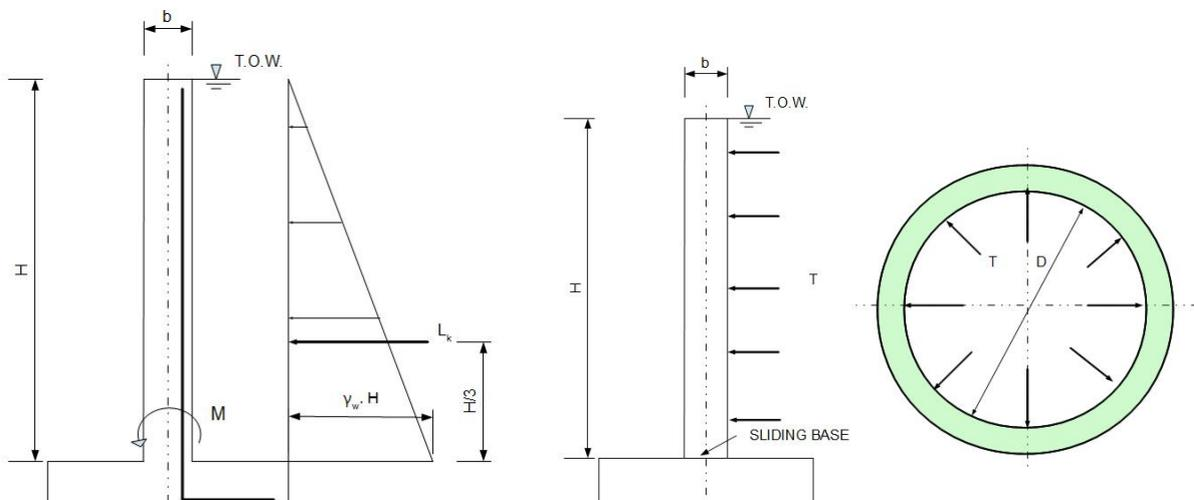
**Figure 6.4: Rectangular (left) and circular reservoir (right) wall configurations**
