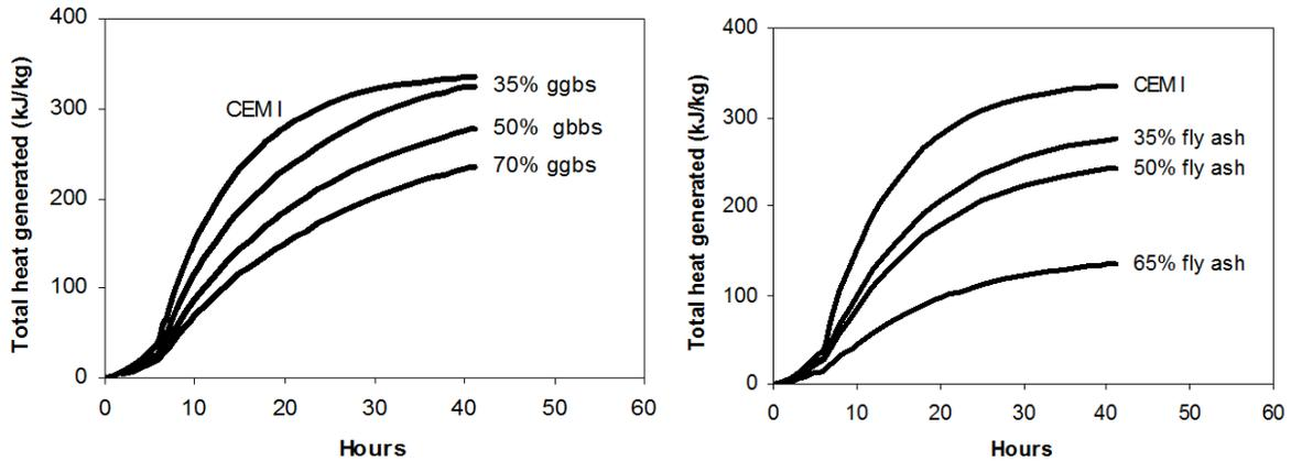
**Figure 2.4: Adiabatic heat curves of different mortar blends (Dhir et al., 2006)**
