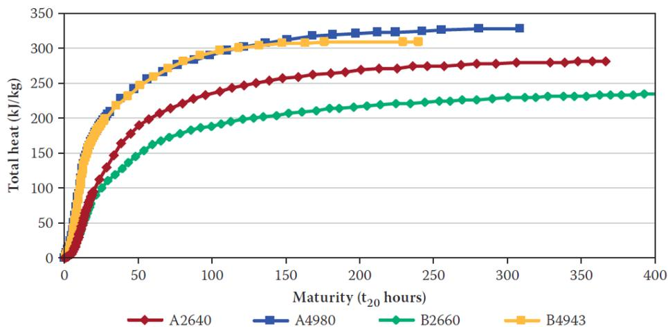
**Figure 2.3: Comparison of total heat profiles of low and high fineness (2,640 cm<sup>2</sup>/g and 4,980 cm<sup>2</sup>/g) cements produced from two clinker types (A and B) (Graham et al., 2011)**
