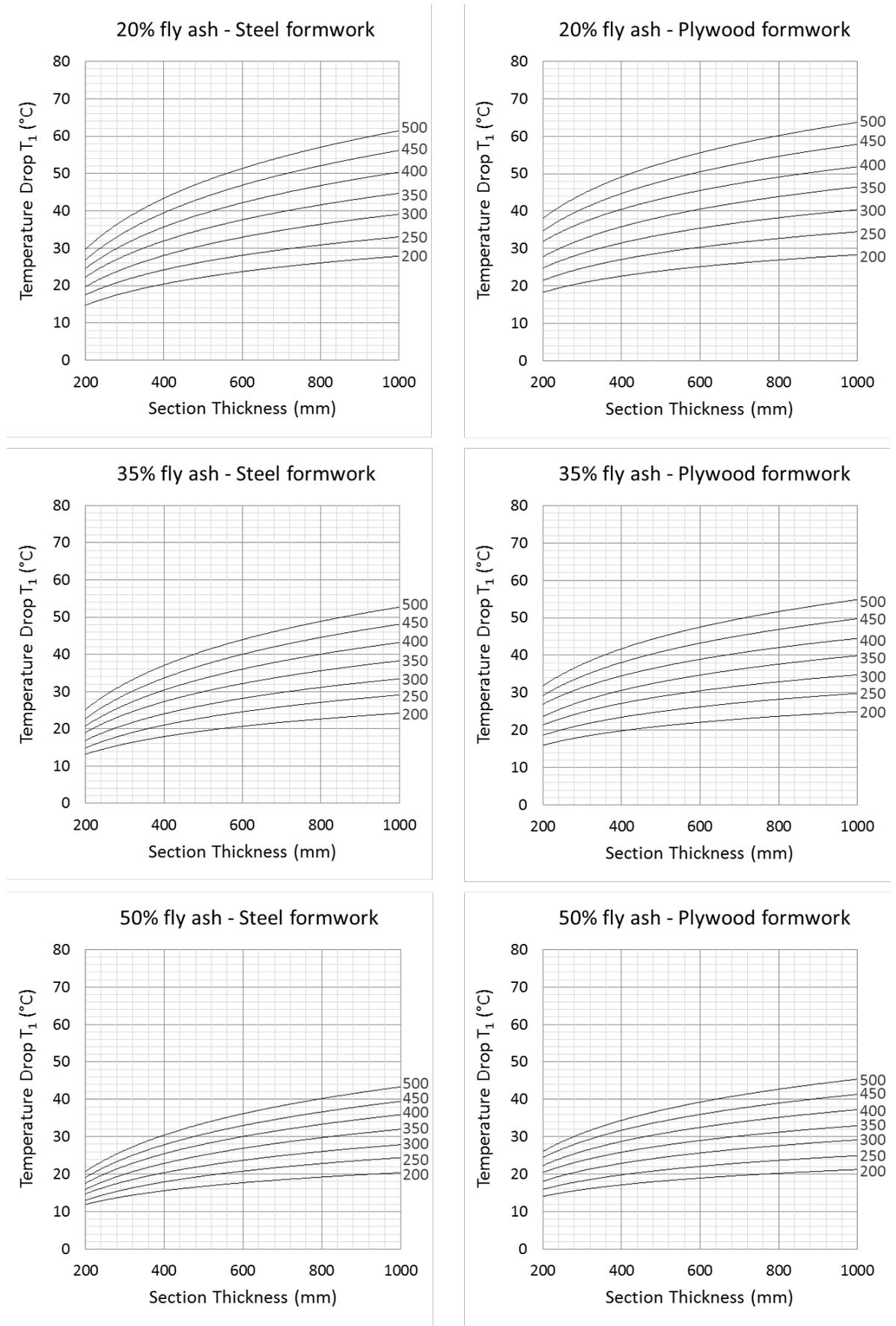
Figure 2.14: The  $T_1$  values for walls with concrete (of different binder content) containing fly ash
