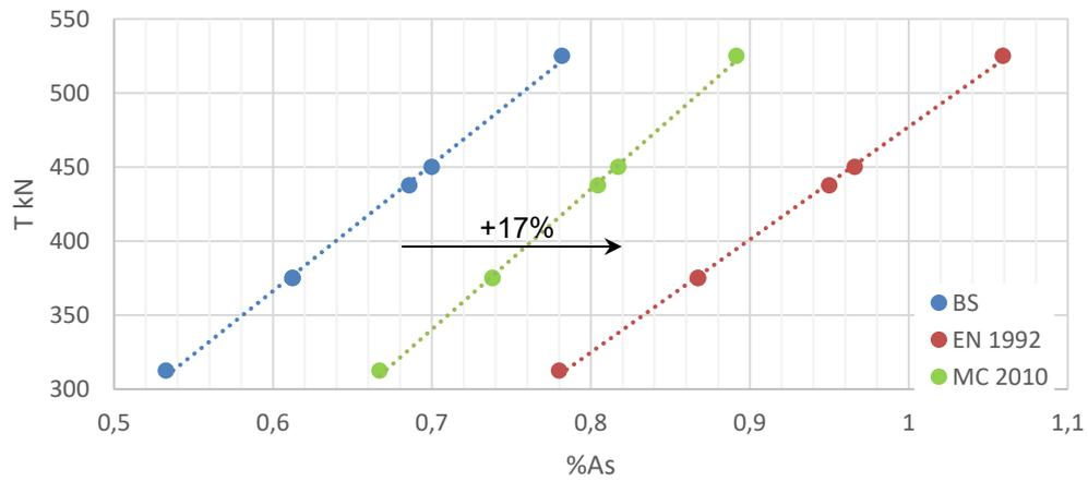
Figure 6.8: Reinforcement ratios for short-term tension,  $w_k = 0.2$  mm
