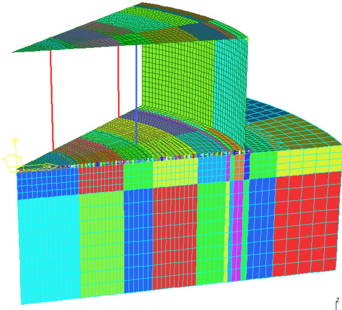
**Figure 3.5: Finite element model of 6 Mℓ reservoir**
