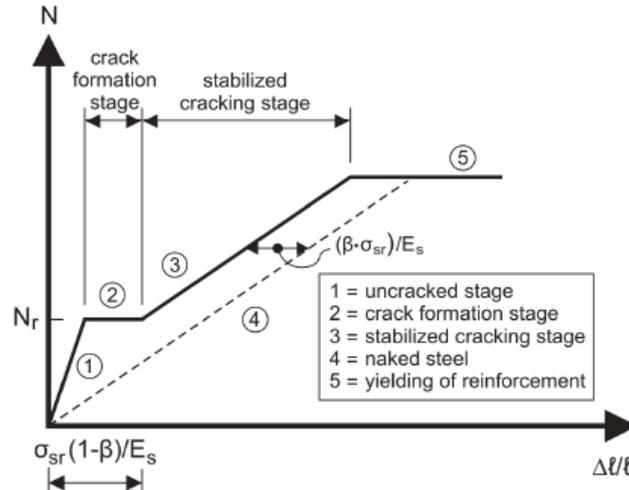
**Figure 6.2: Simplified load – strain relation for a reinforced prismatic bar subjected to tension**
