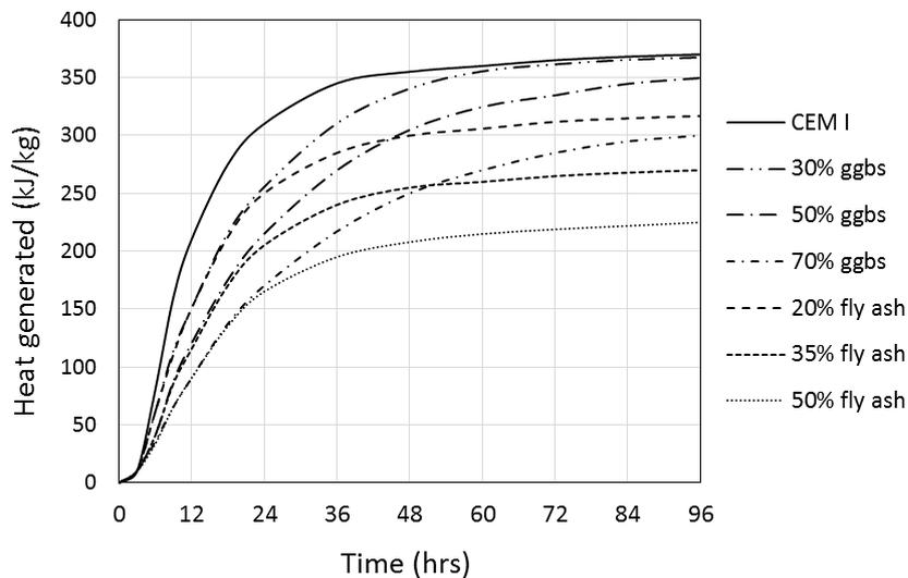
**Figure 2.7: Design curves for adiabatic heat (10% probability of exceedance values) of concretes used in the Bamforth model (Bamforth, 2007)**
