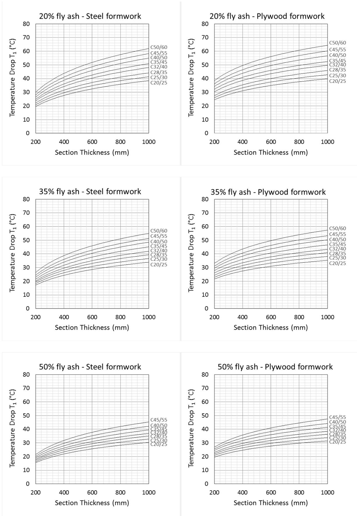
Figure 2.15 : The  $T_1$  values for walls with concrete (of different strength classes) containing fly ash
