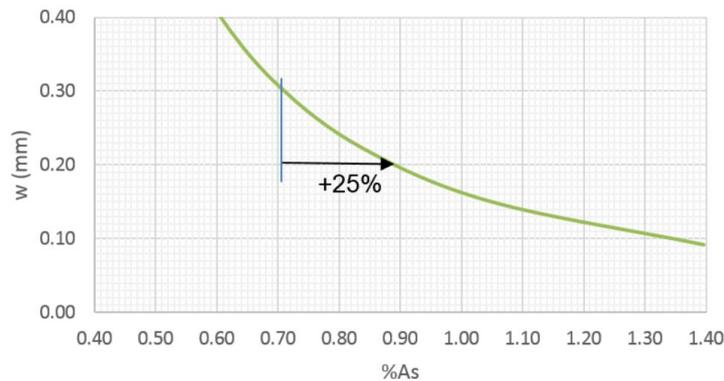
**Figure 6.11: Reinforcement implication of crack width limit in MC 2010 formulation (bending and flexure)**
