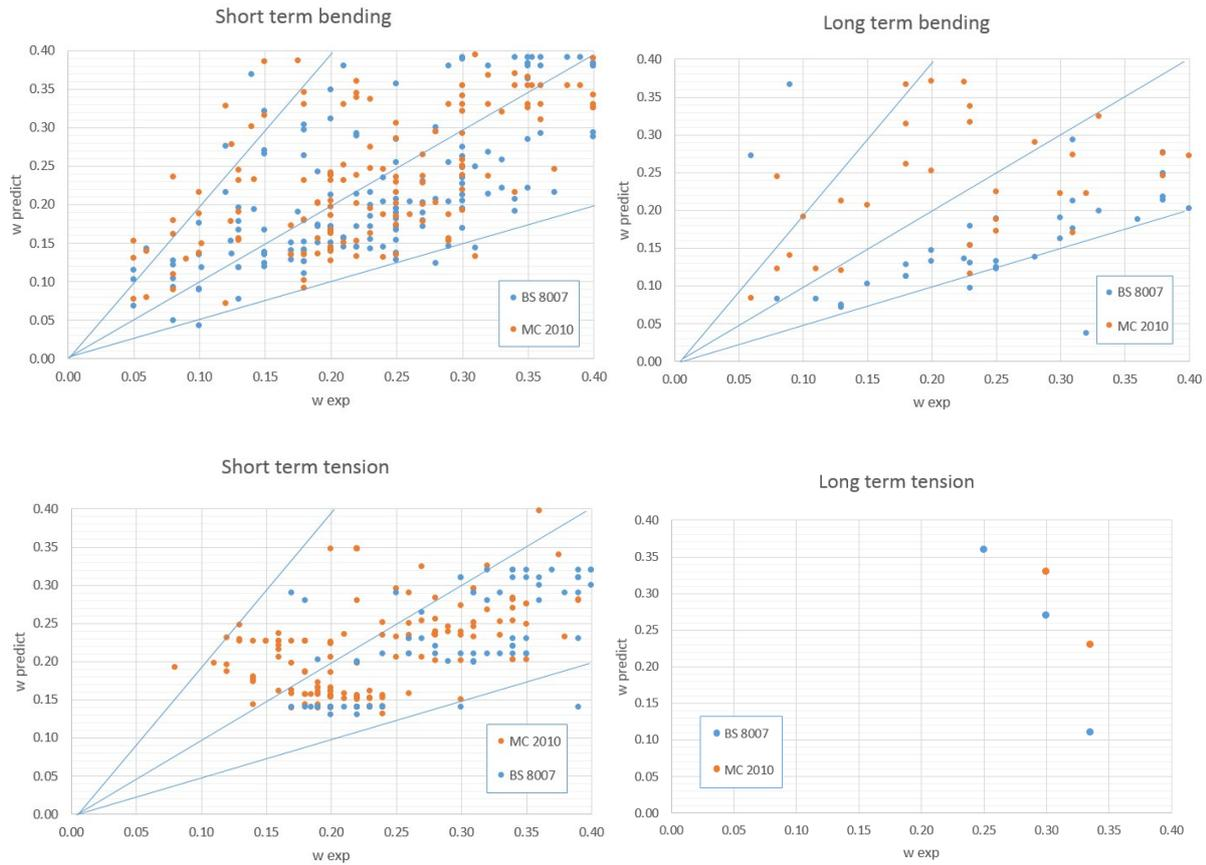
**Figure 6.5: Experimental vs MC 2010 and BS 8007 predicted crack widths for: (a) short-term bending, (b) long-term bending, (c) short-term tension and (d) long-term tension**
