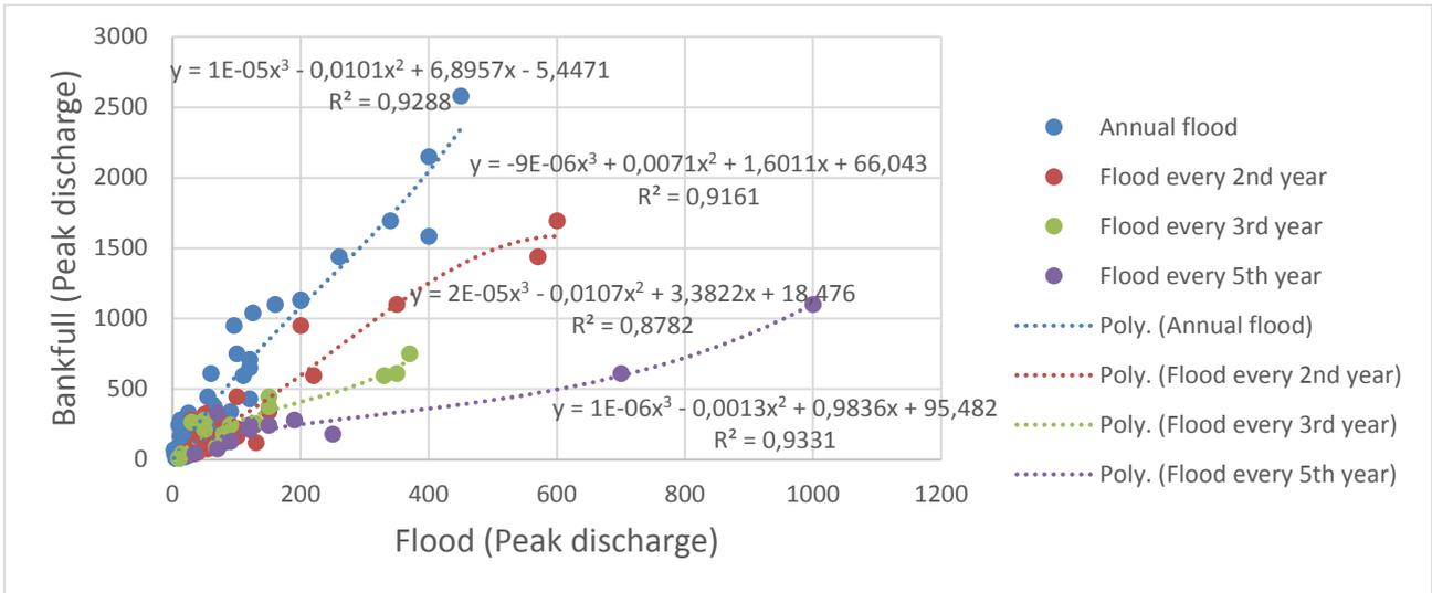
**Figure 3.2 Relationship between bankfull discharge and inter-annual flood requirements, including the annual flood.**
