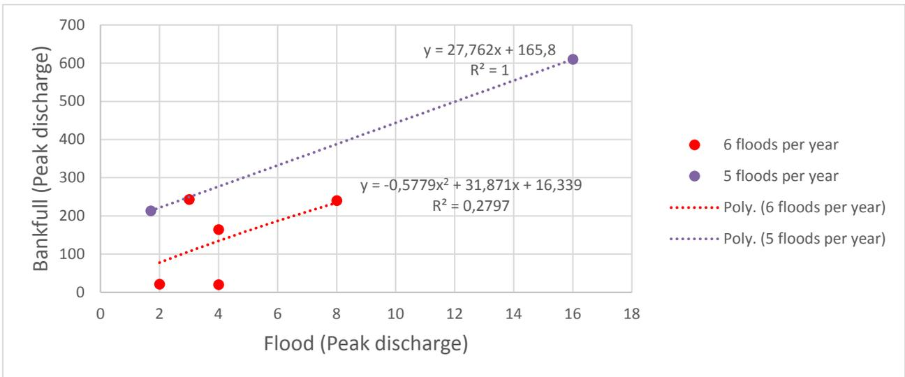
**Figure 3.3 Relationship between bankfull discharge and intra-annual flood requirements where 6 or 5 events are required per year.**
