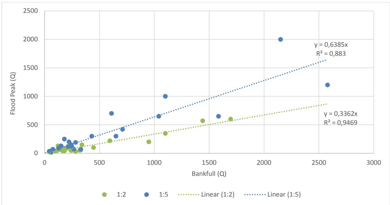
**Figure 3.13 Relationship between bankfull discharge and flood peak discharge for inter-annual floods.**
