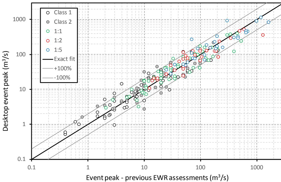
**Figure 4.4** Plot of event peaks for various flood classes as estimated by the RDRMv2 (post-October 2017 workshop) against values from previous (higher confidence) EWR assessments for numerous EWR sites
