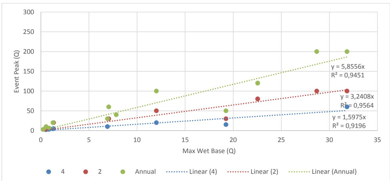
**Figure 3.14 Relationship between maximum wet season base flow and flood peak discharge, for within-year floods, including the annual event.**
