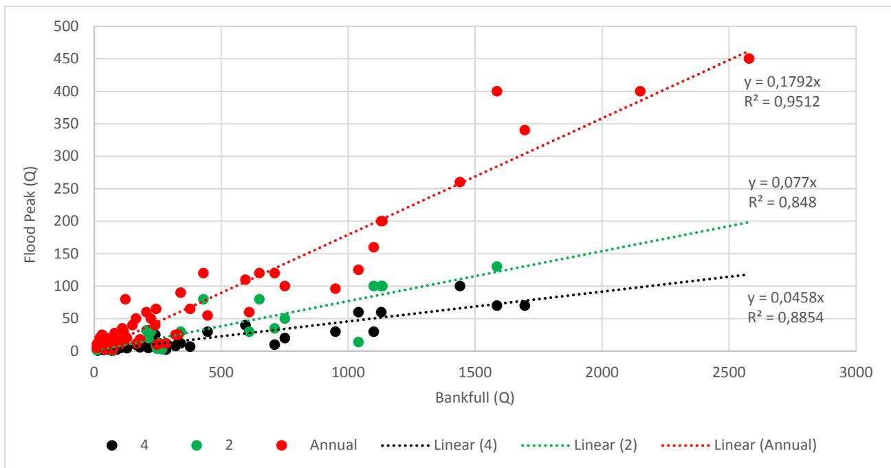
**Figure 3.12 Relationship between bankfull discharge and flood peak discharge for within-year floods, including the annual event.**
