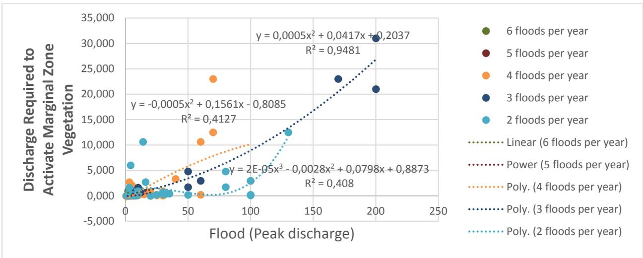
**Figure 3.10 Relationship between PD discharge required to activate marginal zone vegetation and intra-annual flood requirements.**
