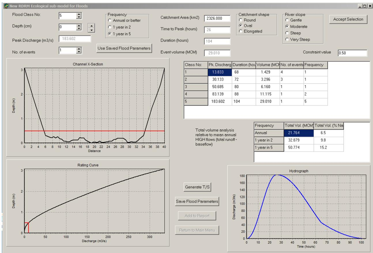
**Figure 4.2 Form for setting Reserve floods and high flow requirements**
