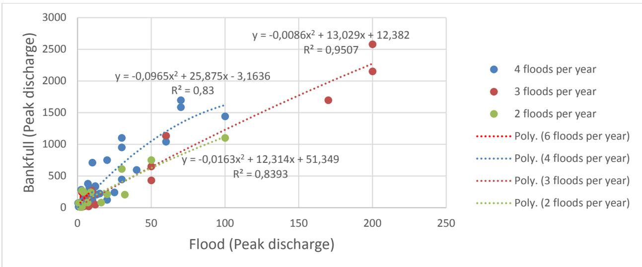
**Figure 3.1 Relationship between bankfull discharge and intra-annual flood requirements (6 events shown in Figure 3.3).**
