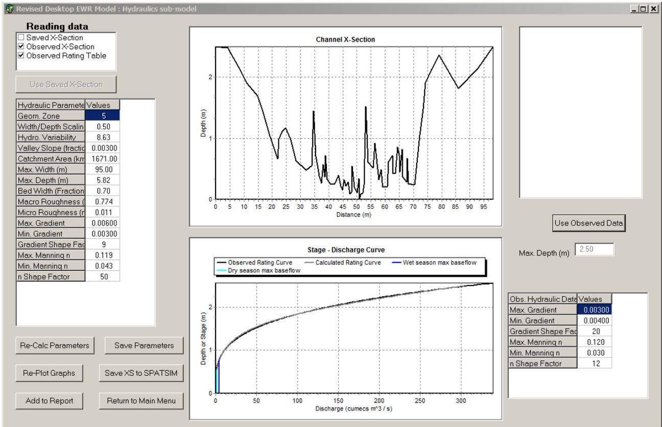
**Figure 14.3** The hydraulics sub-model form showing an observed cross-section (top-centre) and rating curve (bottom-centre; black curve), and fitted rating values (bottom-right textbox) that differ from the desktop values (last six values in the left textbox); the calculated rating curve (grey) is aligned with the observed curve.
