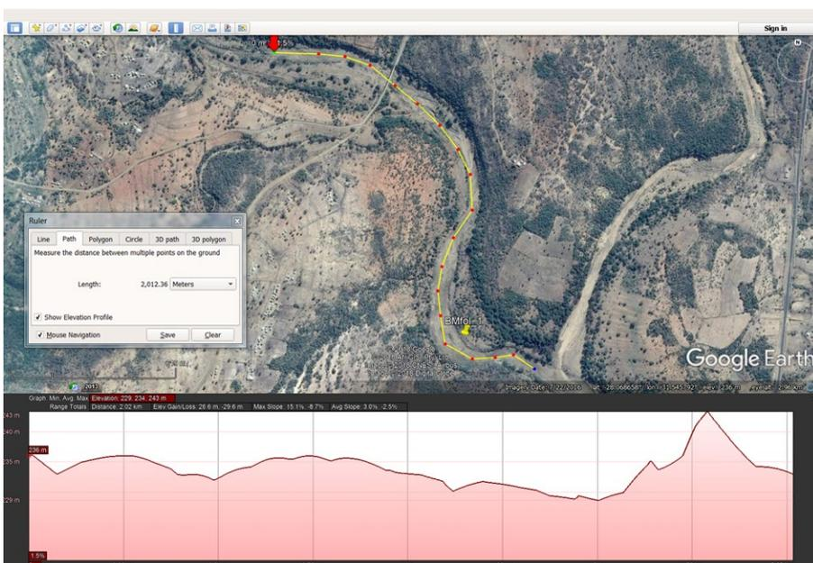
**Figure 5.3** Alternative option of measuring the difference in elevation
