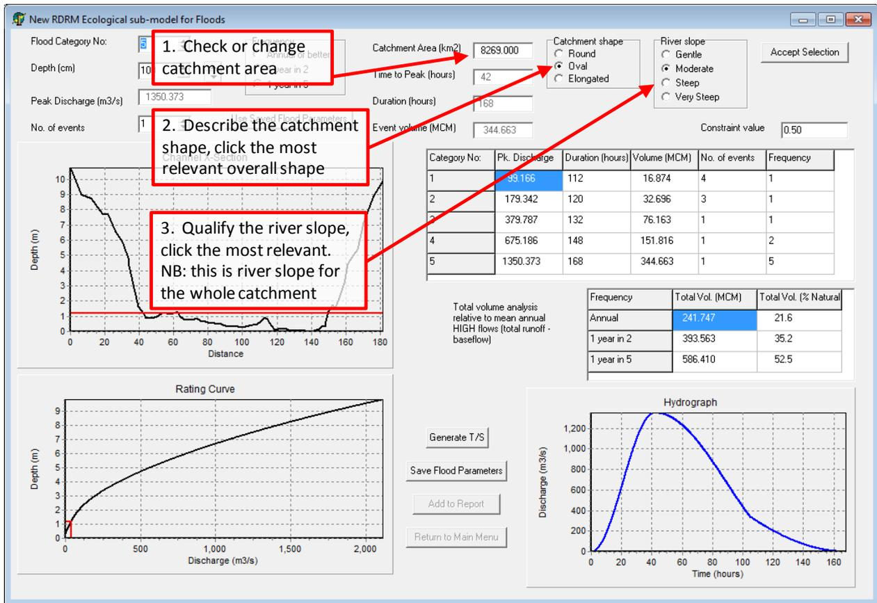
Figure 16.2 Adjusting catchment characteristics.
