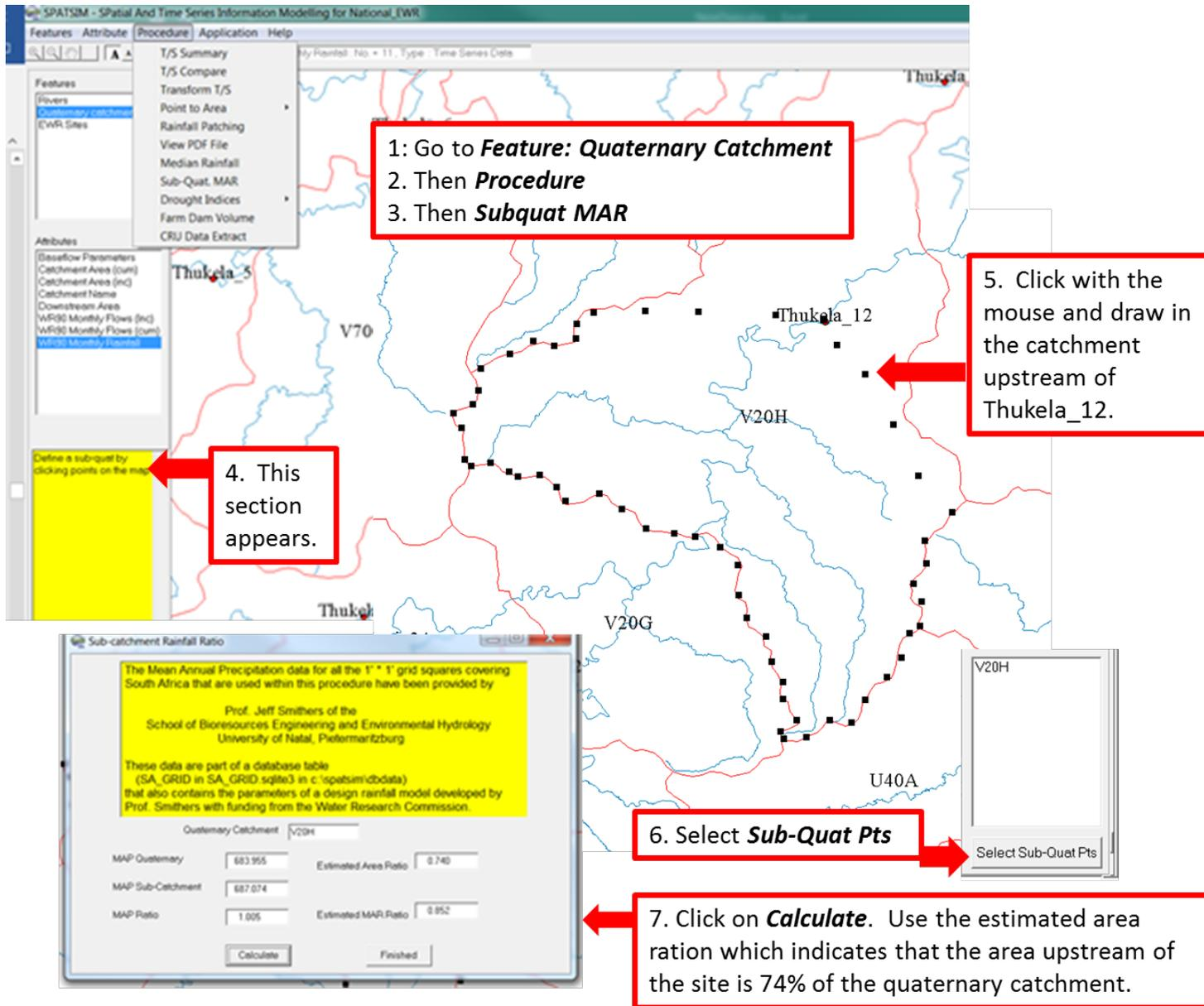
Figure 5.6 Determining catchment area for a portion of a quaternary catchment
