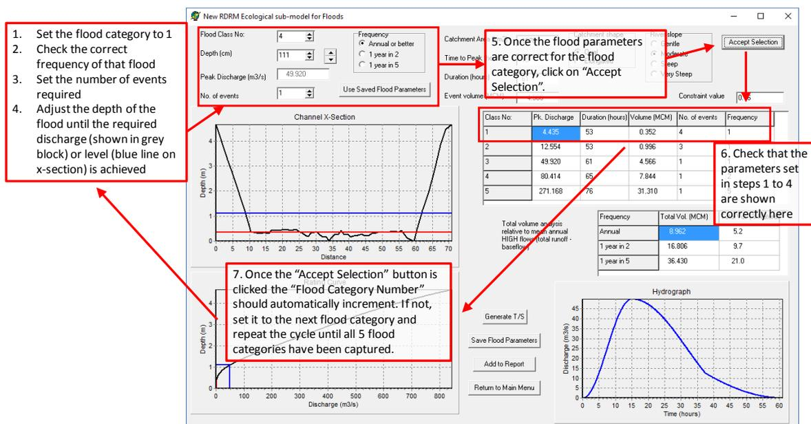
Figure 16.3 Overriding default flood parameters.
