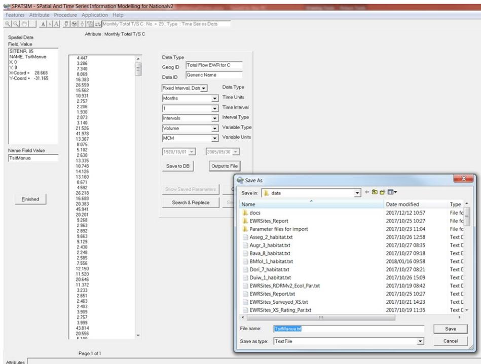
Figure 12.3 Screen showing how to output and save attributes such as a specific time series
