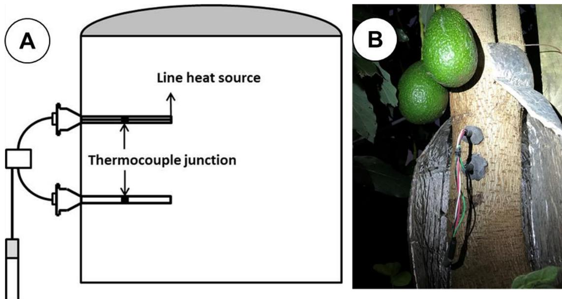
**Figure 3.6: A) Schematic representation of the thermal dissipation technique and B) the insertion of the probe into an avocado tree in the non-bearing orchard**
