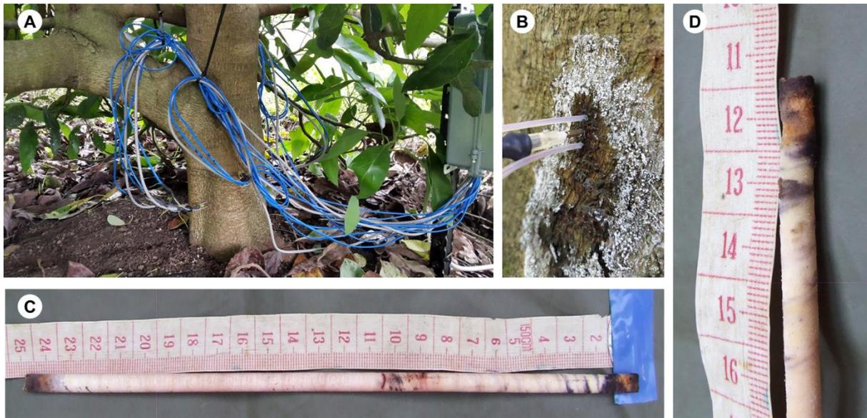
**Figure 3.4: A) A stem at the intermediate orchard instrumented with four sets of heat ratio measurement thermocouples and heaters. Junction box located on the right-hand side. B) A pair of thermocouples with a heater between them. C) Cores taken from the mature orchard, D) clearly showing the bark to be 10 mm thick.**
