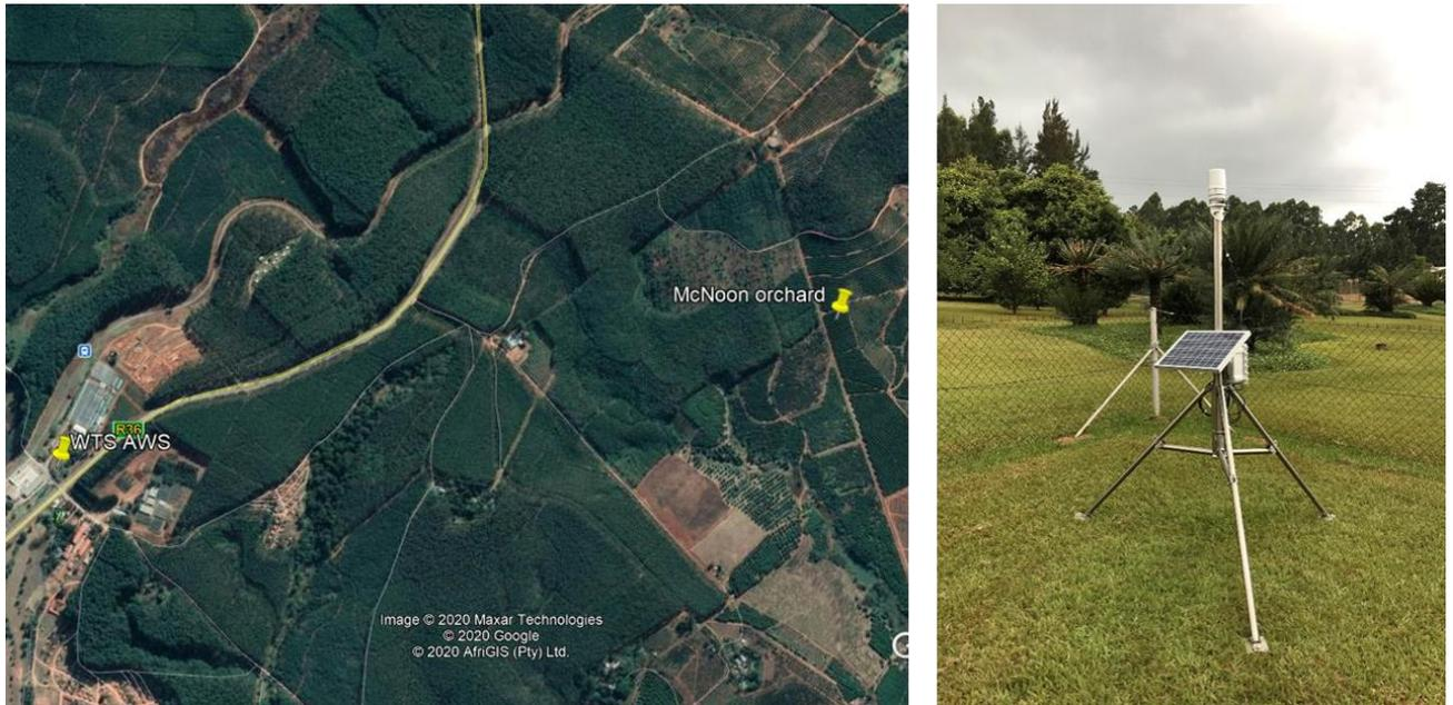
**Figure 3.13: Location of automatic weather station located close to the Westfalia offices in Tzaneen relative to the measurement orchard and the automatic weather station consisting of a ClimaVue 50 system.**
