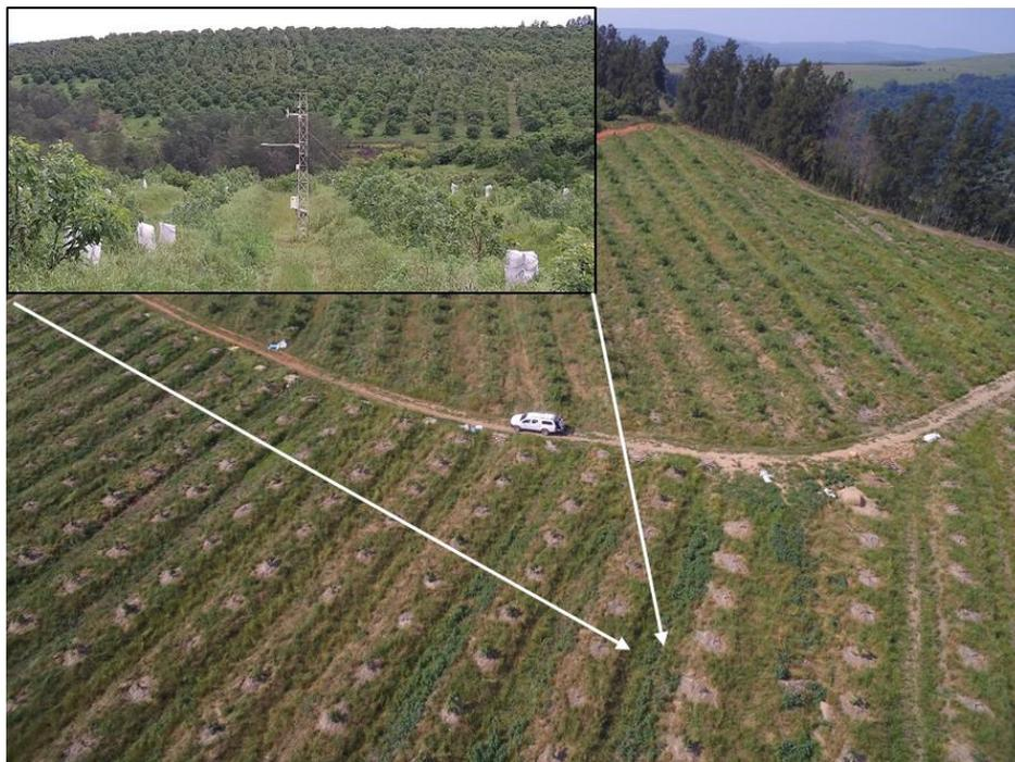
**Figure 3.9: Location of the non-bearing orchard (NB) eddy covariance system on a 6 m lattice mast**
