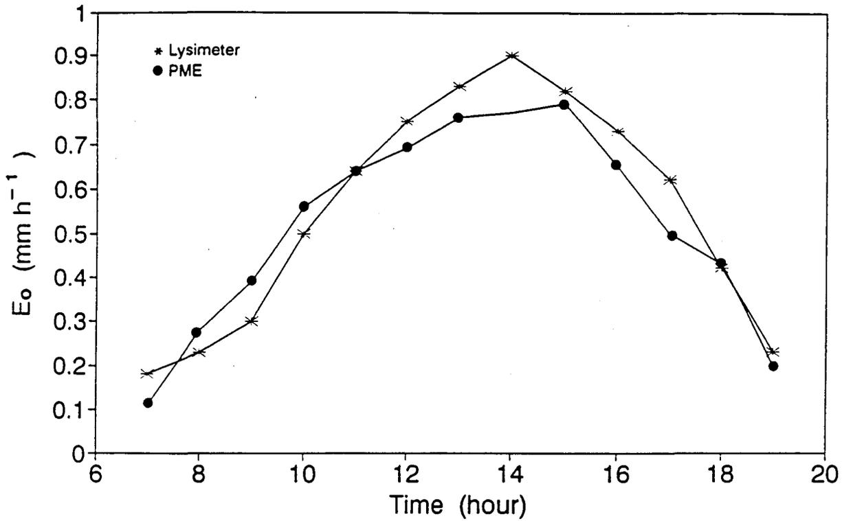
FIG. 3.4 Hourly variation of  $E_o$  measured lysimetrically and estimated from the PME over the daylight period during 1990.
