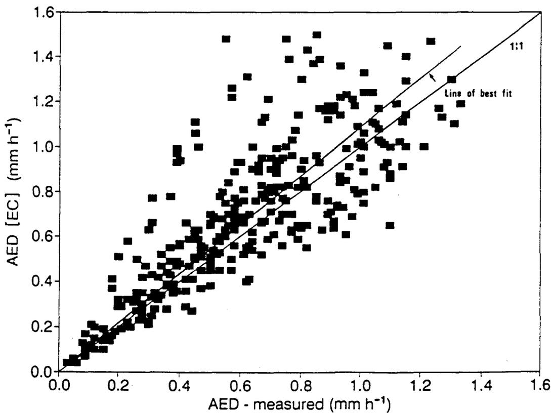
FIG. 4.2 Comparison between hourly AED measured lysimetrically and AED measured using EC technique.
