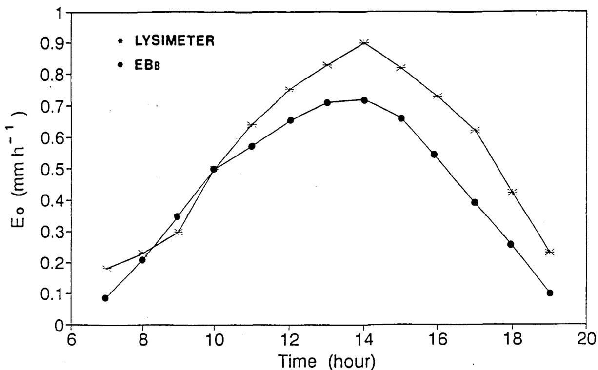
FIG. 3.2 Hourly variation of  $E_o$  measured lysimetrically and estimated from EBb over the daylight period during 1990.
