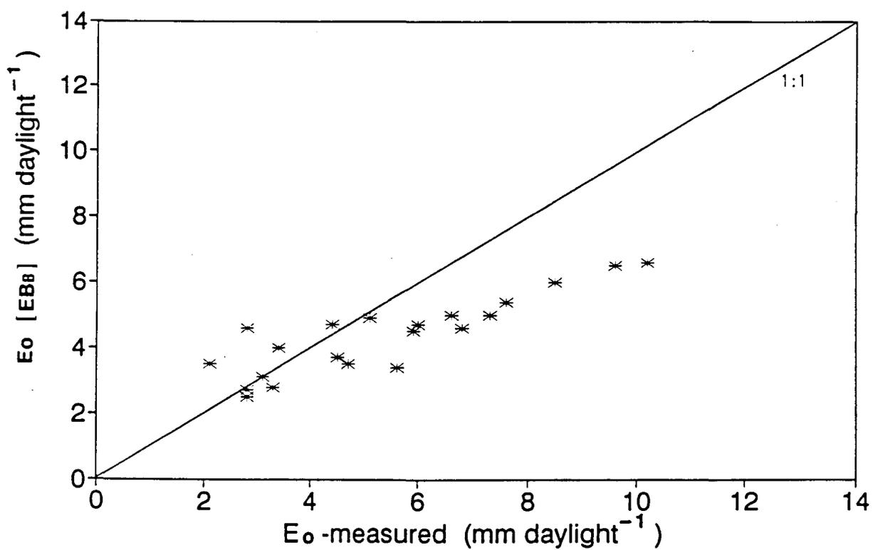
FIG. 3.7 Comparison between daylight  $E_0$  measured lysimetrically and  $E_0$  estimated from EB<sub>8</sub> during 1990.
