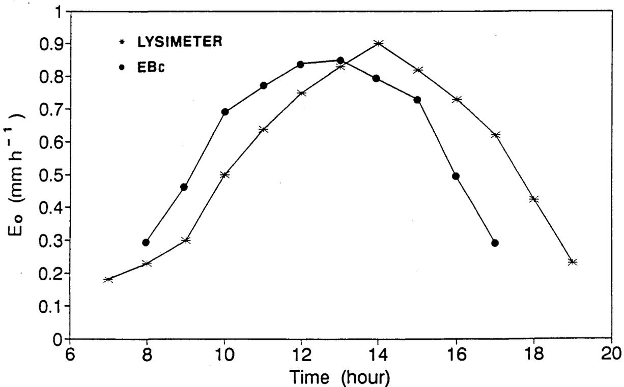
FIG. 3.5 Hourly variation of  $E_o$  measured lysimetrically and  $E_o$  estimated from EBC over the daylight period during 1990.
