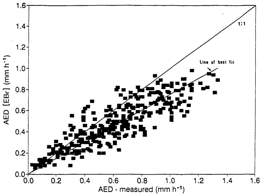
FIG. 4.1 Comparison between hourly AED measured lysimetrically and AED estimated from EBC
