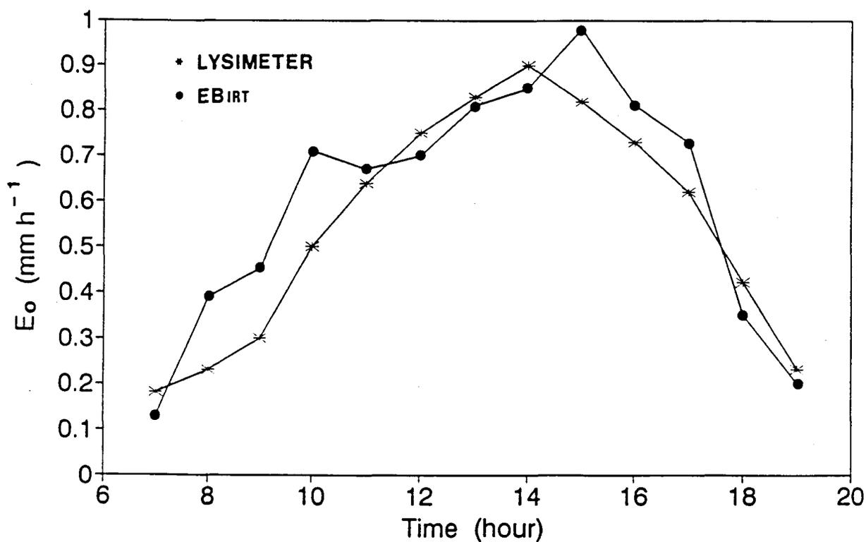
FIG. 3.3 Hourly variation of  $E_o$  measured lysimetrically and estimated from EBIRT over the daylight period during 1990.
