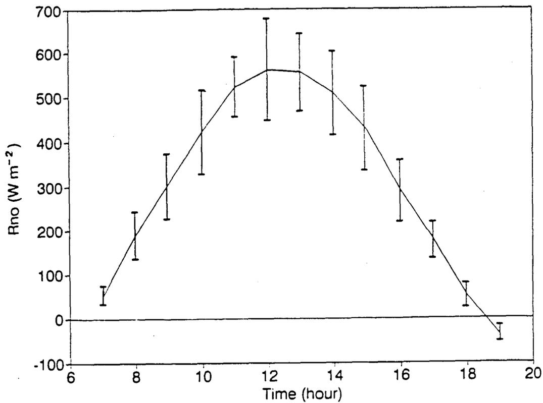
FIG. 5.13 Mean hourly variation in  $R_{no}$  for the period DOY 241 till 331. The bar indicates 1 standard deviation.
