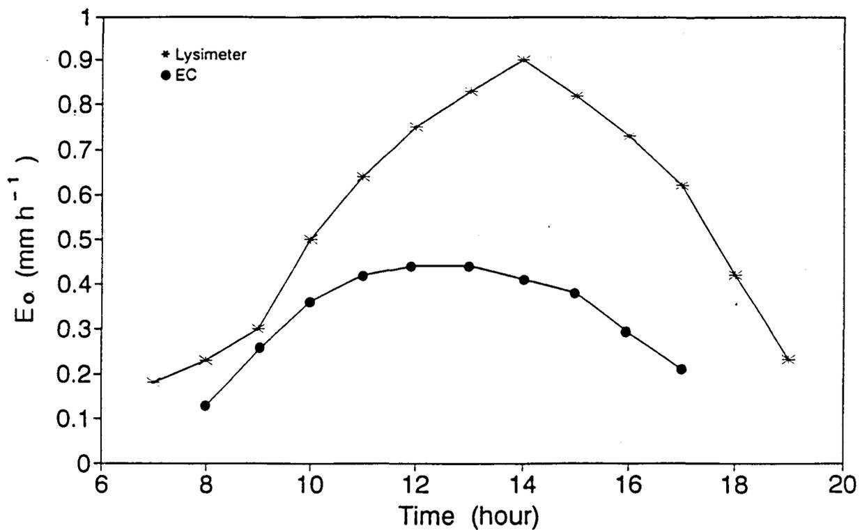
FIG. 3.6 Hourly variation of  $E_0$  measured lysimetrically and  $E_0$  estimated from EC over the daylight period during 1990.
