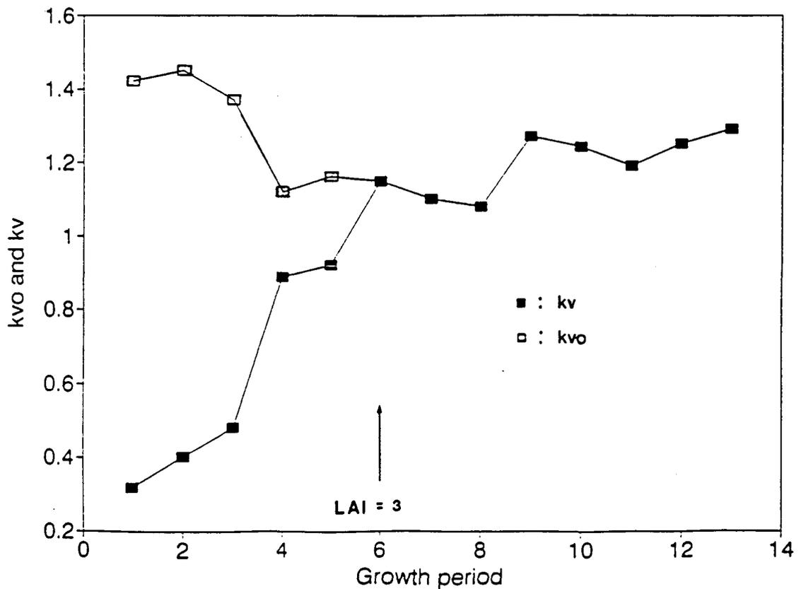
FIG. 2.2 Variation of  $k_{vo}$  and  $k_v$  with growth stage of wheat under virtually constant climatic conditions. Eqs. 2.17, 2.18 and 2.20 were used to calculate  $k_{vo}$  and  $k_v$ .
