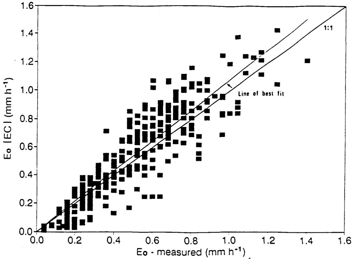
FIG. 3.12 Comparison between hourly  $E_o$  measured lysimetrically and  $E_o$  estimated from EC during 1992.
