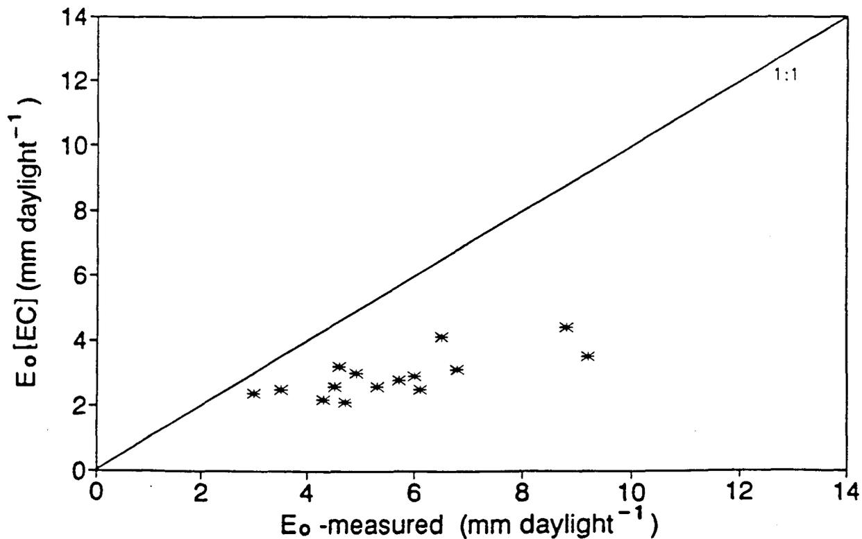
FIG. 3.11 Comparison between daylight  $E_0$  measured lysimetrically and  $E_0$  measured EC during 1990.
