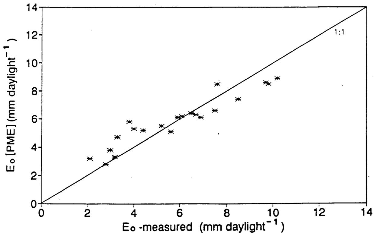
FIG. 3.9 Comparison between daylight  $E_o$  measured lysimetrically and  $E_o$  estimated from PME during 1990.
