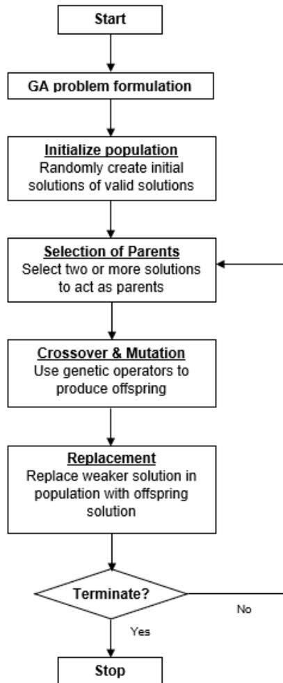
**Figure 2.1: Flow chart of the basic methodology of genetic algorithms**
