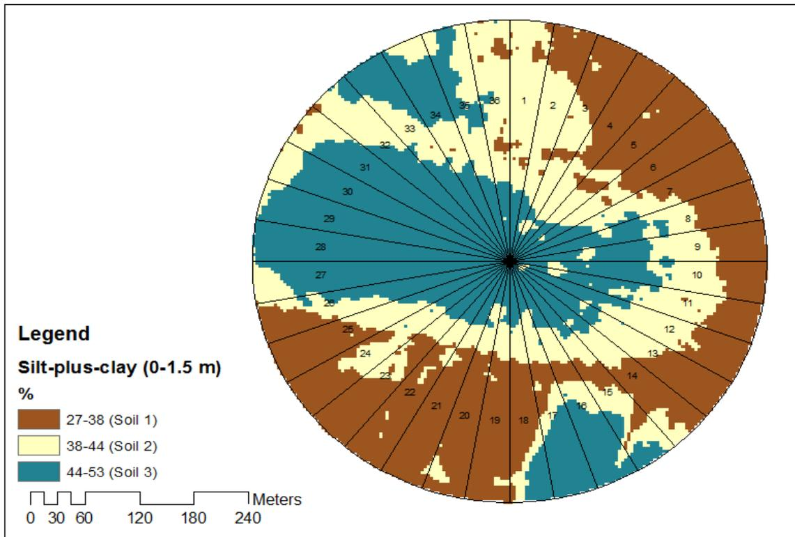
**Figure 3.6: Thematic map of the soils of a 39.9 ha centre pivot in the Orange-Riet Irrigation Scheme**
