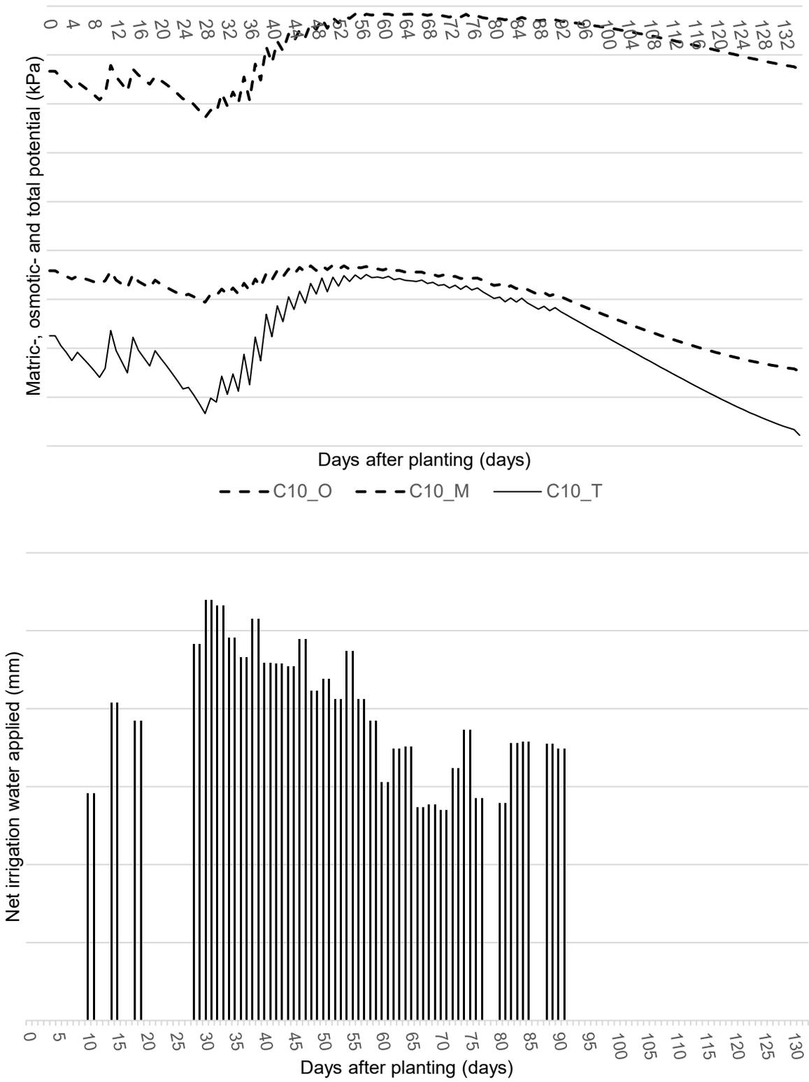
**Figure 4.7: Daily matric (C10\_M), osmotic (C10\_O) and total potentials (C10\_T) (kPa) and the net irrigation water applied (mm) (management zone 10, Orange-Riet)**
