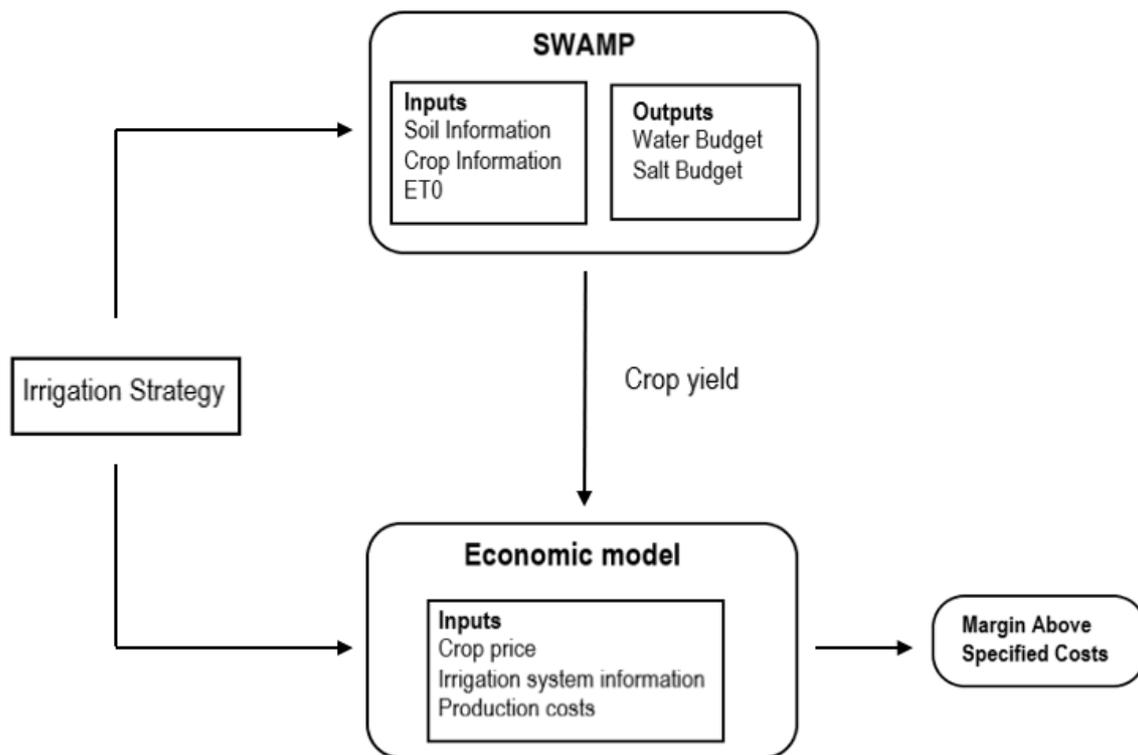
**Figure 3.2: Flow chart of the bioeconomic model simulation procedure**
