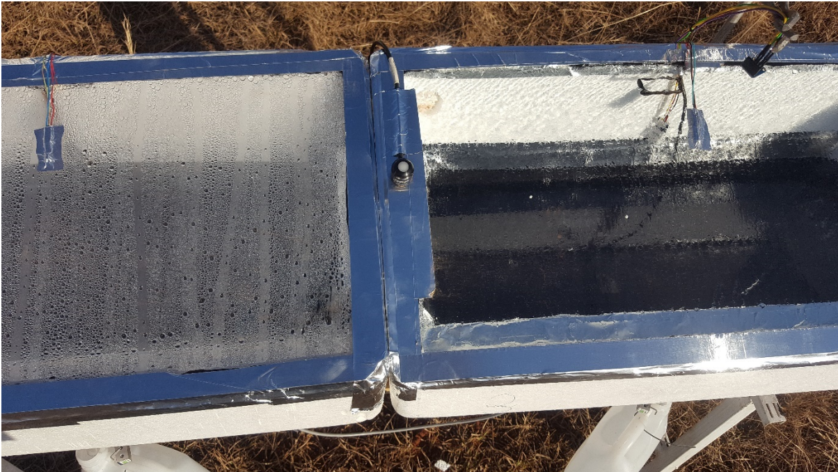
Figure 4-6: Different modes of condensation observed on PMMA and glass covers.
