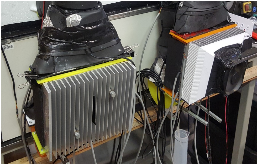
Figure 3-2: Heat sinks used as external condensers. The unit on the right is equipped with a fan for forced convection.
