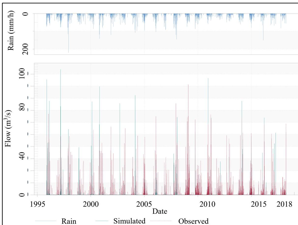
Figure 8.1 Simulated flow at A2H054 for the period from 1995 to 2018 using the uncalibrated SWMM and the modified Green-Ampt infiltration model
