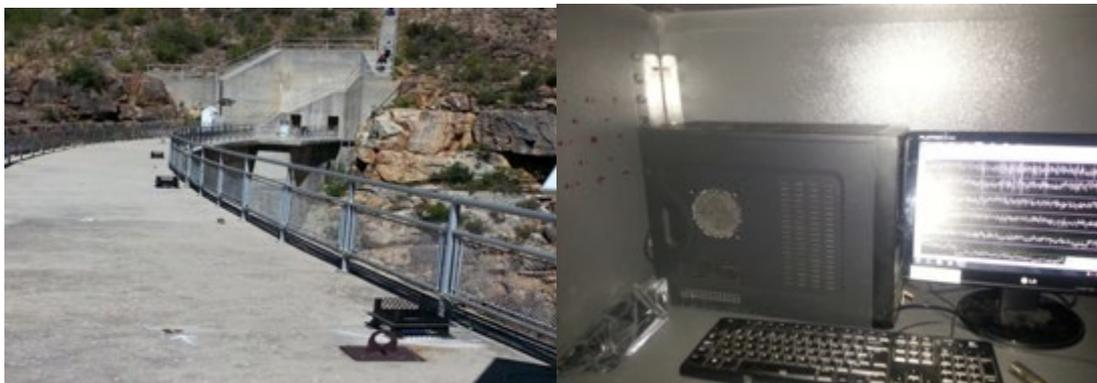
Figure 4.7: Accelerometers on the dam crest and data acquisition system in the upper dam gallery
