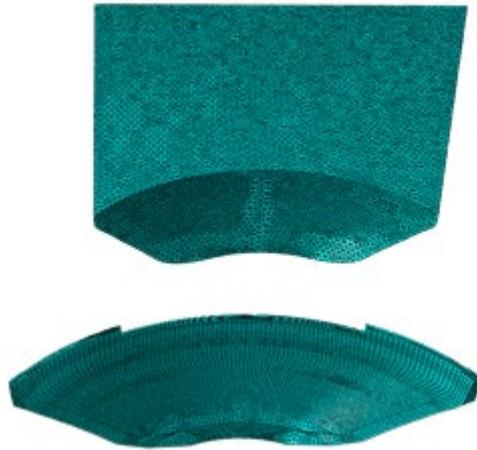
Figure 5.7: Kouga Dam Finite element model geometry
