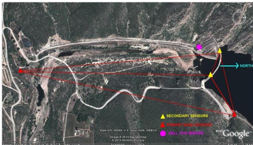
Figure 4.21: Kouga Dam GNSS/GPS Network (Pretorius et al., 2013)
