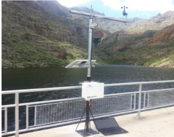
*Figure 4.5: Weather station installed on the dam crest near the spillway*
