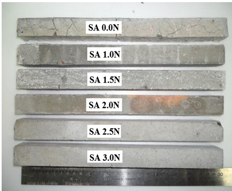
Figure 1: Concrete mixtures made with BOFS that had been chelated with oxalic acid after four days of steam curing process (Ding et al., 2017)
