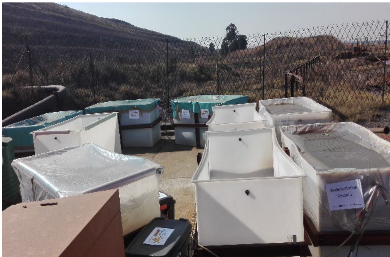
Figure 5: AMD remediation pilot plant at mine dam site (photographs taken by authors)
