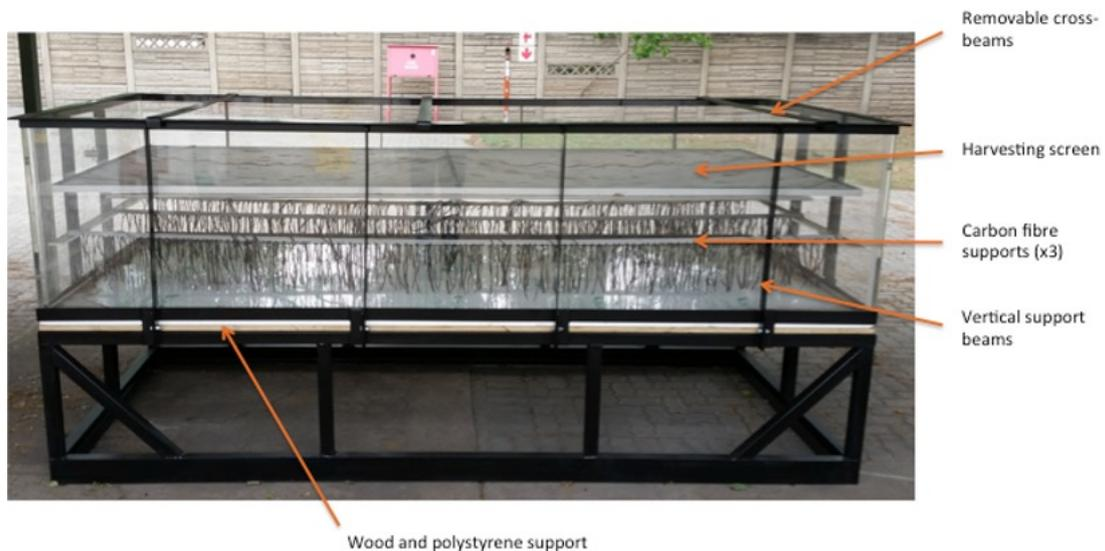
Figure 13: Photograph showing a single hybrid reactor unit and steel support frame
