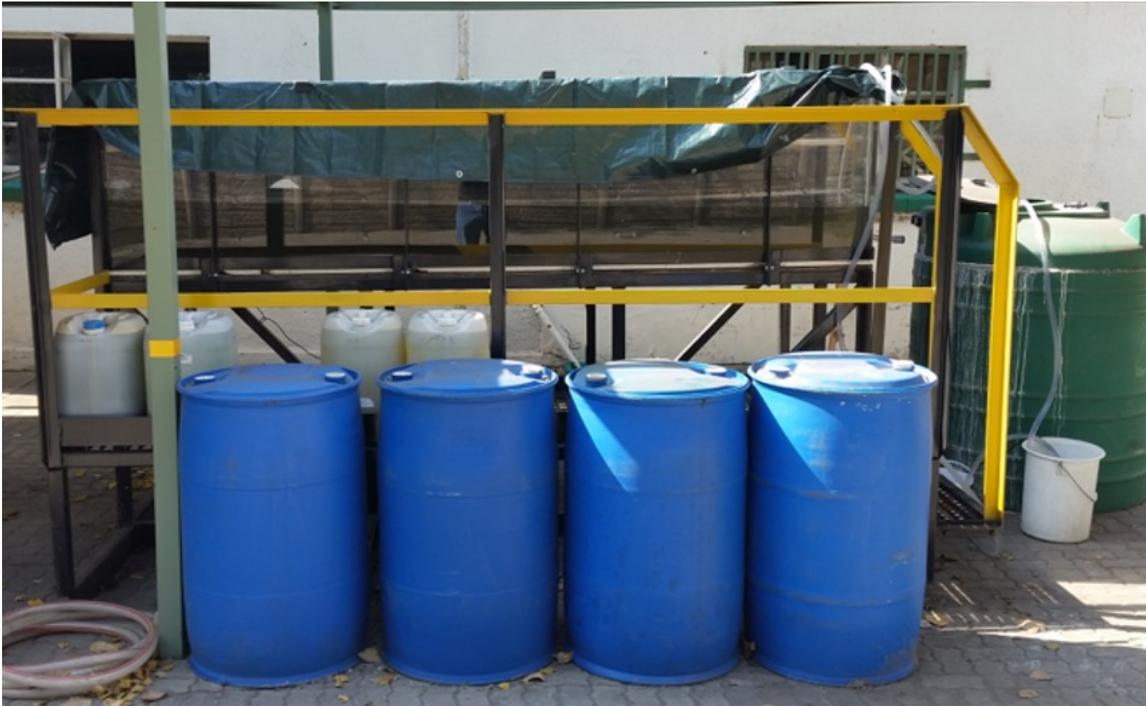
Figure 16: Image showing stages of SRB culture build-up, from 25 l drums (back) to 210 l drums (front) and ultimately 1 000 l tank (green tank)
