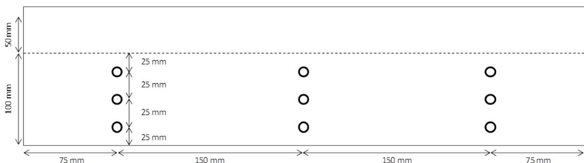
Figure 7: Schematic diagram of the new LFCR showing positions of the sample ports in the front wall.
