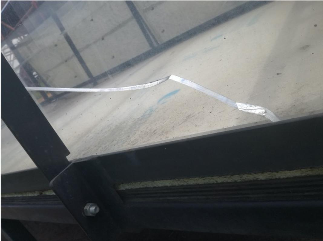
Figure 27: Photograph showing damage to the channel reactor inflicted during relocation
