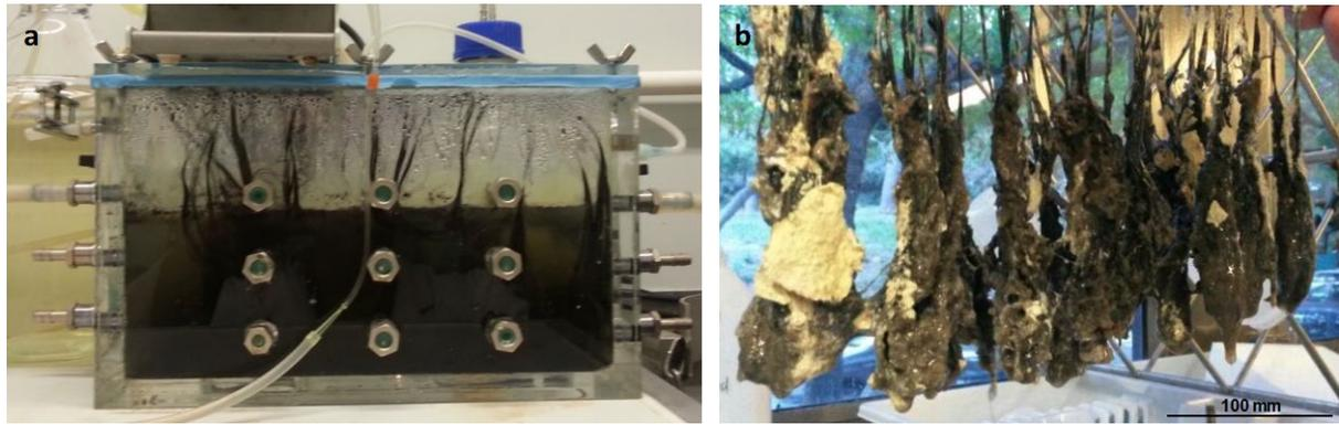
Figure 2: Images showing the application of the LFCR for sulphate reduction: (a) reactor configuration and (b) biomass accumulation on the carbon fibres
