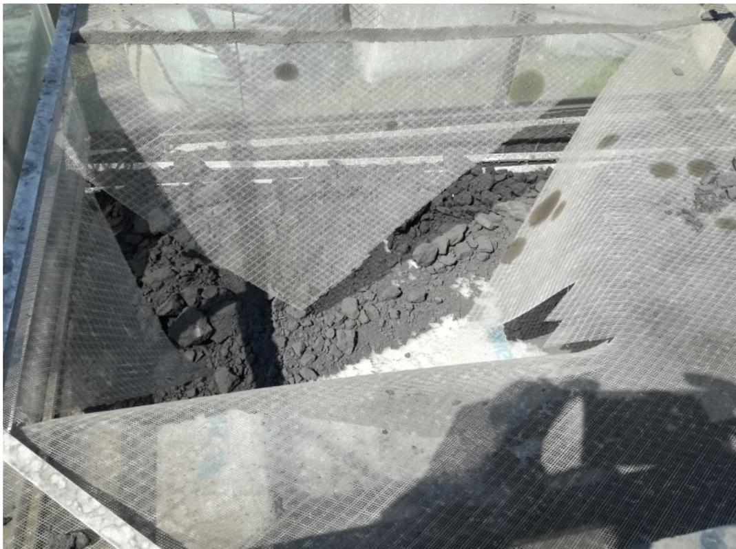
Figure 26: Photograph showing damage to the harvesting screen and accumulation of coal fines in the channel reactor
