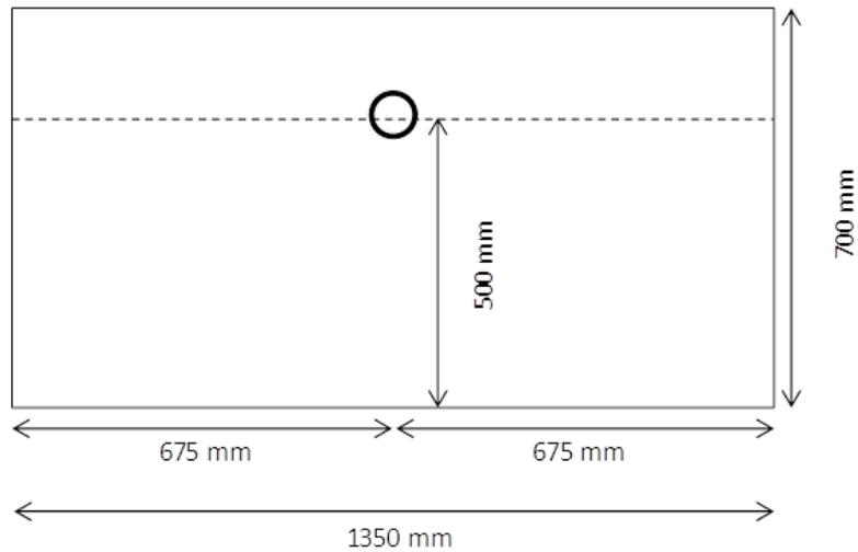
Figure 12: Schematic representation of the left and right walls of the reactor showing the location of the feed/effluent port
