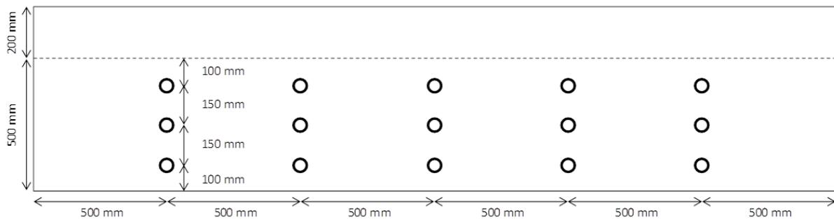
Figure 11: Schematic representation of the front wall of the pilot scale reactor showing the location of sample ports
