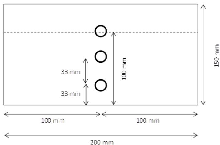
Figure 8: Schematic representation of the left and right side walls of the new LFCR showing location of feed/effluent port as well as the positioning of the carbon fibre support rod and heat exchange pipe.
