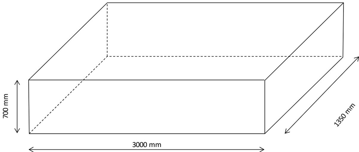
Figure 10: Overall dimensions of the channel reactor. Measurements reflect internal values
