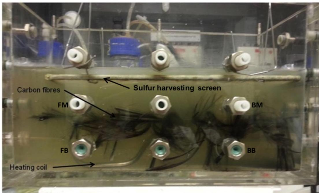
Figure 6: Photograph of the hybrid linear flow channel reactor showing the position of the heating coil, carbon fibres, sulphur harvesting screen and the location of the sampling ports (FM, FB, BM, and BB)
