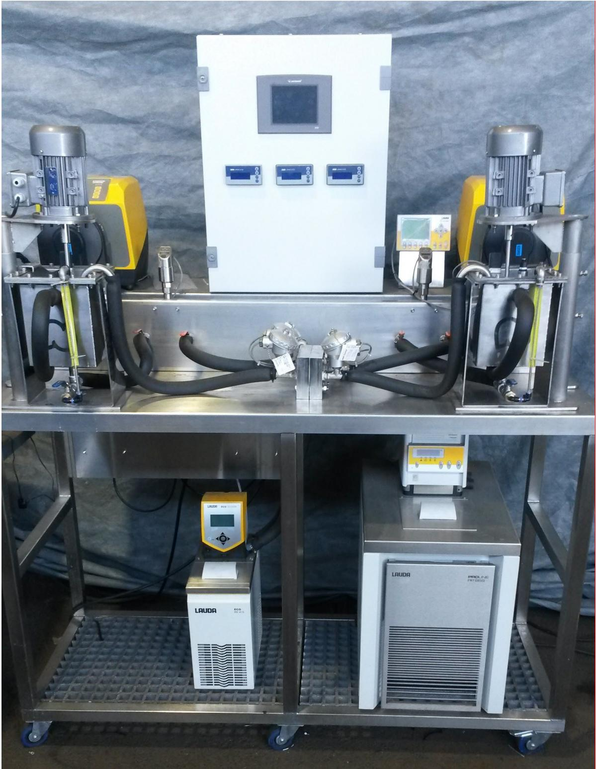
Figure 6: Photograph of commissioned DCMD experimental set up
