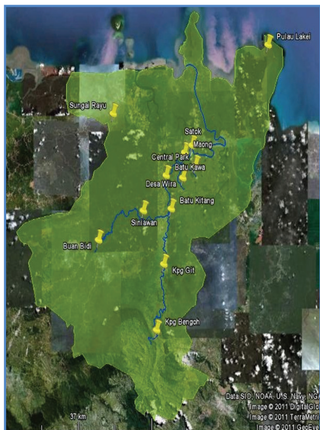
Figure 4 Delineate the Sarawak River Basin boundary, its main rivers and mark the location of water level stations in Google Earth
